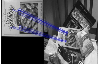
Figure 3.5: Example of matching of ORB features from the OpenCV Tutorials
