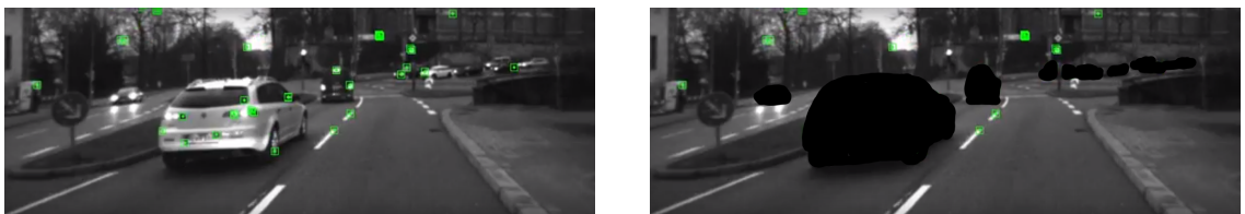
Figure 9.2: Mock-up of the image segmentation ROI: cars are excluded. This remove 'noise' in the map
