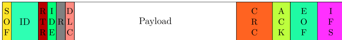
Figure 2.3: Standard (11-bit Identifier) CAN frame
