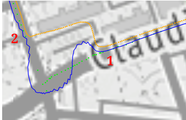
Figure 3.10: Example of the GPS causing the localization to fail: at point 1, the GPS (green) tries to track the straight path, while the Xsens (orange) correctly follows the right turn. The EKF filter output (blue) initially follows the odometry data, detecting the right turn, but eventually the system becomes unstable due to the wrong GPS estimate, causing oscillations. A correct state is only recovered around point 2
