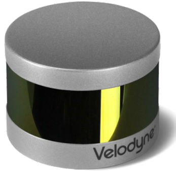
Figure 2.17: Velodyne VLP-16. A cost-effective rotating lidar for various robotic applications.
