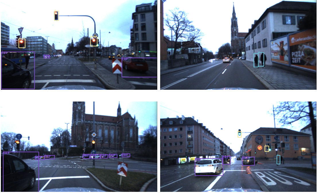
Figure 4.3: YOLOv2 applied on our images. Generally, the detector is able to find car, people and traffic lights in the sequence of images, but fails to detect all objects in a single frame.
