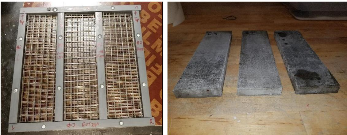
**Figure 10.12:** Mold and steel mesh reinforcement used for both specimens FERRO-FL and FERRO-S (left); FERRO-FL samples after curing (right)
