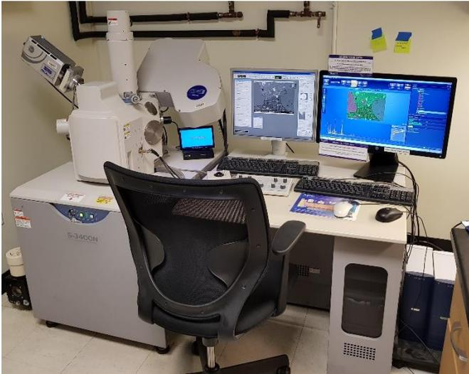
**Figure 10.18:** Hitachi S-3400N-II SEM
