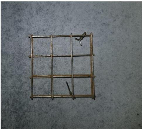
**Figure 10.10:** Reinforcement for samples FERRO-CARB
