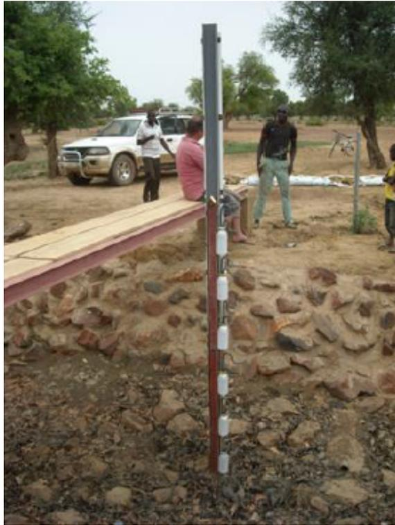
Figure 2.4: Cans used for the collection of water samples [17].
