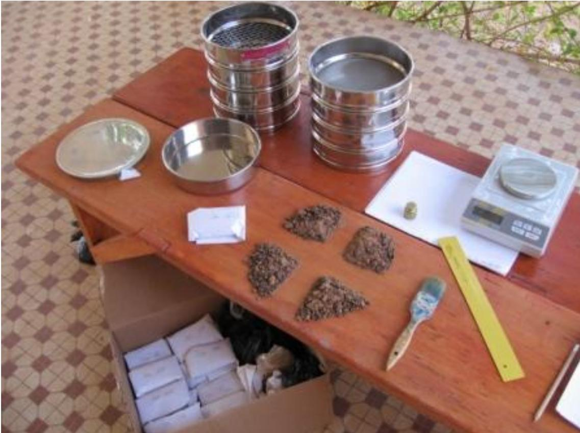
Figure 2.14: Tools adoperated for the determination of the grading curve, with the sieves and the precision scale (courtesy of Paolo Vezza).
