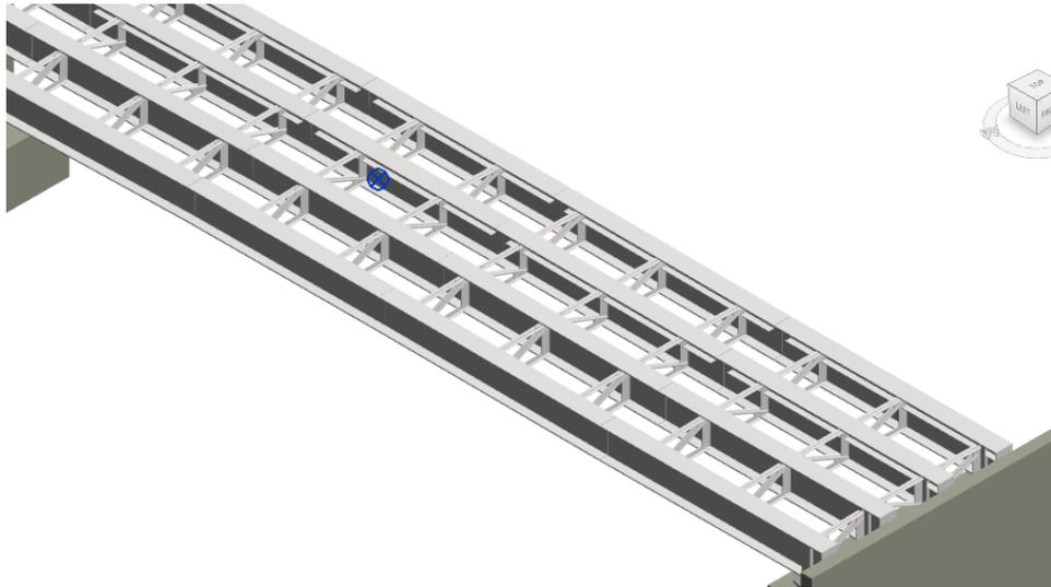
*Image 3-55 Internal trusses*
