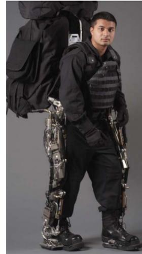
FIGURE 1.8: BLEEX Exoskeleton design [13].
