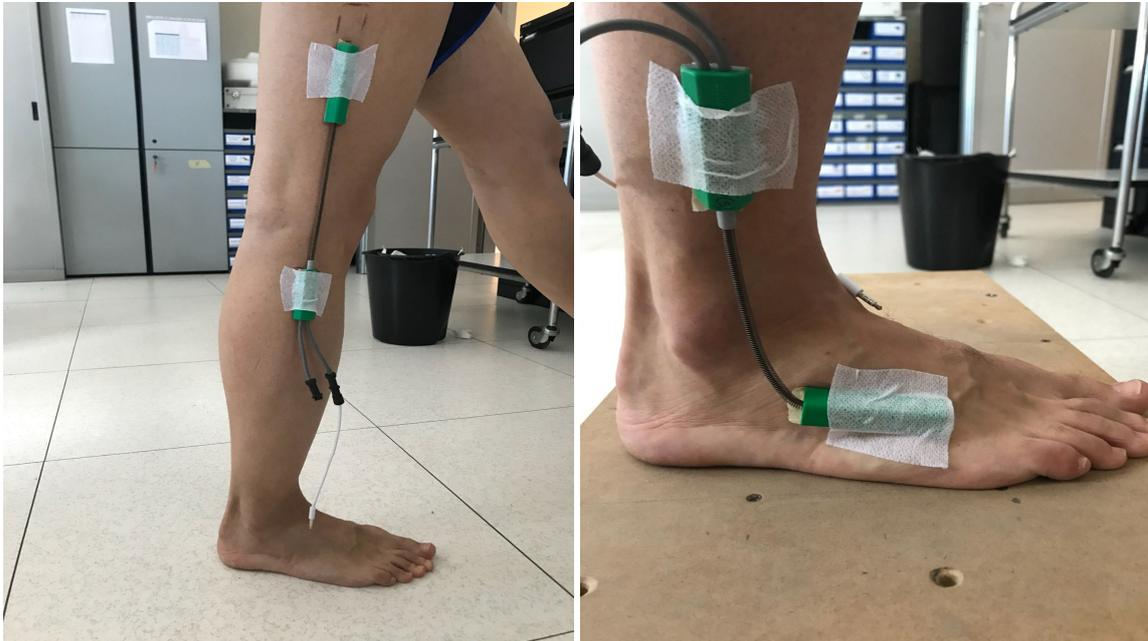
Figure 16: Left: Knee Goniometer Placement. Right: Ankle Goniometer Placement
