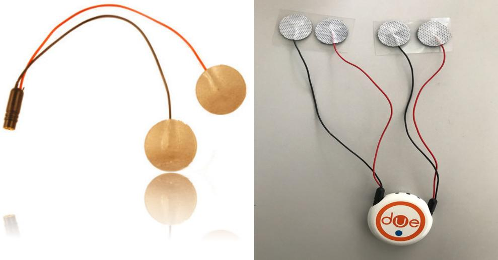
Figure 13: Left: Disposable adhesive bipolar electrode. Right: Due probe connected with 2 bipolar electrodes, one for each channel.
