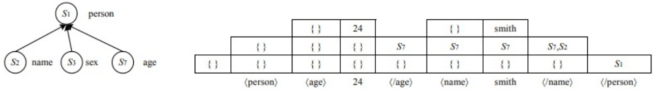
Figure 9. The tree automaton and the running stack of it on XML data stream
