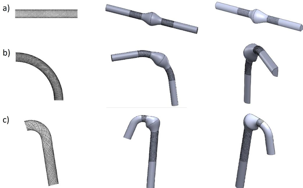
**Figure 2.2:** Stent models and final model made of aortic model and stent, in the last column they are illustrated as sections: a) model 1S b) model 2S c) model 3S
