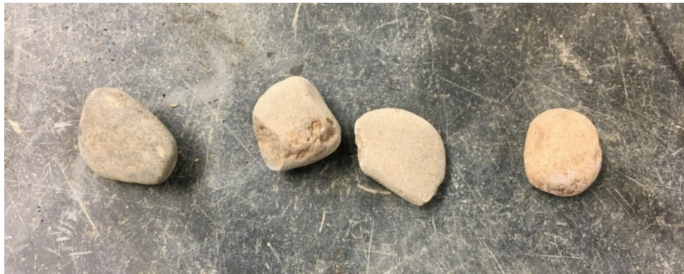
Figure 3: Aggregates after ignition test
