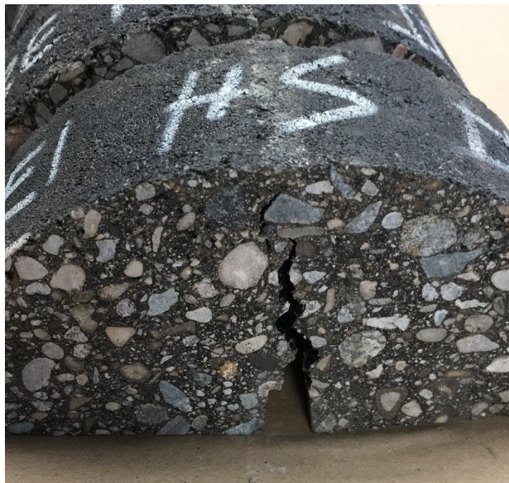
Figure 36: Tested SCB sample
