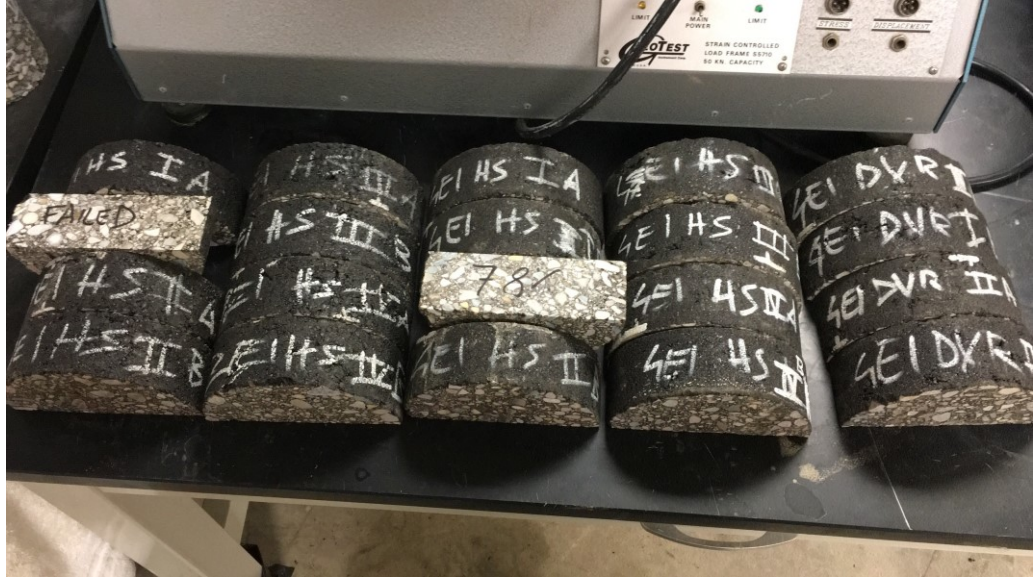
Figure 29: SCB samples ready for testing
