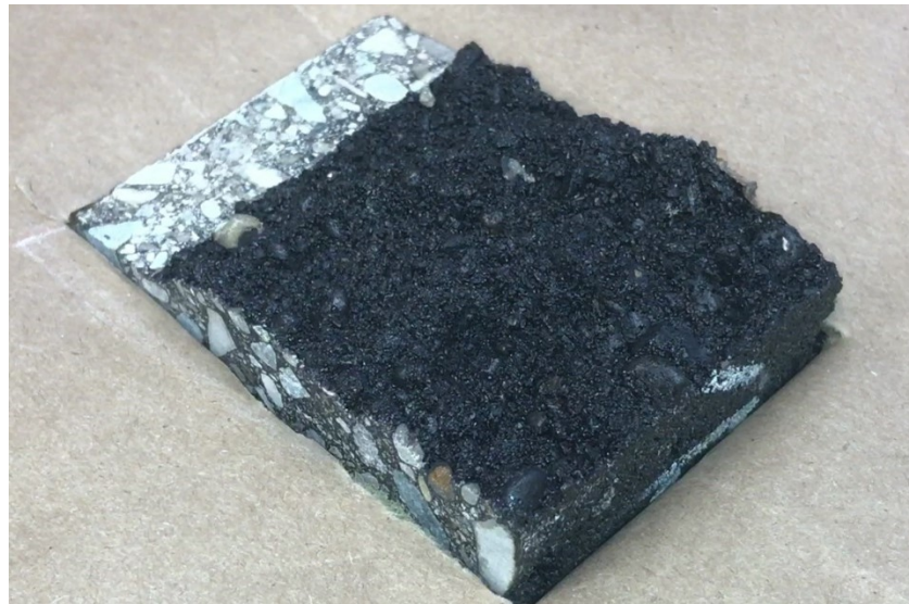
Figure 37: Sample ready for Actual Ligament Area determination
