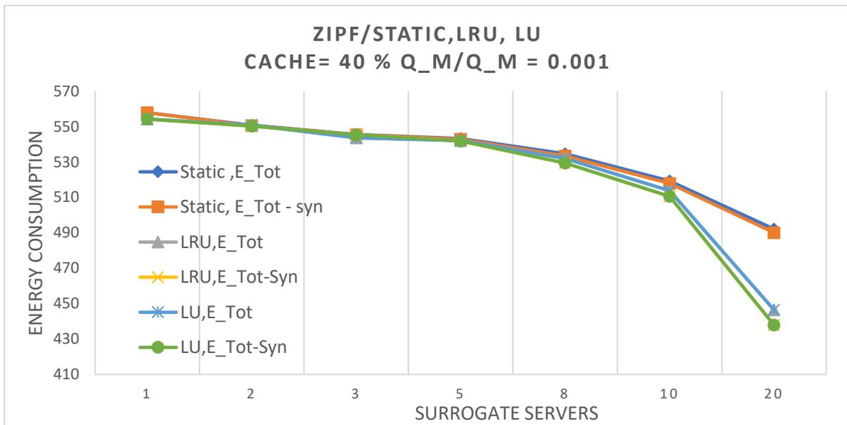
Figure 21: Total Energy Consumption with and without Synchronization, Static, LRU, LU Caching, Zipf and Uniform Content Request Distribution. When  $Q_m/q_m = 0.001$
