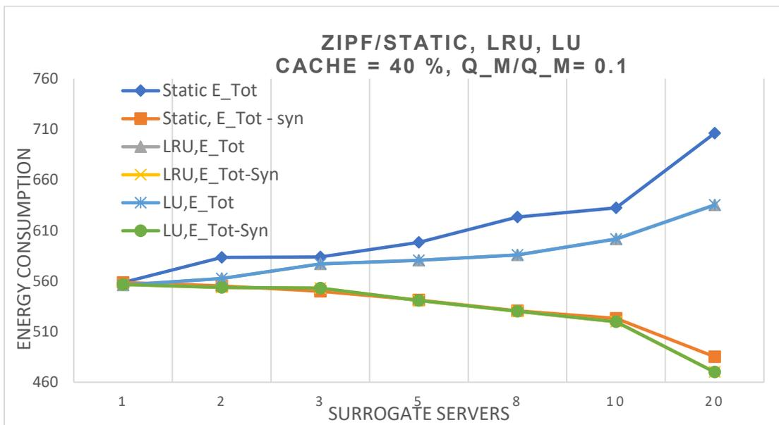
Figure 23: Total Energy Consumption with and without Synchronization, Static, LRU, LU Caching, Zipf and Uniform Content Request Distribution. When  $Q_m/q_m = 0.1$
