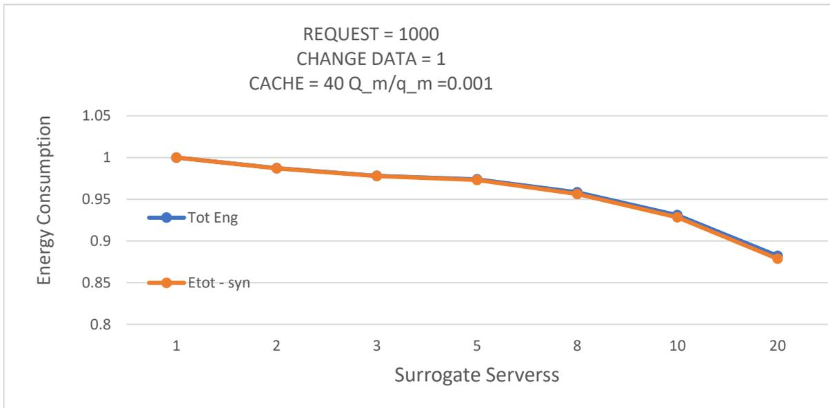
Figure 18: Total Energy Consumption with and without Synchronization, Static Caching, Uniform Content Request Distribution. When  $Q_m/q_m = 0.001$
