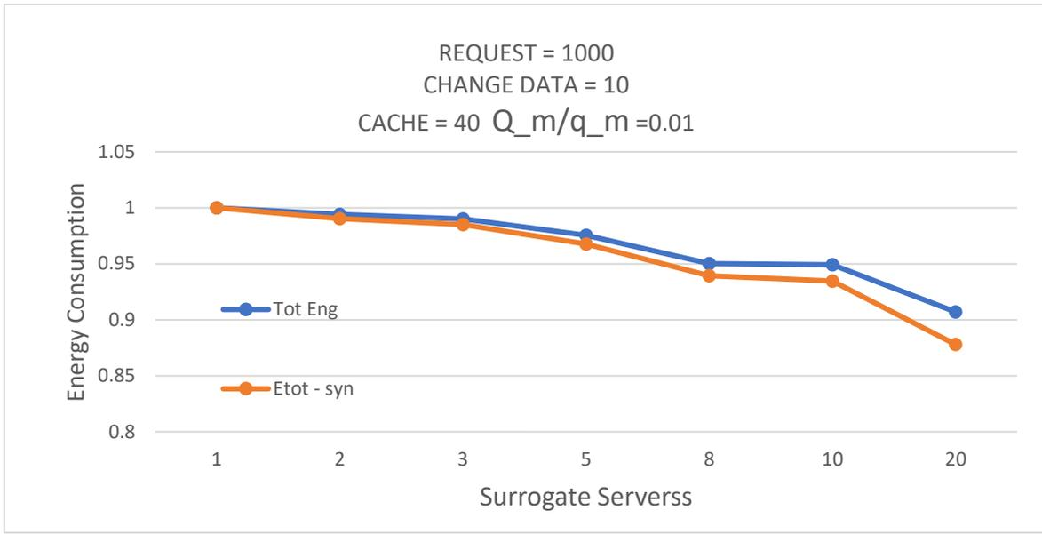
Figure 19: Total Energy Consumption with and without Synchronization, Static Caching, Uniform Content Request Distribution. When  $Q_m/q_m = 0.01$
