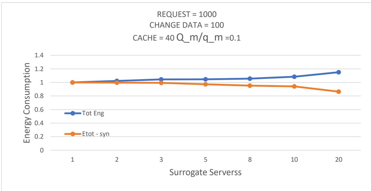
Figure 20: Total Energy Consumption with and without Synchronization, Static Caching, Uniform Content Request Distribution. When  $Q_m/q_m = 0.1$
