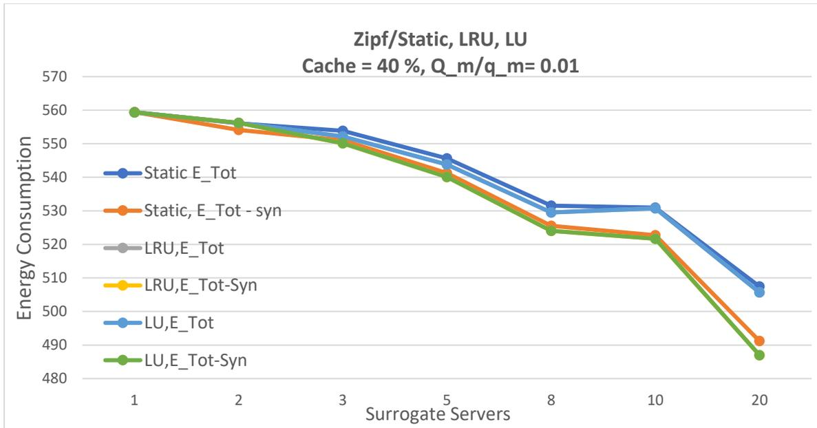
Figure 22: Total Energy Consumption with and without Synchronization, Static, LRU, LU Caching, Zipf and Uniform Content Request Distribution. When  $Q_m/q_m = 0.01$
