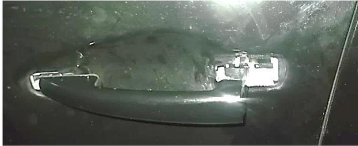
Figure 7 Damages to door lock
