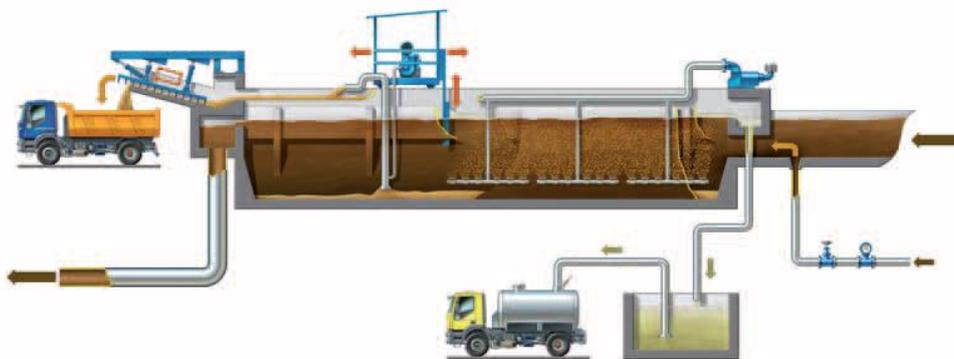
Figure 2 Sand & Oil Removal
