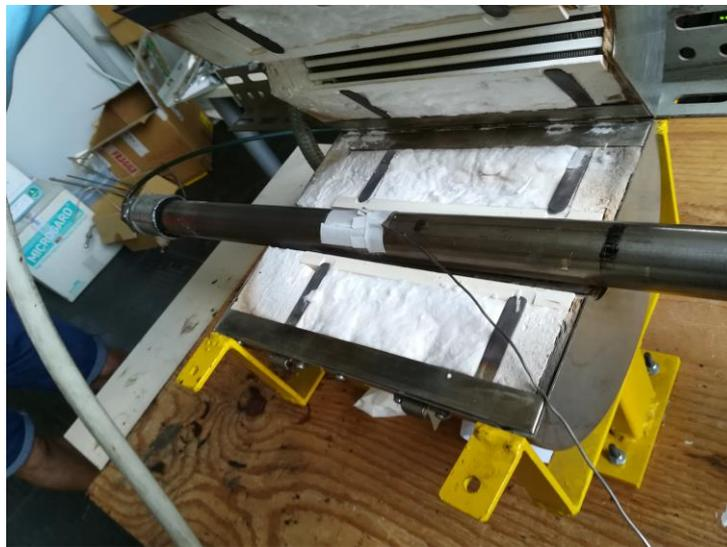
Figure 30 Positioning of the activation reactor inside the horizontal insulated electrical oven . Wadding was used as filter in the extremities of the reactor to avoid dragging of powder .
