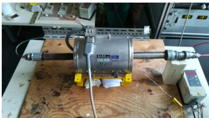
Figure 31 Activation Unit. The thermocouple controls Temperature transients and of activation Temperature for the designed dwelling time.
