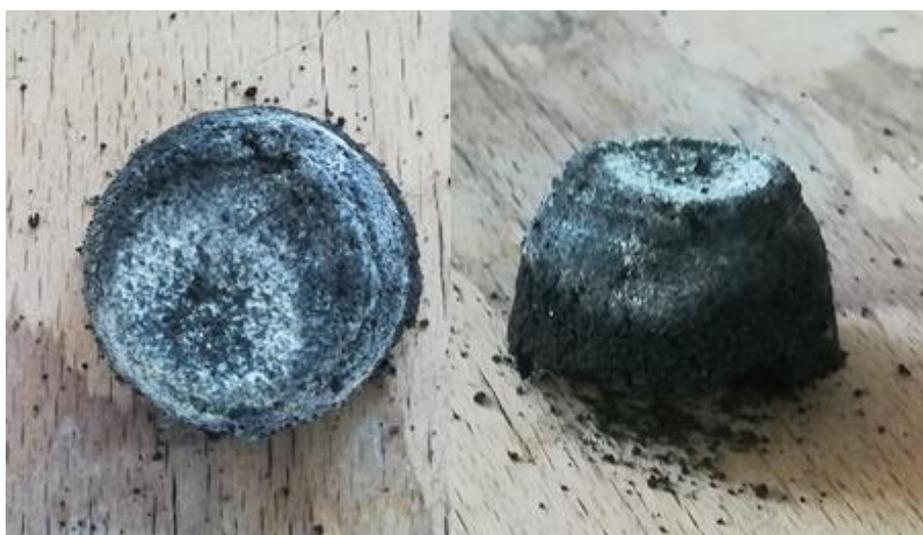
Figure 34 Mould formation for humidified exhaust samples.
