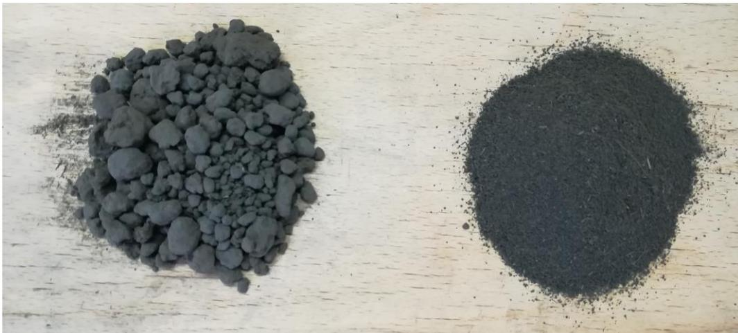
Figure 1 As received Sewage Sludge (S0) complements after sieving.
