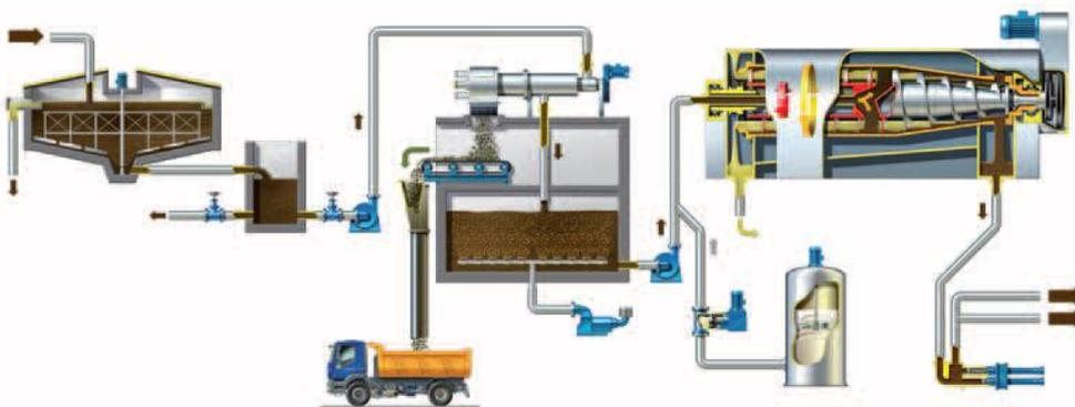
Figure 10 Centrifugal Dehydration
