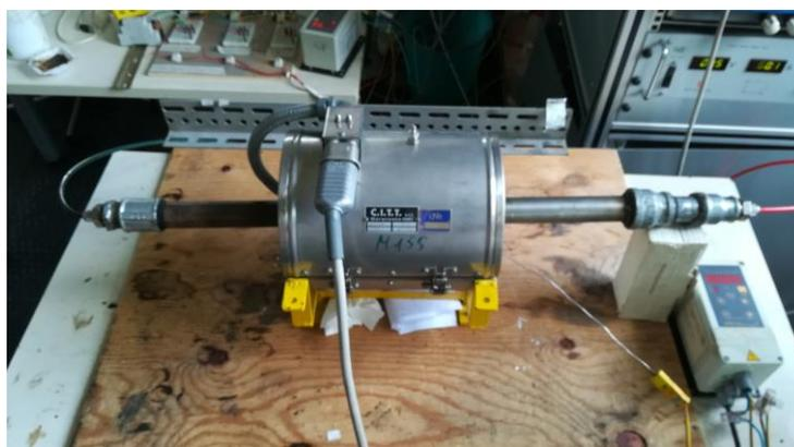
Figure 31 Activation Unit. The thermocouple controls Temperature transients and of activation Temperature for the designed dwelling time.
