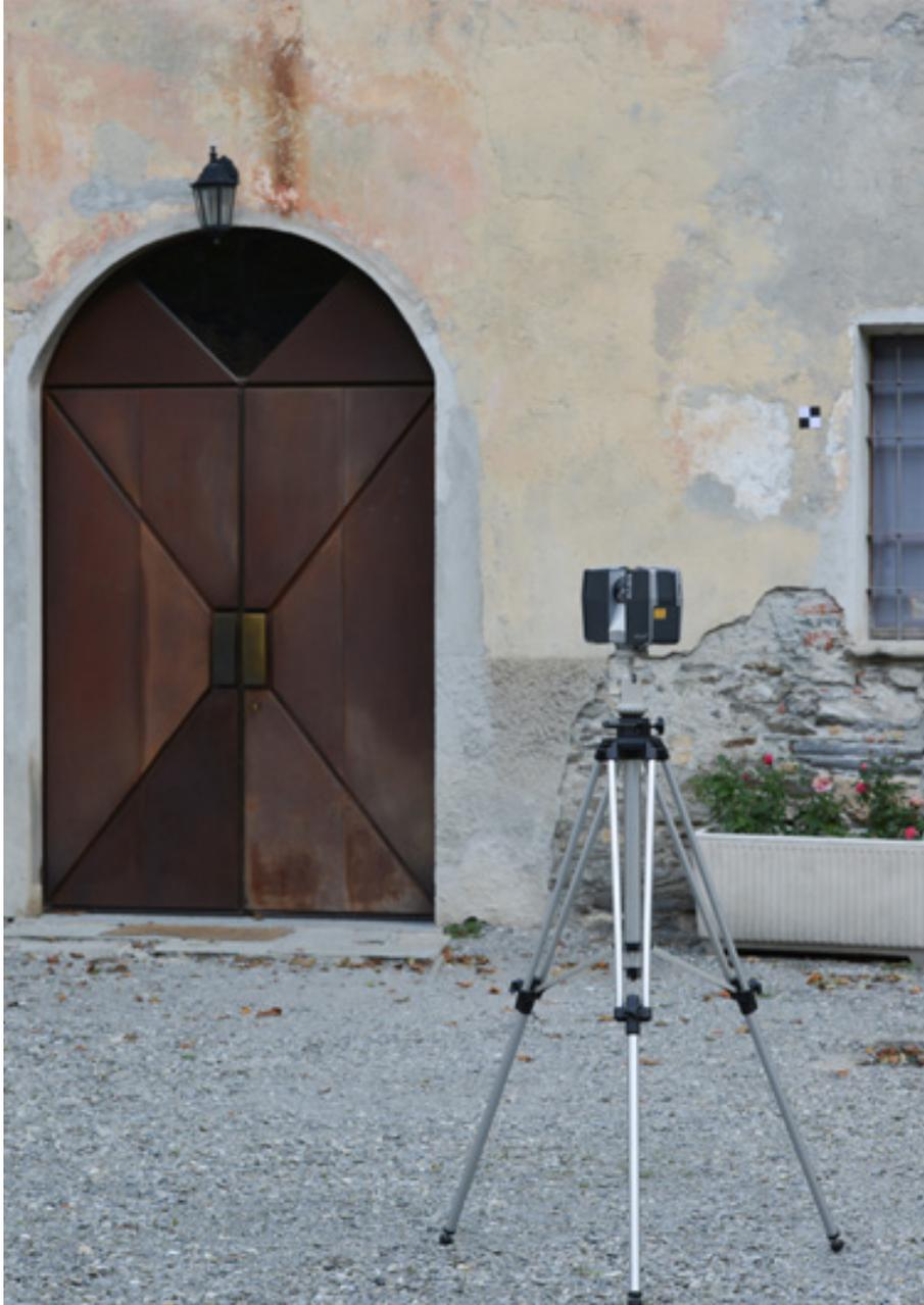
Laser scanner terrestre FARO Focus 3D 120 S.
