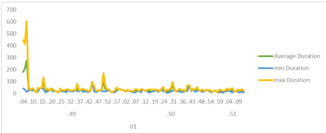
**FIGURE 19 AVERAGE (GREEN), MINIMUM(BLUE) AND MAXIMUM(ORANGE) AWS LAMBDA INVOCATIONS' DURATION WITH NODE.JS FOR 300 LOG-IN**
