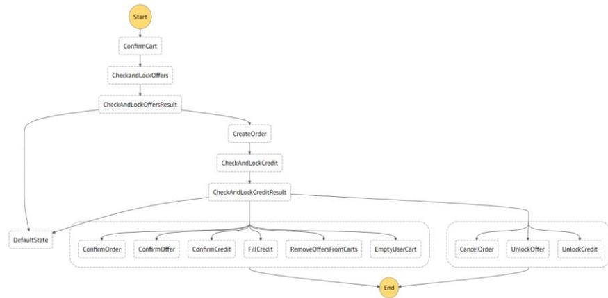
**FIGURE 6 AWS CONSOLE SHOWING A GRAPHICAL VIEW OF AN AWS STEP FUNCTIONS WRITTEN IN ASL REPRESENTING UBS'S PURCHASE FLOW**
