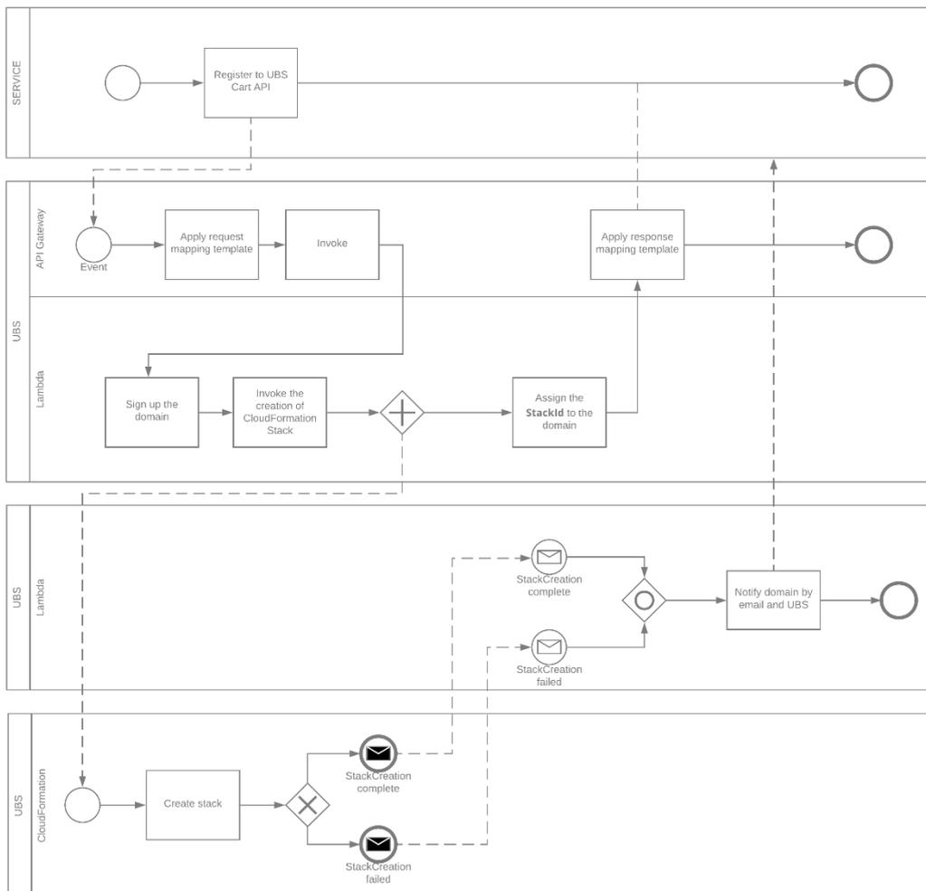
**FIGURE 12 BPMN REPRESENTING THE PROCESS OF THE AUTOMATIC CREATION OF A DOMAIN'S CART API BY REGISTERING TO UBS AND USING CLOUDFORMATION TEMPLATE**
