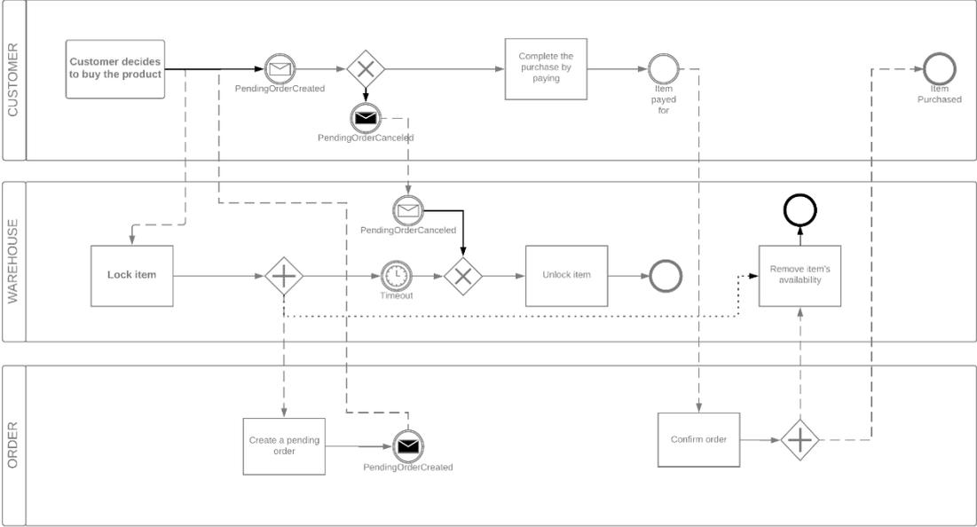
**FIGURE 5 BPMN REPRESENTING THE PURCHASE FLOW IN A SYSTEM HAVING NO CART**
