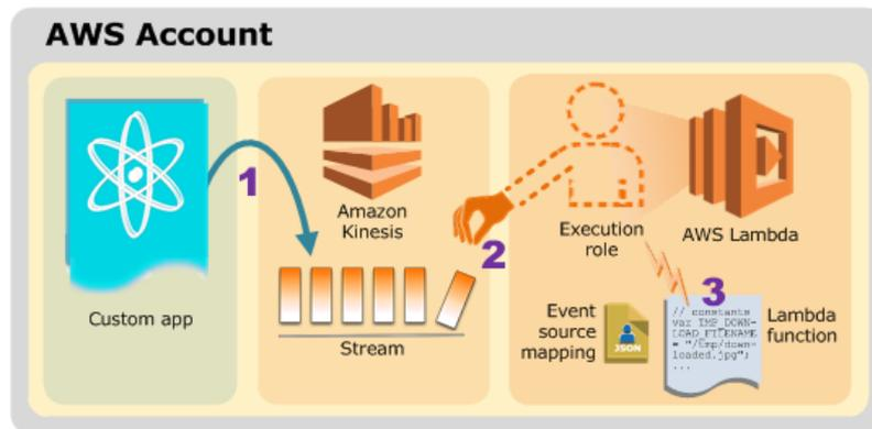
an event source mapping residing in the Lambda service must be configured so that, at a fixed time rate, the service polls the stream to check whether some data has been published; then, the events
