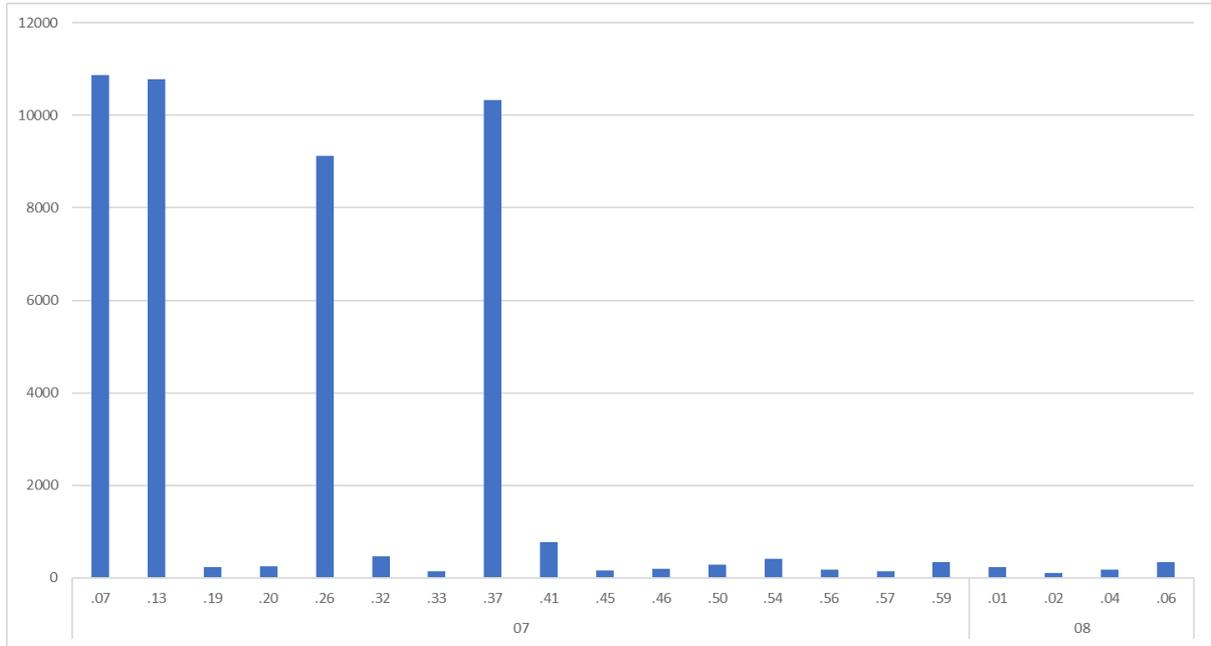
**FIGURE 22 MAXIMUM AWS LAMBDA INVOCATIONS' DURATION WITH JAVA FOR 900 LOG-IN REQUESTS DIVIDED IN 15 GROUPS VARYING THE PARALLEL REQUESTS COUNT AND THE WAIT TIME BETWEEN REQUESTS**
