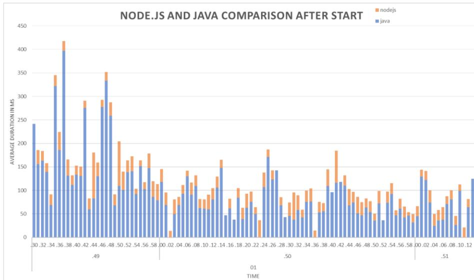
**FIGURE 20 AVERAGE AWS LAMBDA INVOCATIONS' DURATION WITH JAVA (BLUE) AND NODE.JS (ORANGE) WITHOUT COLD START**
