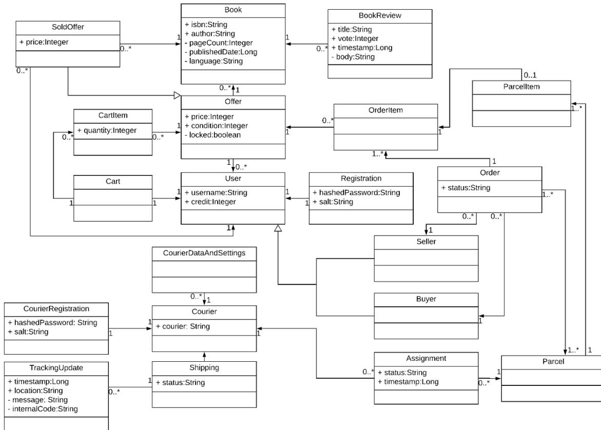
FIGURE 4 UML CLASS DIAGRAM REPRESENTING THE OVERALL CLASSES NEEDED FOR THE PURCHASE PROCESS
