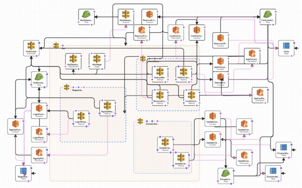
**FIGURE 11 AWS CONSOLE SHOWING A GRAPHICAL VIEW OF THE CLOUDFORMATION TEMPLATE DESCRIBING AND PROVISIONING ALL THE AWS COMPONENTS NEEDED TO DEPLOY THE ARCHITECTURE PROVIDING A SUBSCRIBED DOMAIN'S CART APIS**
