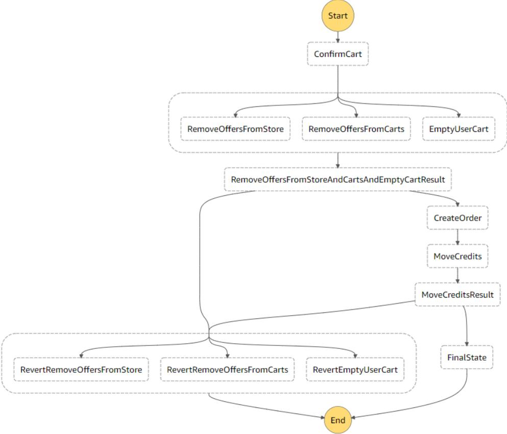
**FIGURE 7 AWS CONSOLE SHOWING A GRAPHICAL VIEW OF AN AWS STEP FUNCTIONS WRITTEN IN ASL REPRESENTING AN HYPOTHETICAL UBS'S PURCHASE FLOW FULLY COMPLIANT TO COMPENSATING TRANSACTION PATTERN**
