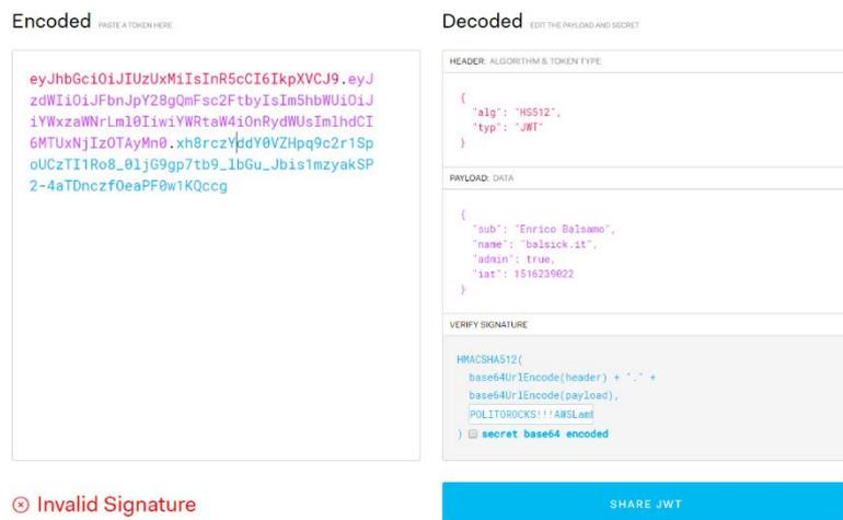
FIGURE 2 JWT.IO VERIFYING AND DECODING AN INVALID JWT TOKEN
