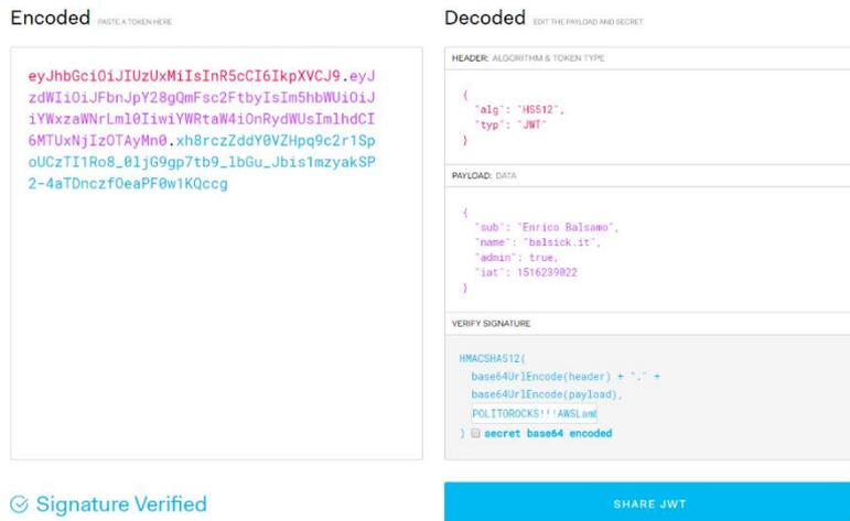
FIGURE 3 JWT.IO VERIFYING AND DECODING A VALID JWT TOKEN
