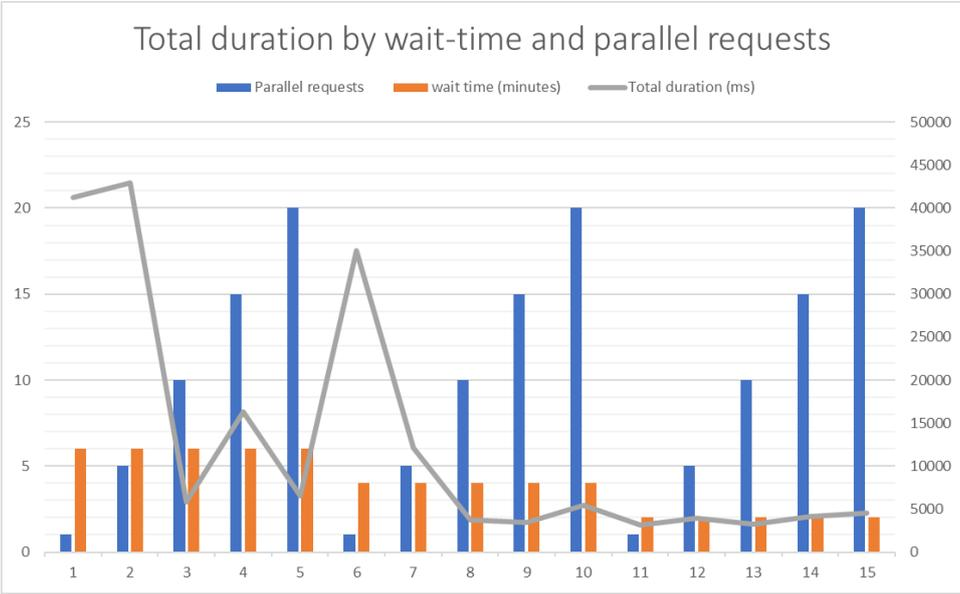
**FIGURE 21 TOTAL AWS LAMBDA INVOCATIONS' DURATION WITH JAVA FOR 900 LOG-IN REQUESTS DIVIDED IN 15 GROUPS VARYING THE PARALLEL REQUESTS COUNT AND THE WAIT TIME BETWEEN REQUESTS**
