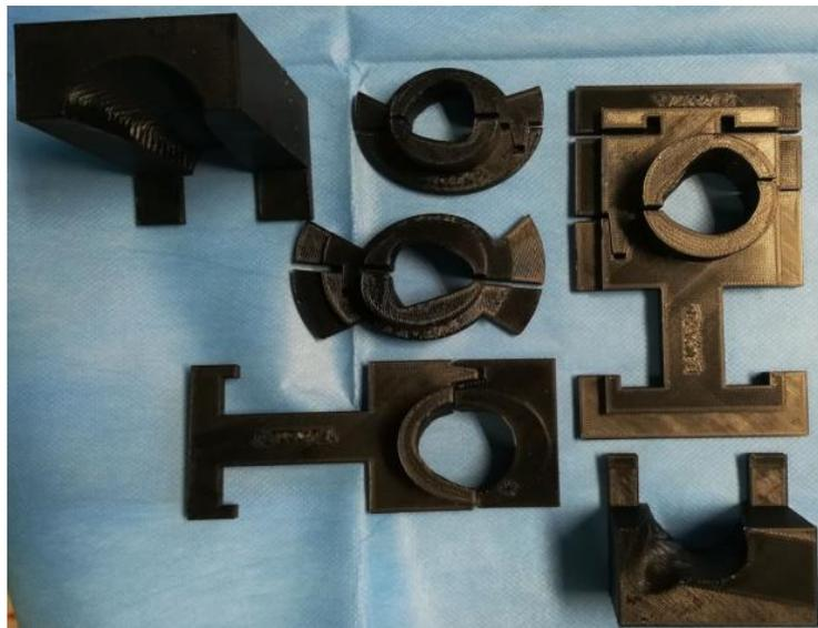
**Figure 4.9:** 3D printing of the final design of the alignment and cutting guides for femur and tibia.
