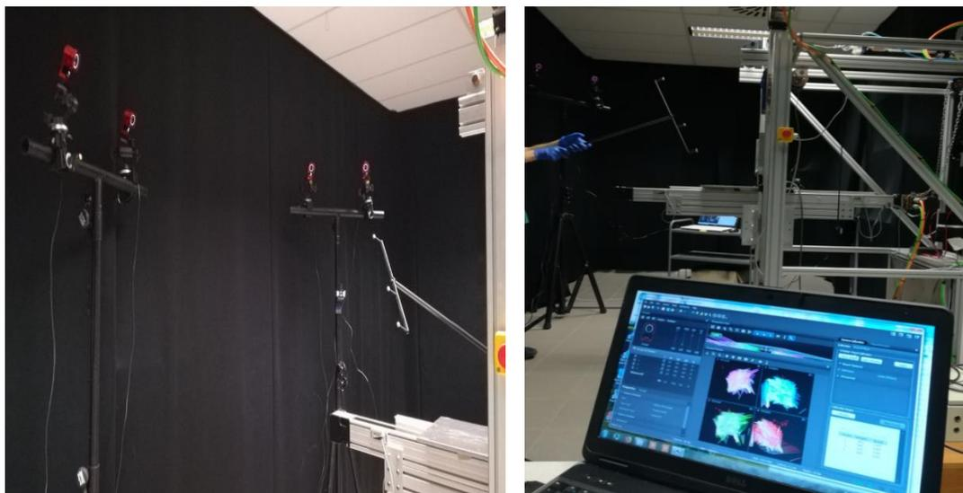
**Figure 4.15:** (left)Cameras positioning before the calibration process; (right) Calibration process.
