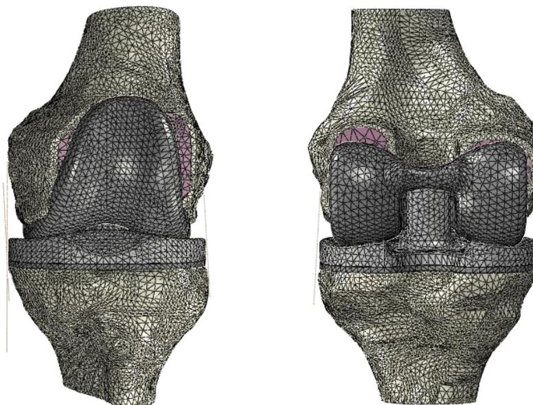
**Figure 6.5:** (left) Abaqus mesh model from front point of view; (right) Abaqus mesh model from back point of view.
