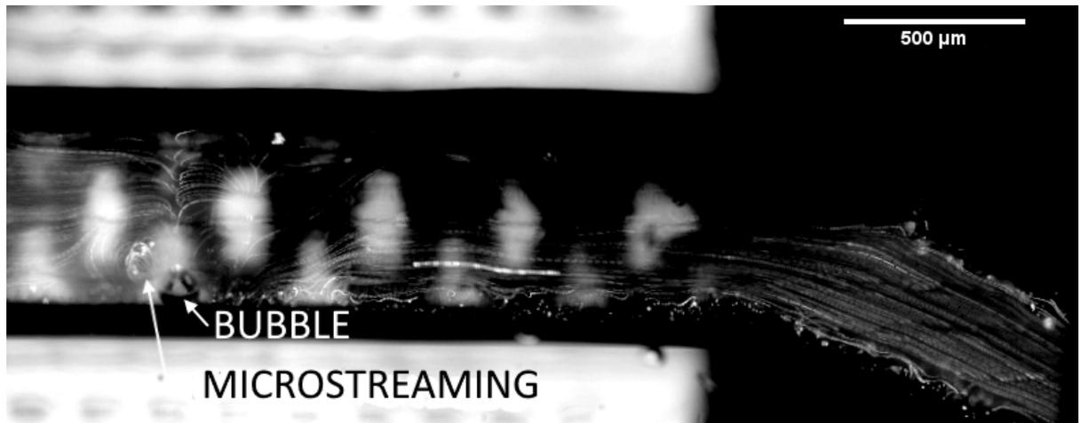
Figure 3: Microstreaming pattern as developed by an oscillating bubble. Device manufactured with clear, optically transparent resin.
