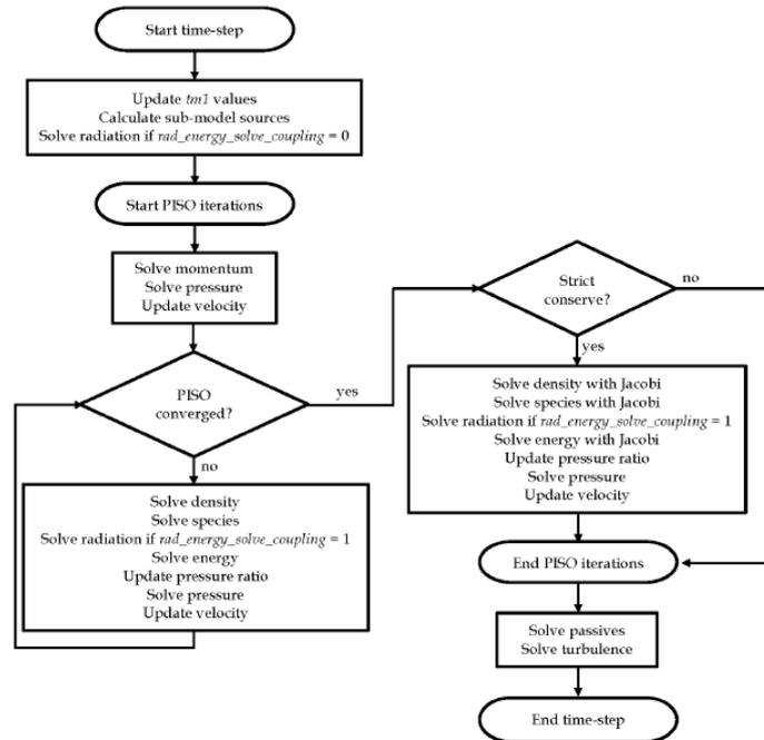
**Figure 1.6:** Solution Order of the Transport Equation. The Turbulence Equation were removed from the PISO loop for efficiency reasons.
