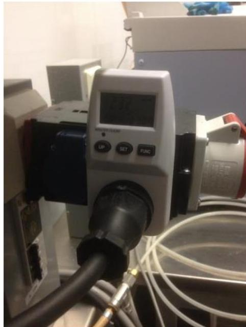
**Fig. 4.19:** Electricity meter.
