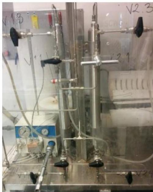
**Fig. 4.7:** Ball valves disposition.
