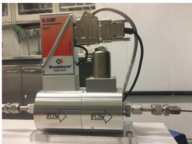
**Fig. 4.5:** Mass flow controller.
