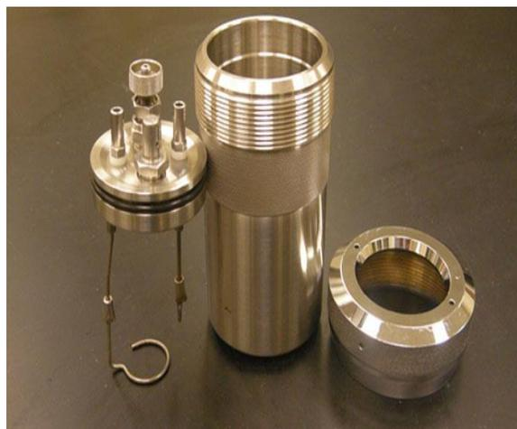
**Fig. 5.13:** Section of bomb calorimeter (left) and main components of bomb calorimeter (right).
