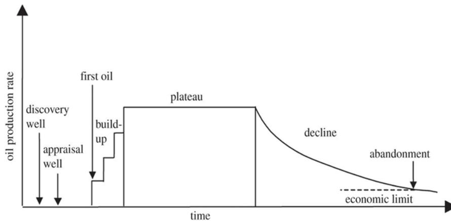
Figure 2.2 Representation of theoretical production rates during life cycle of an oil and gas (Höök, Söderbergh, & Jakobsson, 2009) field
