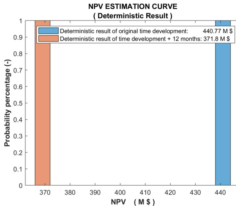
Figure 5.18 Visual representation of the Deterministic NPV results related to an offshore field (FPSO rented) with respect to two different project development durations
