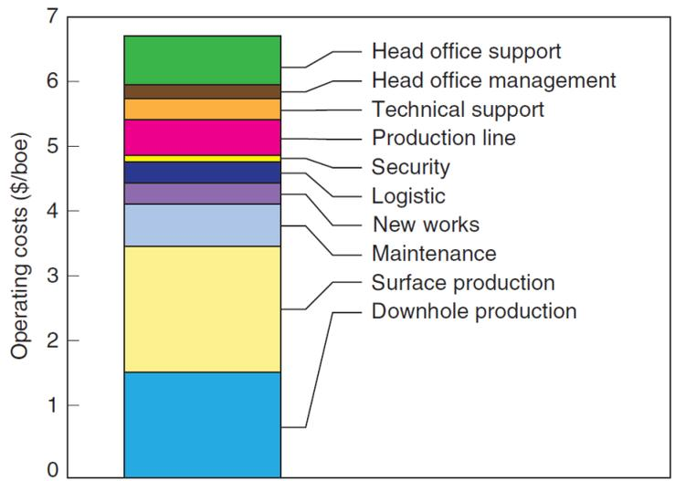
Figure 3.23 Example of elements and their cost inside the Operational cost category (Bret-Rouzaut, Favennec, & al., 2011)
