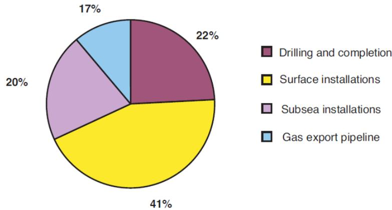
*Figure 3.22 Example of the cost breakdown for an offshore development (North Sea, water depth 300 m) (Bret-Rouzaut, Favennec, & al., 2011).*
