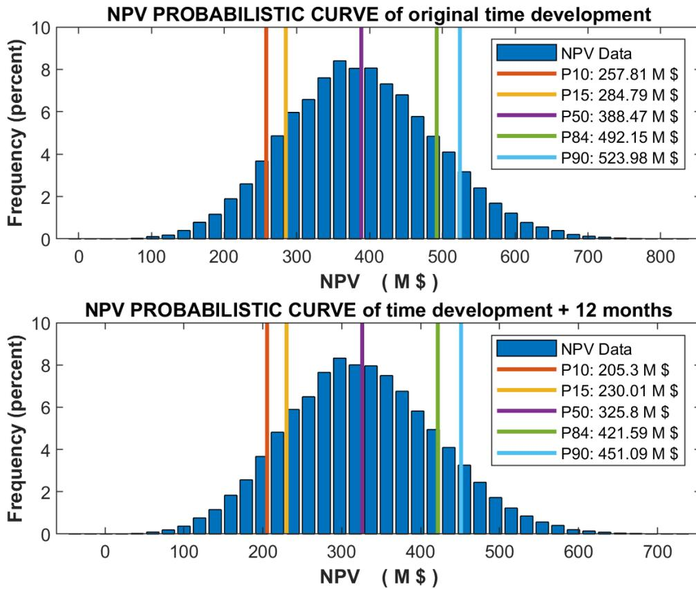
*Figure 5.10 Probabilistic results of NPV from the simulation related to an offshore field (TLP) with respect to two different project development durations*
