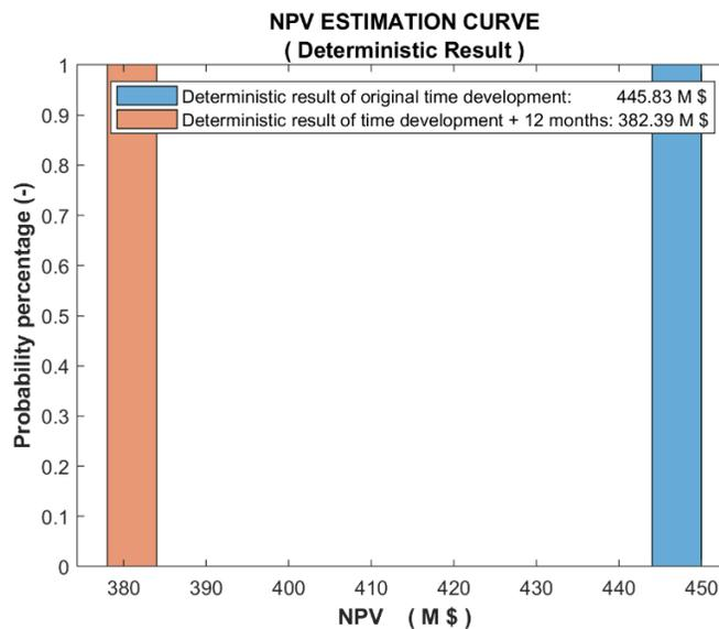
*Figure 5.8 Visual representation of the Deterministic NPV results related to an onshore field with respect to two different project development durations*
