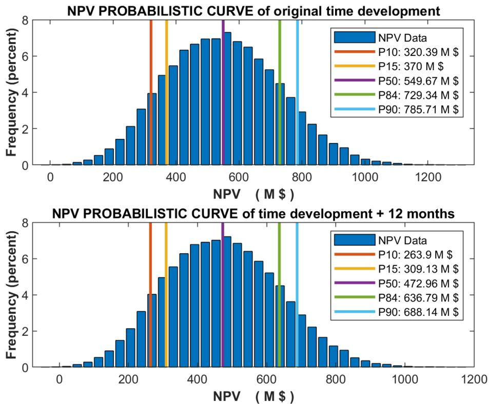
Figure 5.20 Probabilistic results of NPV from the simulation related to an offshore field (FPSO rented) with respect to two different project development durations
