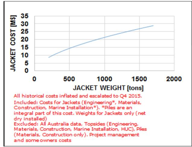
Figure 3.13 Example of Jacket cost determination (in millions of dollar) from the Jacket weight (tons) (Spera, 2016)
