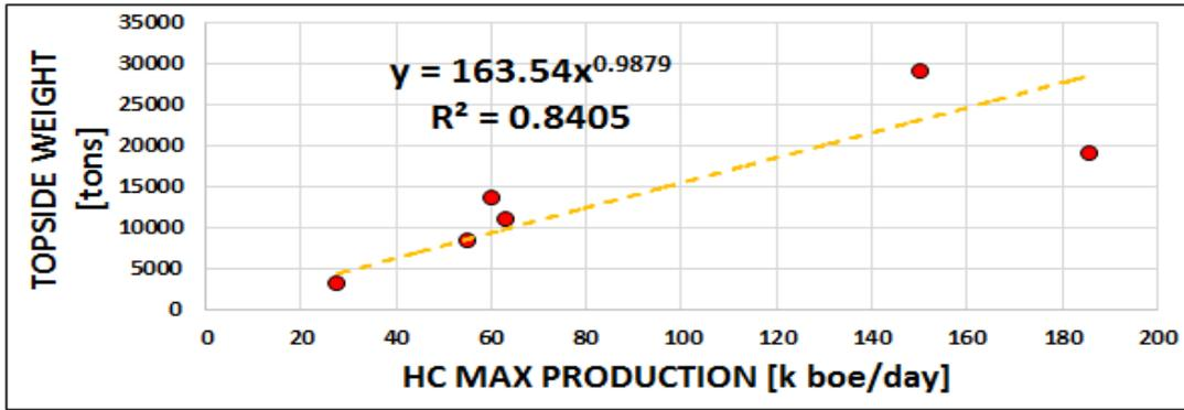
Figure 3.11. Trend of the Topside weight based on the maximum production of hydrocarbon (thousands of bbl per day) (Spera, 2016).
