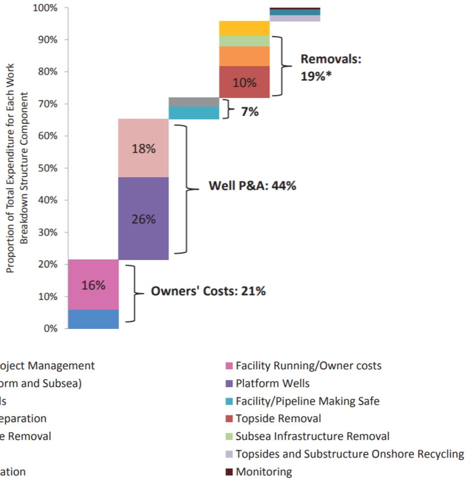
Figure 3.20 Components of WBS relative to all projects in UKCS and their impact on the total Abandonment cost (Decommissioning Insight, 2014)
