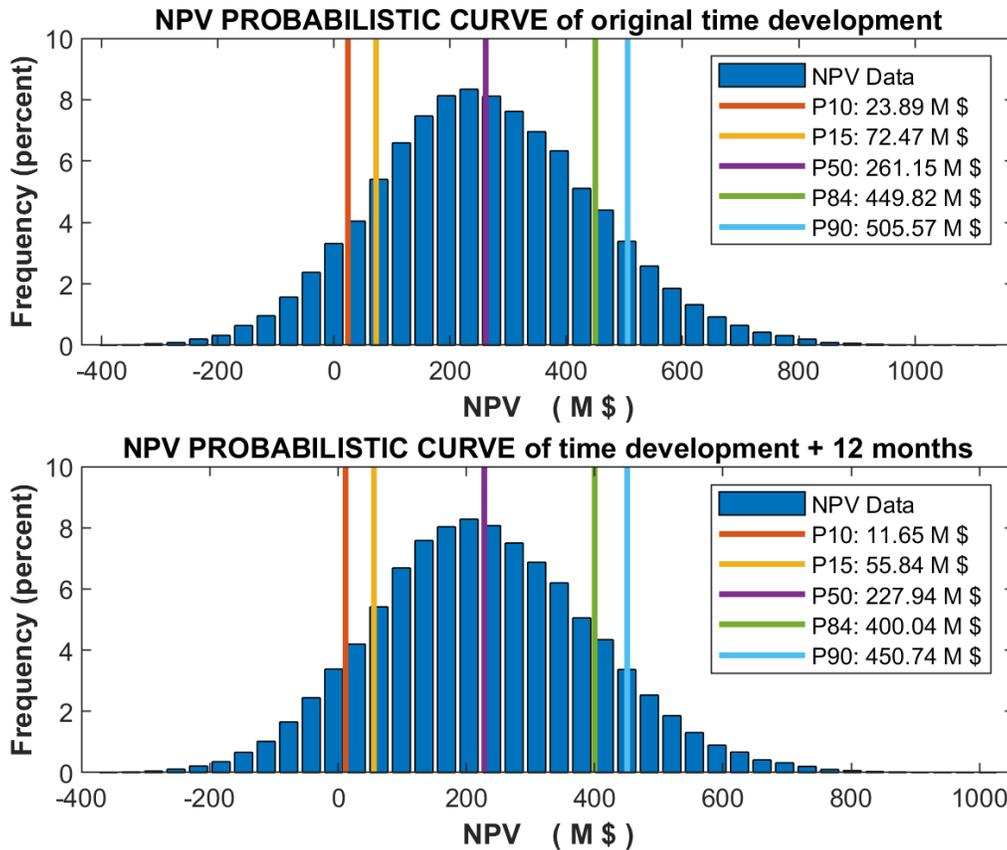
*Figure 5.5 Probabilistic results of NPV from the simulation related to an onshore field with respect to two different project development durations*
