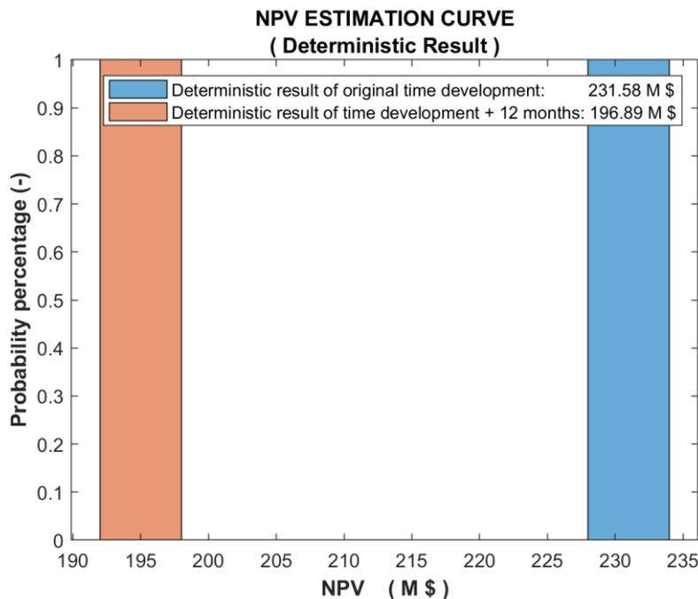
Figure 5.3 Visual representation of the Deterministic NPV results related to an onshore field with respect to two different project development durations
