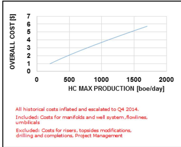
Figure 3.17 Example of Overall cost determination (in millions of dollar) with respect to the maximum production (boe/day) (Spera, 2016)
