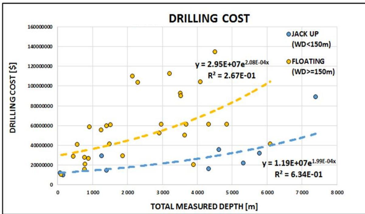
Figure 3.5 Estimation of the Drilling cost regression curve (in dollars) based on the available data of the Jack-up rig and Floating rig (Spera, 2016)
