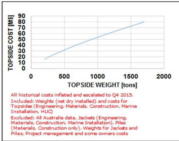
Figure 3.15 Example of Topside cost determination (in millions of dollar) from the Topside weight (tons) (Spera, 2016)
