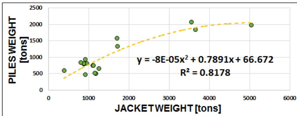
Figure 3.10 Example of the Piles weight (tons) determination of an offshore platform from the Jacket weight (tons) (Spera, 2016).
