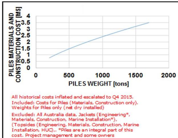
Figure 3.14 Example of Piles cost determination (in millions of dollar) from the Piles weight (tons) (Spera, 2016)
