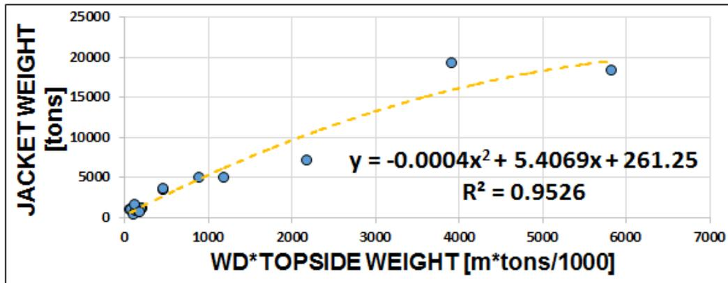
Figure 3.12 Example of the Jacket weight (tons) determination of an offshore platform from the water depth and Topside weight (meters \* tons /100) (Spera, 2016).
