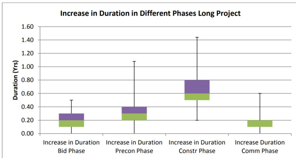
Figure 3.34 Example of the duration overrun analysis at different project stages of a Long Project (Ezenta, 2015)
