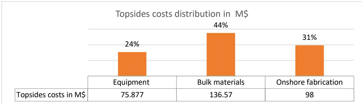
Figure 3.8. Comparison of the elements' cost (in million dollars and in percentage) relative to the total cost of the Topside category (OGDE, 2013)
