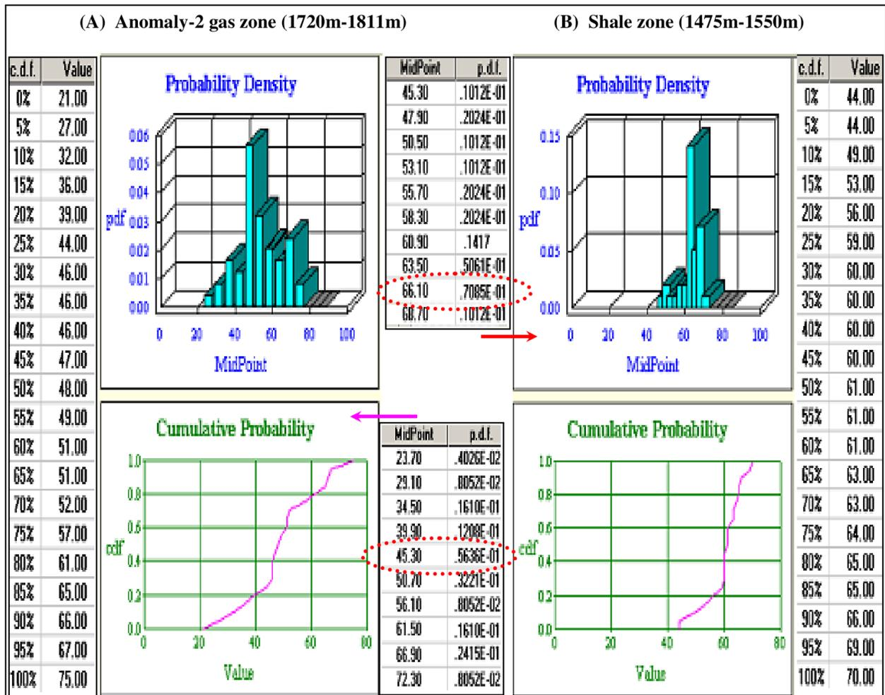
Figure 3.31 Example of distribution definition of the gamma ray data of the gas and shale zones of the well Darfell-7 (Lashin & Mousa, 2015)
