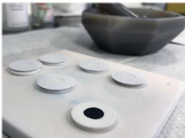
Figure 14 - Working electrode application on YSZ electrolyte disc by slurry coating
