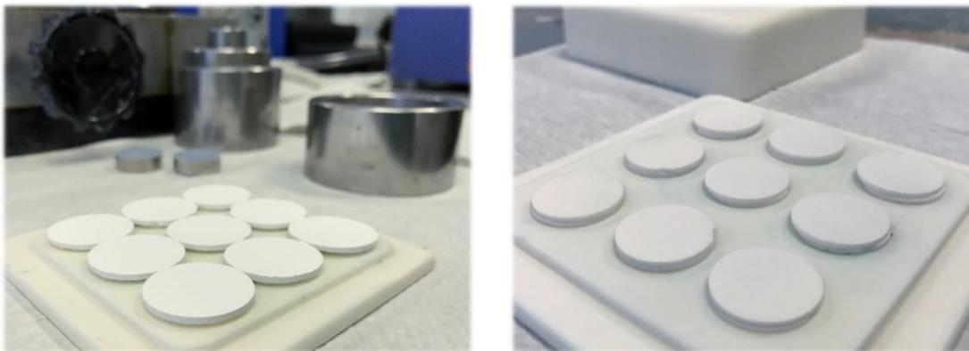
Figure 12 - YSZ electrolyte discs before (left) and after (right) sintering procedure
