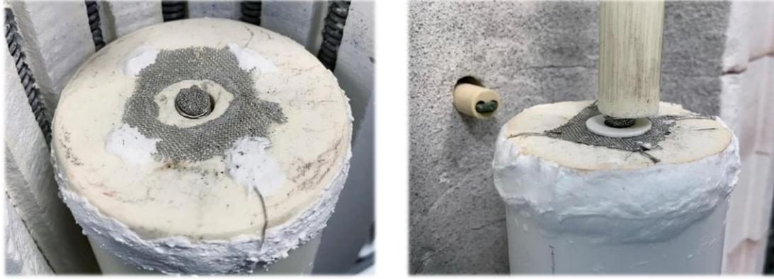
Figure 16 - Three electrodes setup
