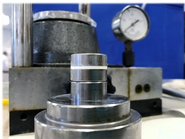
Figure 11 - YSZ electrolyte disc die pressing
