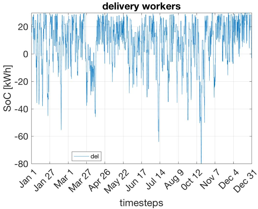
Figure 9: delivery vehicle SoC trend
