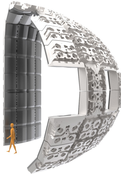
FIGURE 1.3: The ITER blanket [23].
