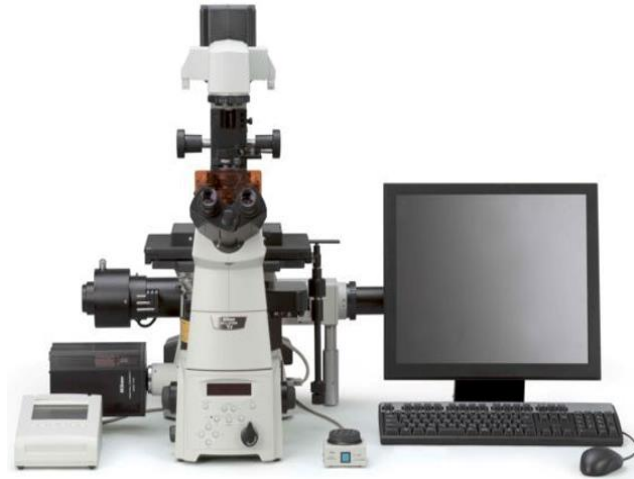
Figure 15: Far-field microscope integrated with the illumination system and a computer screen
