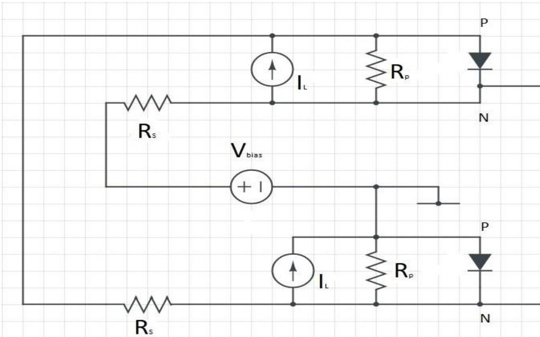
**Figure 35:** Electronic circuit of the tandem.
