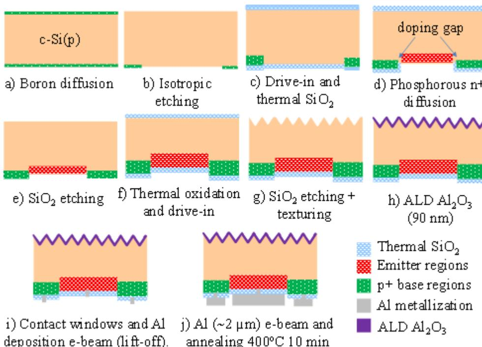
**Figure 31:** Main stages of the baseline fabrication process with homogeneous emitter [14].
