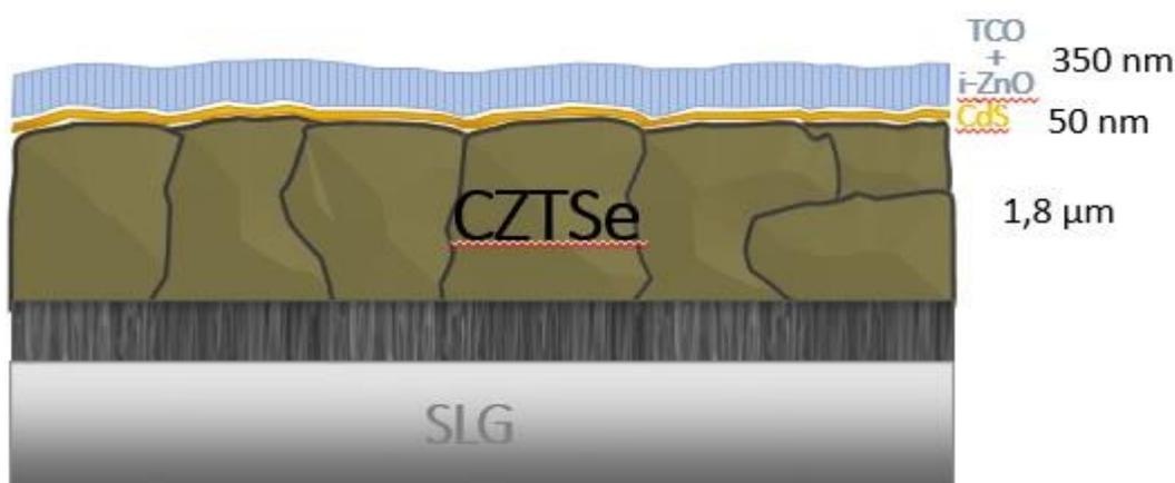
Figure 5: Kesterite based solar cell's structure [7].
