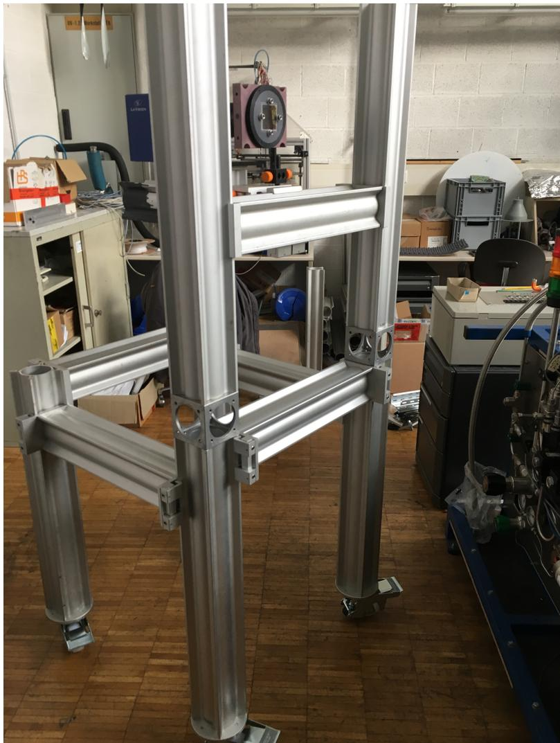
Figure C.1: Camera optical bench
