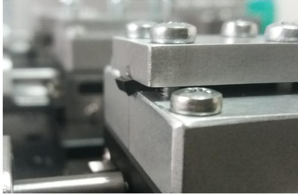
Figure 3.9. Flattening of the rubber layer.
