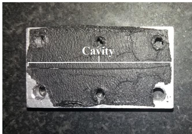
Figure 5.15. Cavity of the soft rubber.
