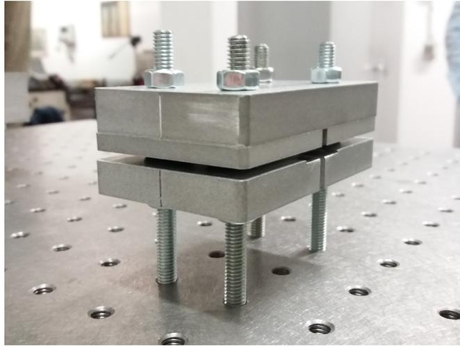
Figure 3.18. Final package locking system for thermal testing.
