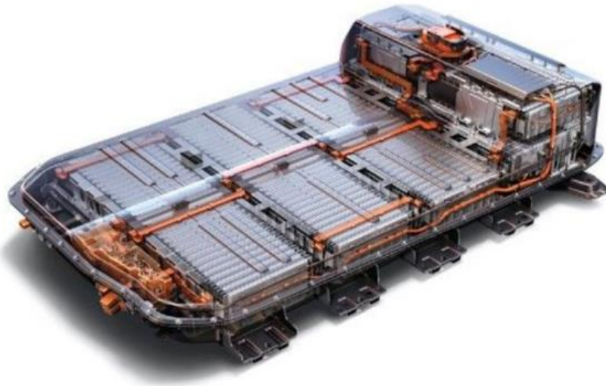
Figure 12: battery pack of 2017 Chevrolet Bolt. Source: General Motors.
