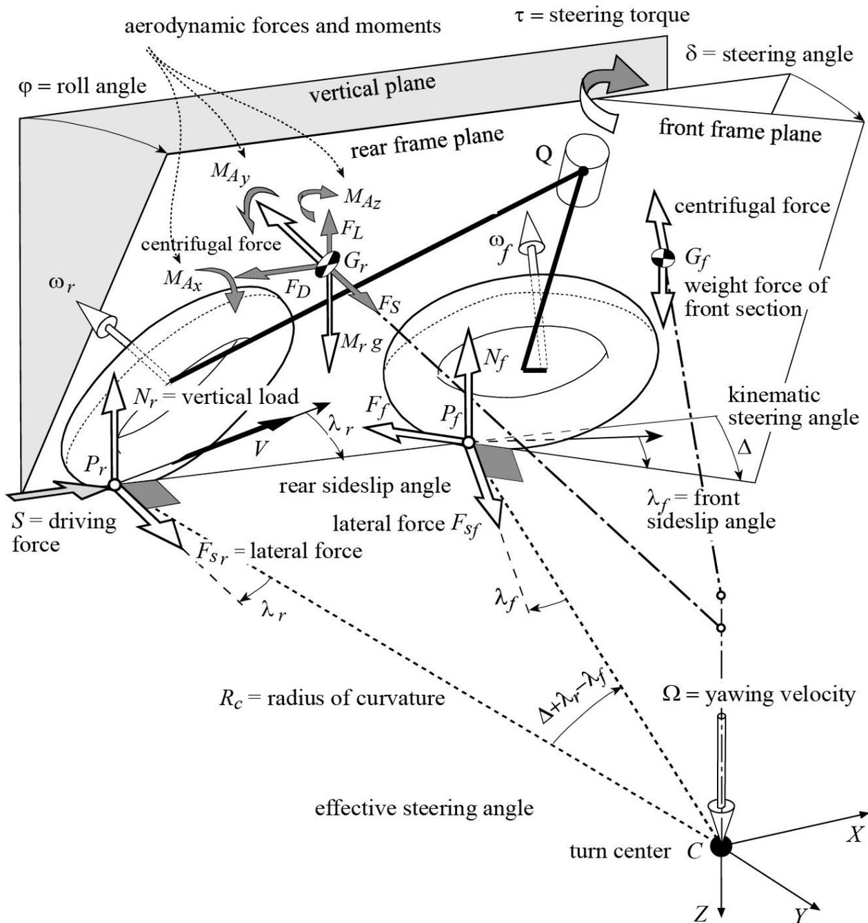
Figure 20, Steady turning bike forces
