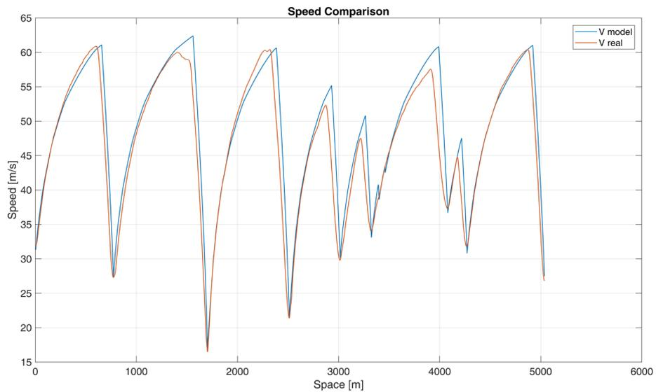
Figure 19, Speed comparison between reality and point mass model
