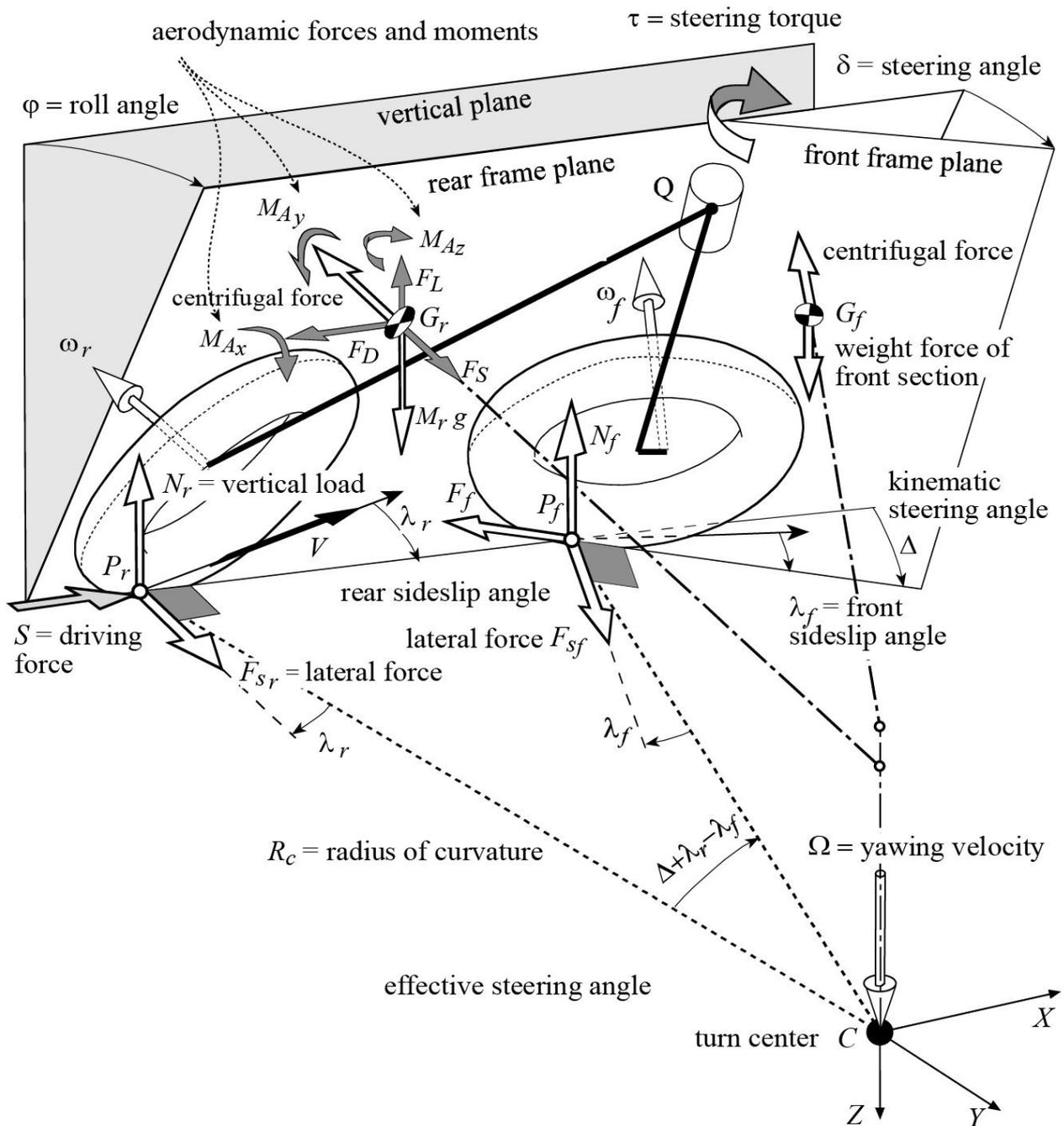
Figure 20, Steady turning bike forces
