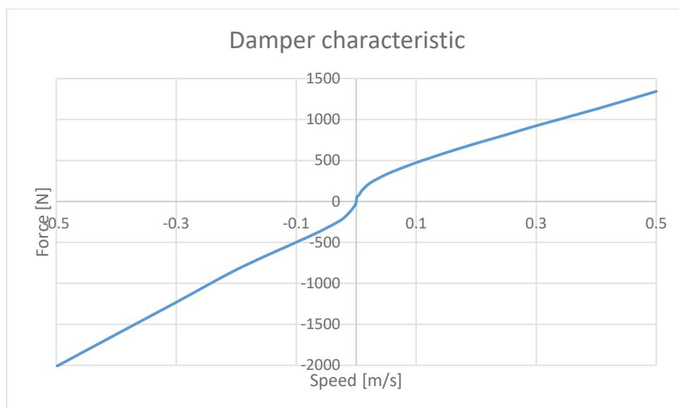
Figure 43, damper characteristics
