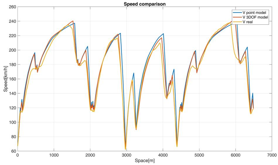
Figure 36, Phillip Island circuit real and model speed comparison
