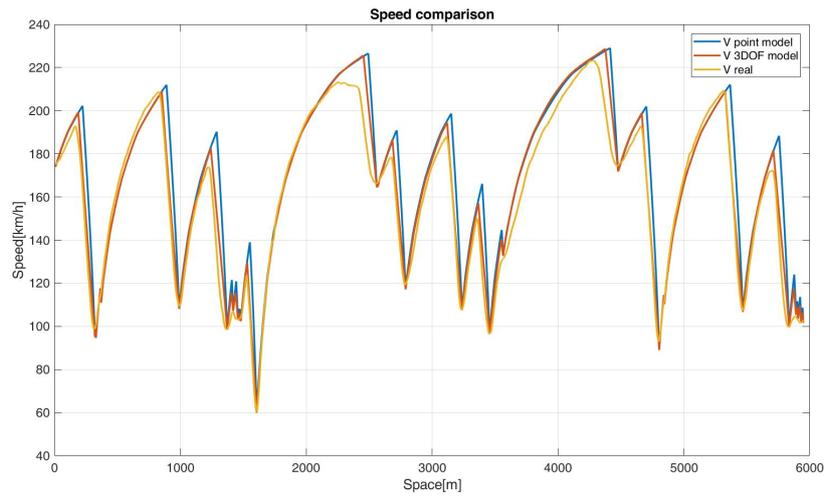
Figure 34, Assen circuit real and model speed comparison
