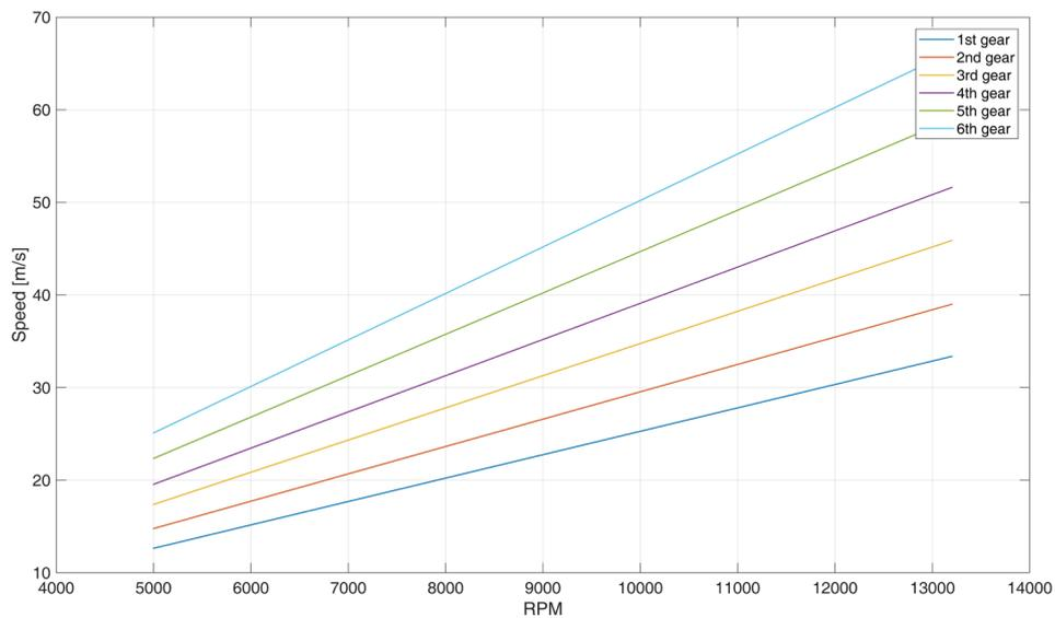
Figure 14, max speed per each gear
