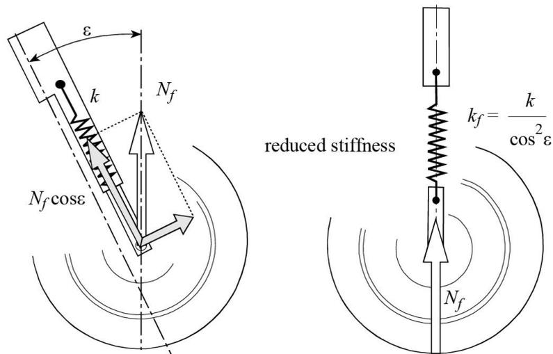
Figure 41, reduced front stiffness
