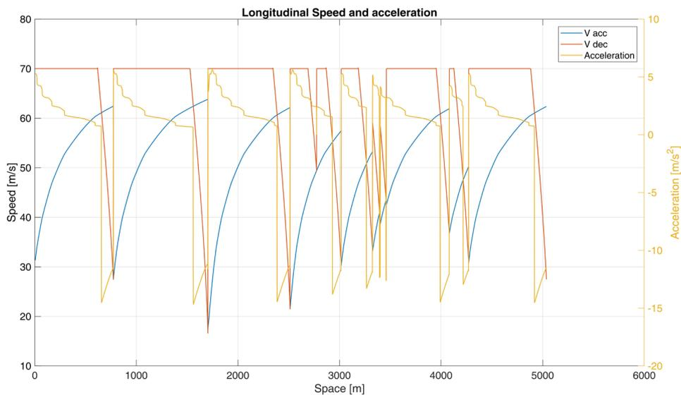
Figure 15, example of speed profile intersection, together with their relative acceleration
