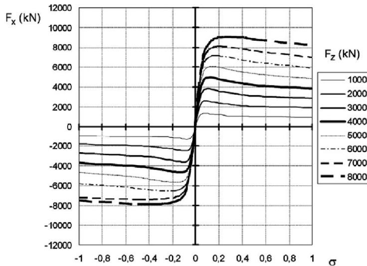
Figure 6, longitudinal force, varying slip
