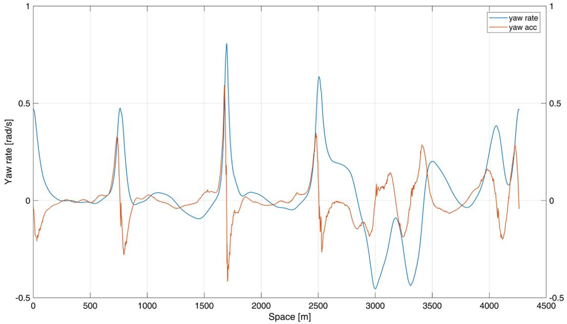
Figure 28, yaw acceleration and yaw rate
