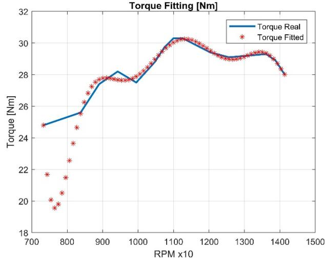
Figure 13, engine torque curve
