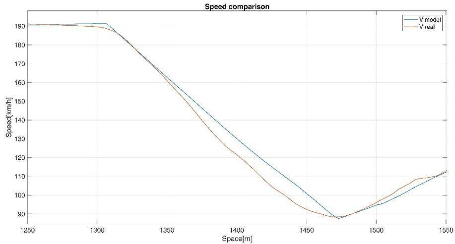
Figure 4, Example of a brake phase. (San Donato turn, Mugello circuit)
