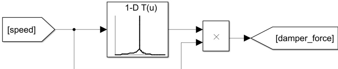
Figure 44, model damping force calculation
