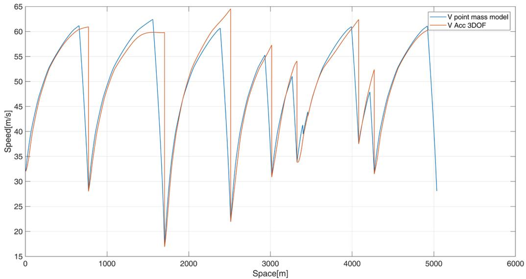
Figure 24, comparison between speed of 3dof model and point mass one
