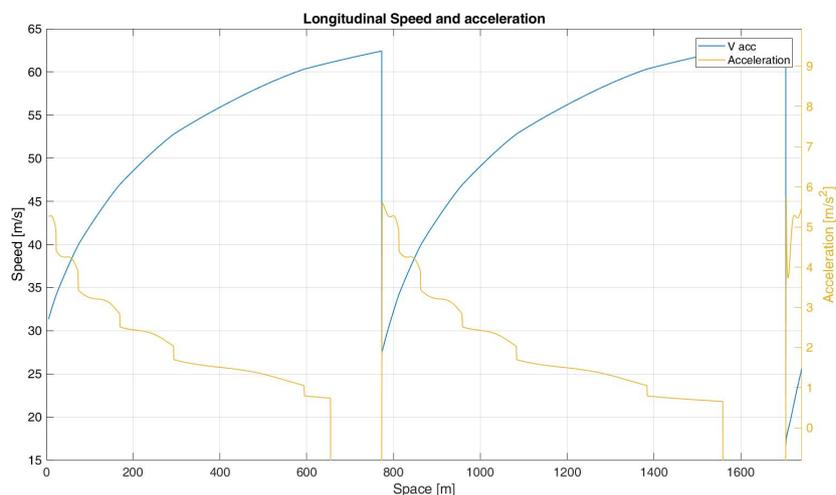
Figure 3, Example of speed profile and acceleration
