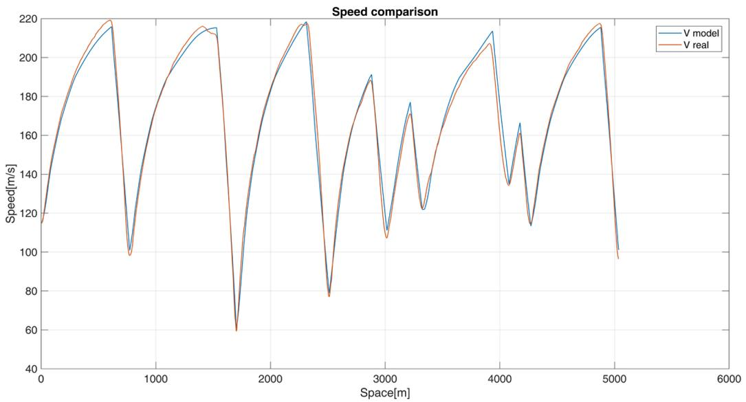
Figure 27, speed comparison 3DOF vs real profile
