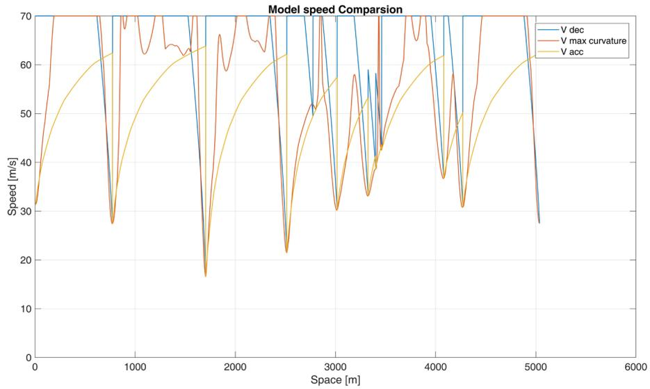
Figure 18, acceleration, deceleration speed profiles and max trajectory speed
