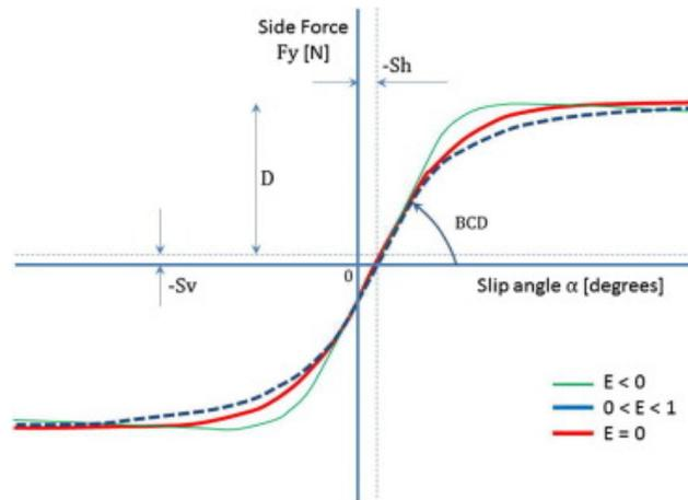
Figure 8, Typical Pacjeka force behavior with respect to sideslip variation
