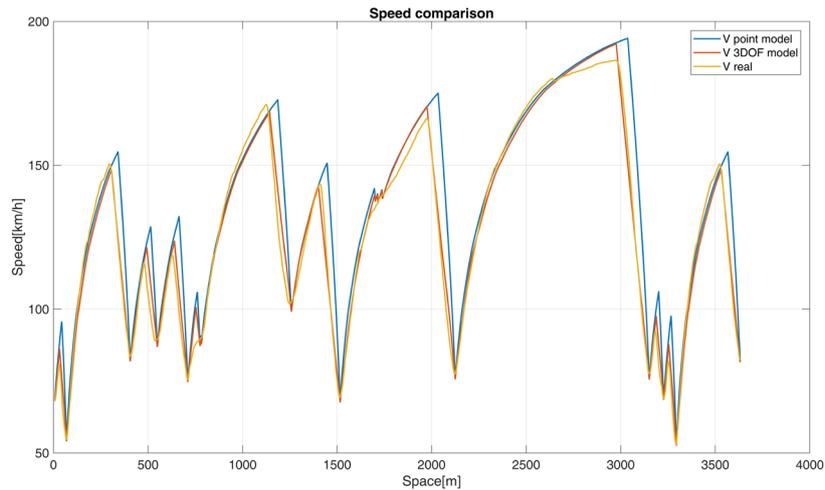
Figure 38, Cremona circuit real and model speed comparison
