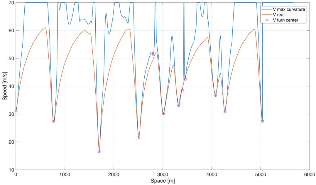
Figure 12, curvature dependent speed
