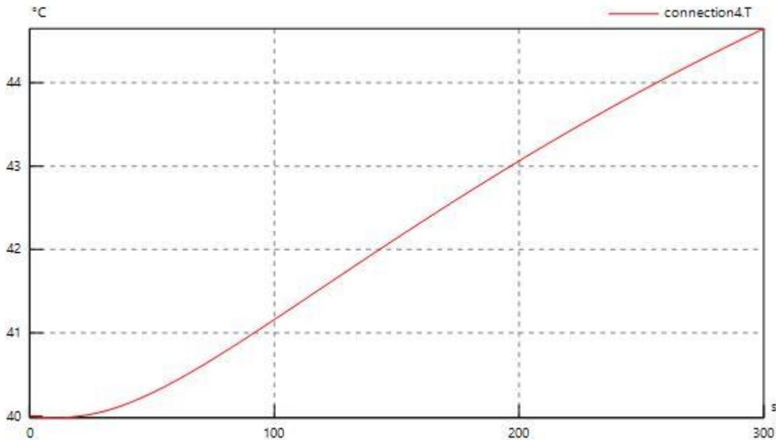
Temperature of coolant tank
