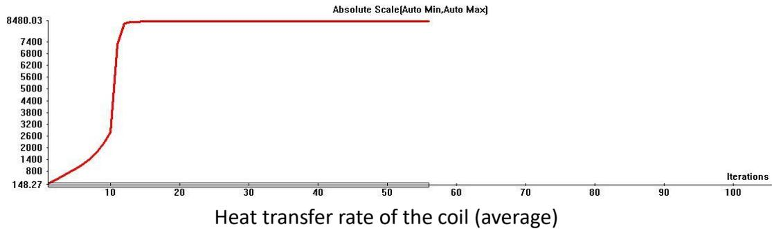
Because fixed the input power at 8500W, the heat transfer and heat flux remain the same. However, the temperature of the solid and fluid increase under the effect of the heat power. Moreover, the coil temperature is higher than previous case, the maximum of the temperature is near close to 70°C, and the average temperature is steely rising to around 62°C. The temperature is near the limit.
