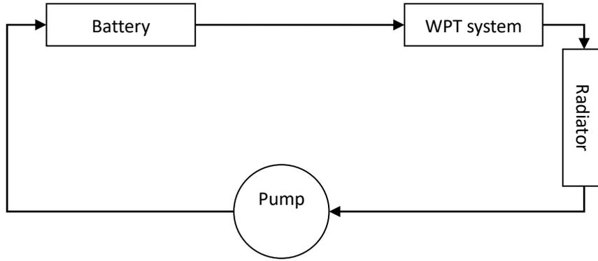
To ensure the temperature of WTP system satisfy the critical, the coolant temperature should be limited at a certain lever, by the way, the PCM can take half of the heat and storage it, thus, the cooling system are rarely asked to carry the rest of heat (about 5Kw).
