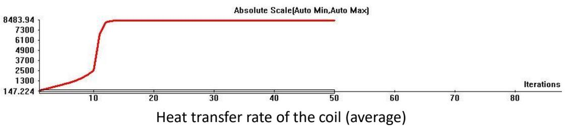
Apparently, the tendency resembles the case 1, but the value is higher. Particularly, the maximum temperature of the coil is 47.6104°C, and the pipe is warmer up to 35.8°C. In addition, because the temperature stabilizes, the heat transfer rate should correspond to the power of heat which is estimated 8.5KW .The heat flux is also increased due to some tolerance in calculation.
