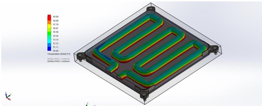
The pipe is also heated by the coil, the heat transfer from the contact surface of them and the temperature reduced with respect to the height of the pipe. The temperature ascends about 8°C.
