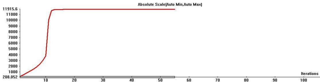
Surface heat flux of the coil (average)
