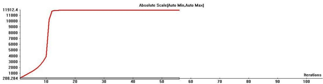
Surface heat flux of the coil (average)
