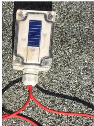
Fig. 4-5 Cella sensore in m-Si
