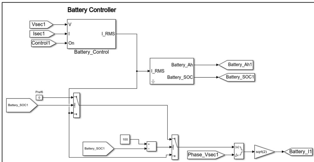
Figure 4-19: scheme of the battery control
