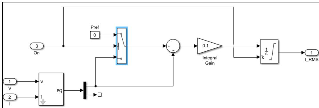
**Figure 4-20: battery control**
