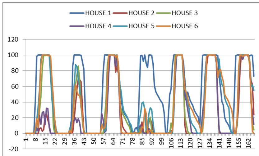
Figure 8-29: SOC of batteries
