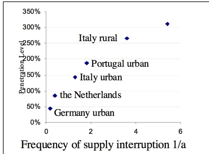
Figure 3-7: System unavaible with the DG penetration
