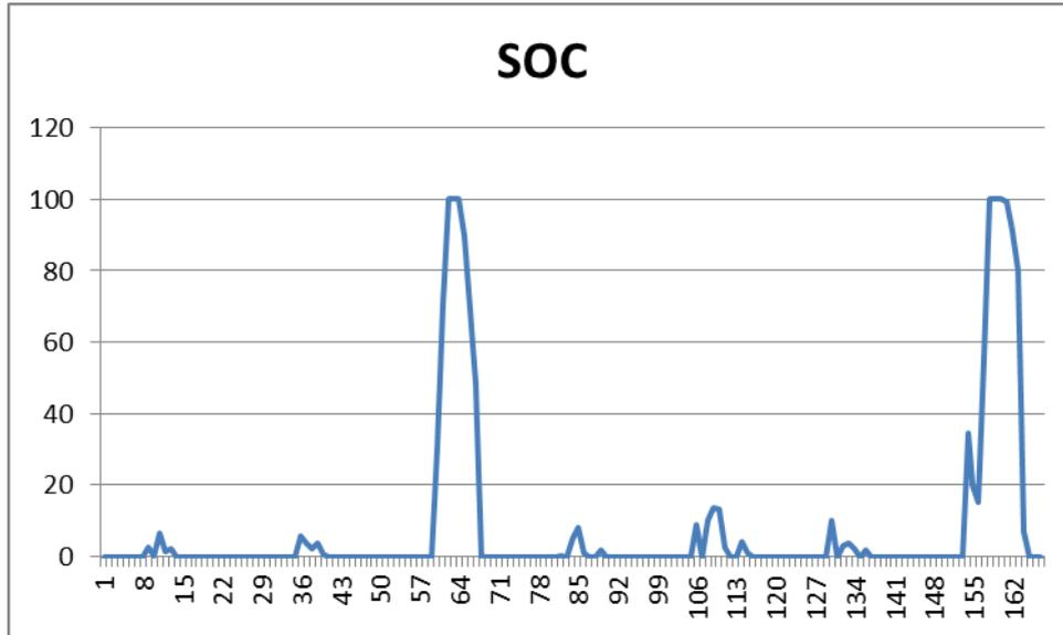
Figure 8-10: SOC of battery
