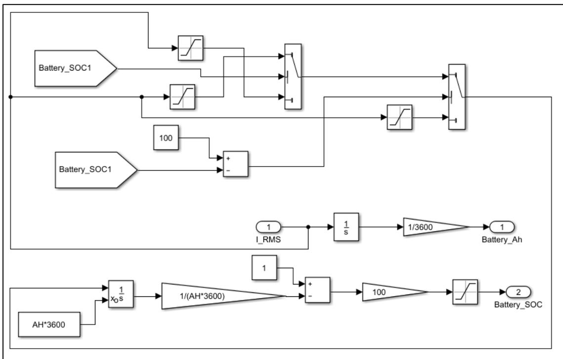
Figure 4-22: SOC and Ah scheme
