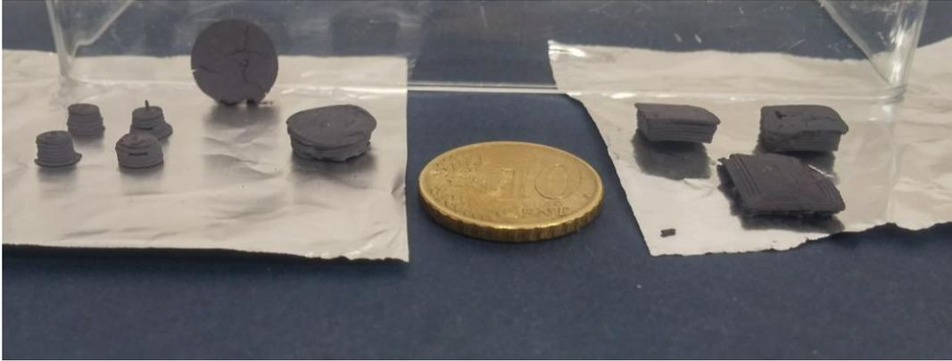
Figure 6.32:  $Mg_2Si$  Printed pieces (ratio 55 : 45)
