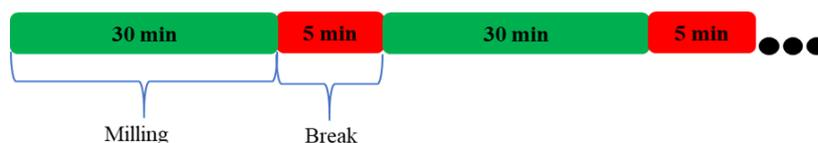
Figure 5.6: Scheme of the operating routine for milling operation. Steps of half an hour milling are alternate with breaks of 5 minutes to avoid overheating.
