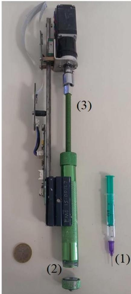
Figure 6.1: Detail of the printing cylinder and syringe
