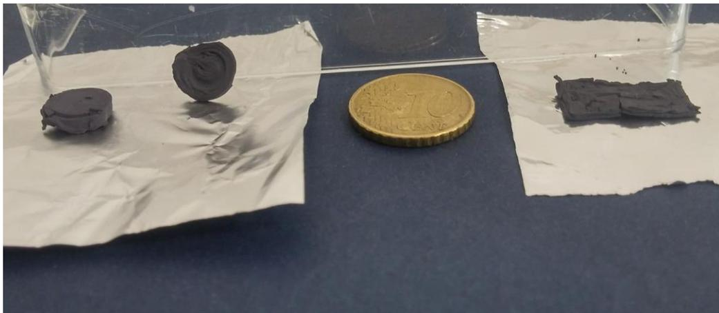
Figure 6.33:  $Mg_2Si$  Printed pieces (ratio 57 : 43)
