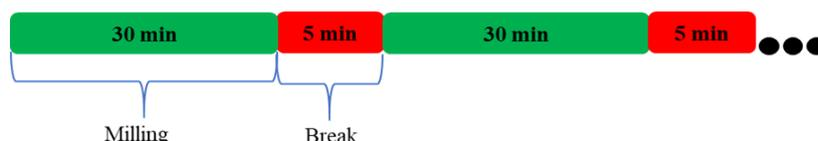
Figure 5.6: Scheme of the operating routine for milling operation.
