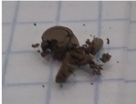
*Figure 6.35: Broken cylinder after the first sintering attempt; the cylinder broke while extracting from the oven*
