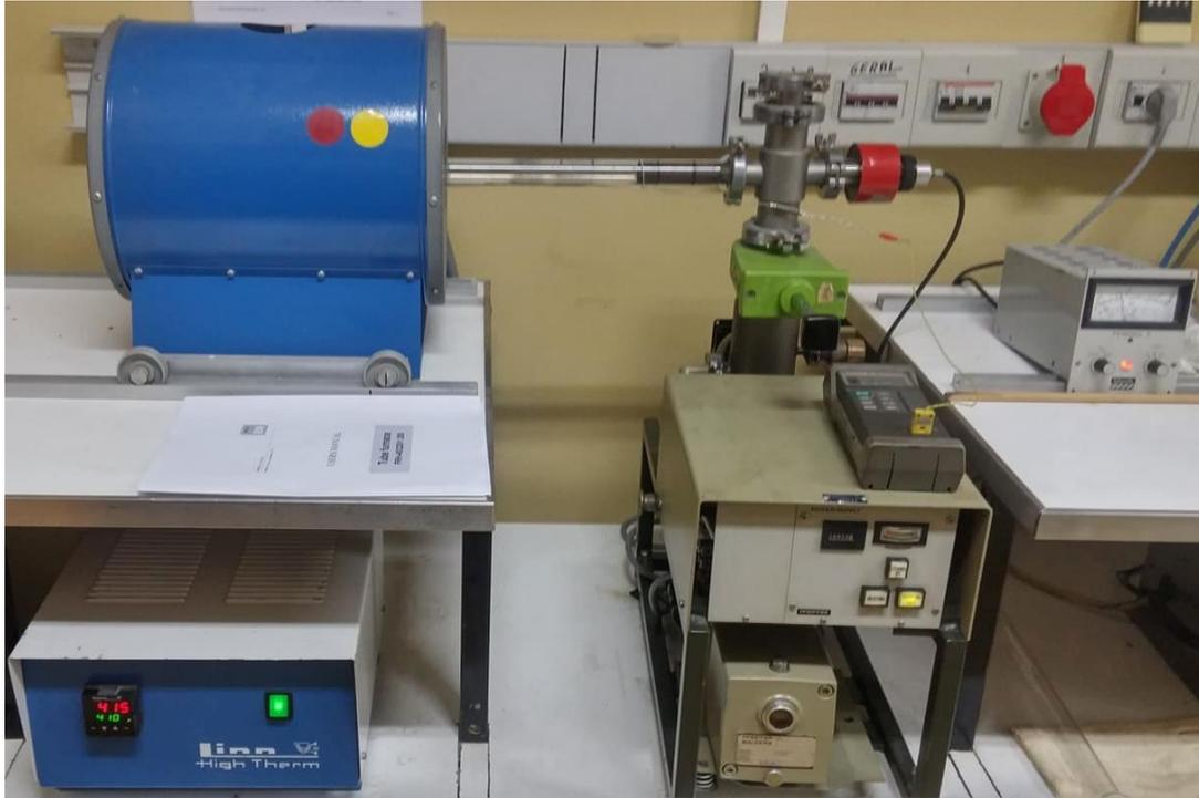
*Figure 5.12: Tubular oven used for annealing*
