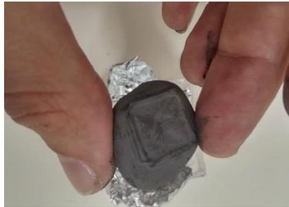
Figure 6.16: Printed pieces using only dodecanol and Si powder (Group 2), formulation\*)
