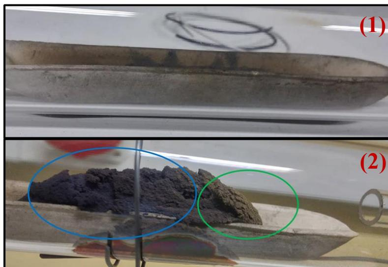
Figure 5.16: Pictures of the crucible inside the quartz tube, before (1) and after (2) argon annealing. After the treatment it is visible an increase of volume of the powder inside the crucible and at the same a color difference is visible (blue and grey/brown, left and right side).
