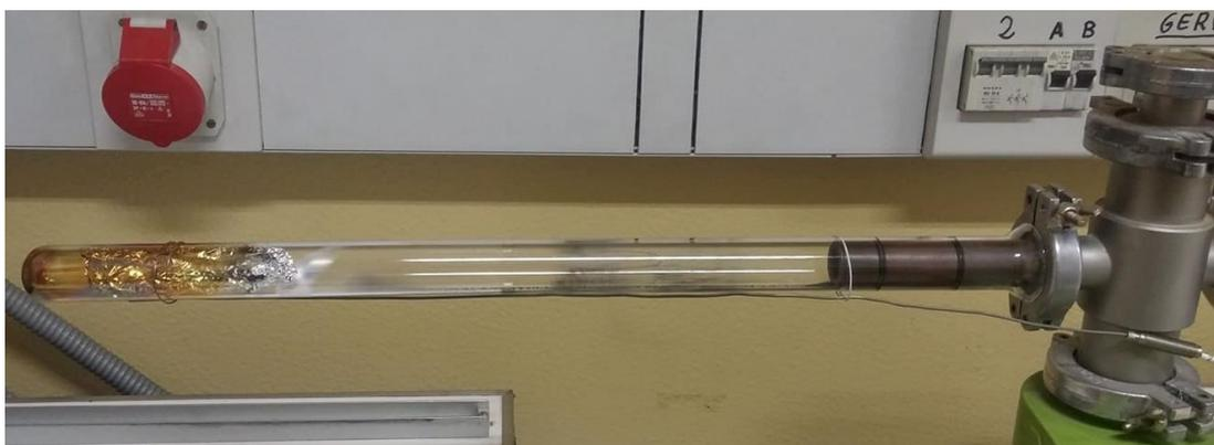
*Figure 5.14: Picture of the quartz tube still fixed on the support, after the oven was slid away in the end of thermal treatment. The tube was removed, and the crucible extracted only after reaching room temperature. The cooling, so, could happen while inside the tube the atmosphere was still inert.*
