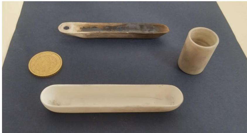
*Figure 5.13: Picture of the alumina crucibles used.*
