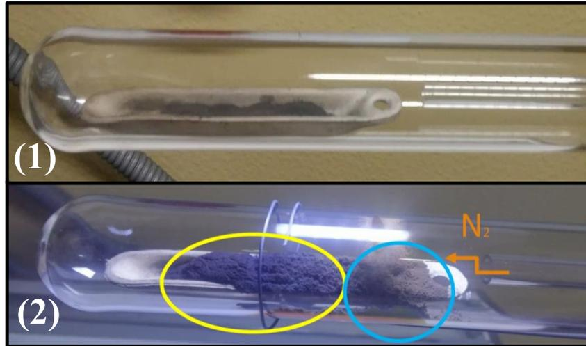
Figure 5.15: Pictures of the crucible inside the quartz tube before (1) and after (2) thermal treatment in  $N_2$  atmosphere. After the annealing it is visible an increase of volume of the powder inside the crucible and at the same a color difference is visible (blue and grey/brown, left and right side).
