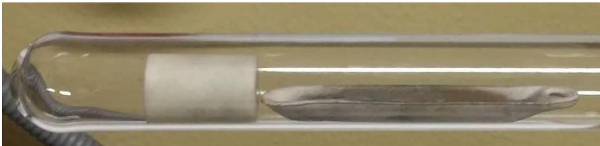
*Figure 5.19: Alumina crucibles containing a mixture of Mg and Si powder, inside the furnace quartz tube*
