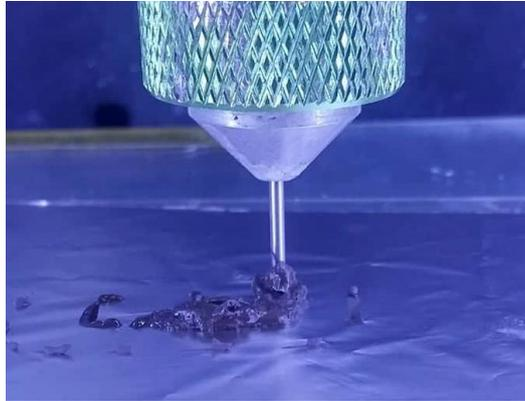
*Figure 6.25: Particular of the printing process of milled silicon powder: lumps formed, turning impossible the printing*
