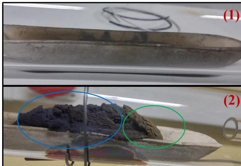
Figure 5.16: Pictures of the crucible inside the quartz tube, before (1) and after (2) argon annealing. After the treatment it is visible an increase of volume of the powder inside the crucible and at the same a color difference is visible (blue and grey/brown, left and right side).
