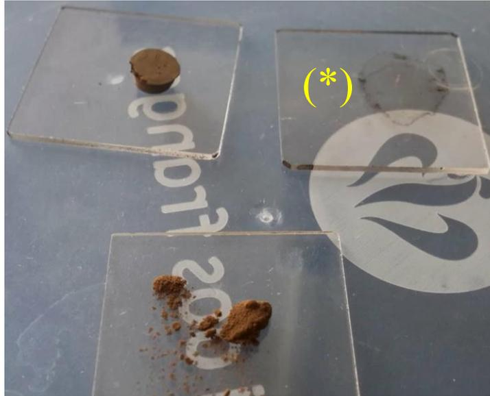
Figure 6.37: After thermal treatment the polystyrene completely vanished (\*), while the cylinder and the powder turned brown.
