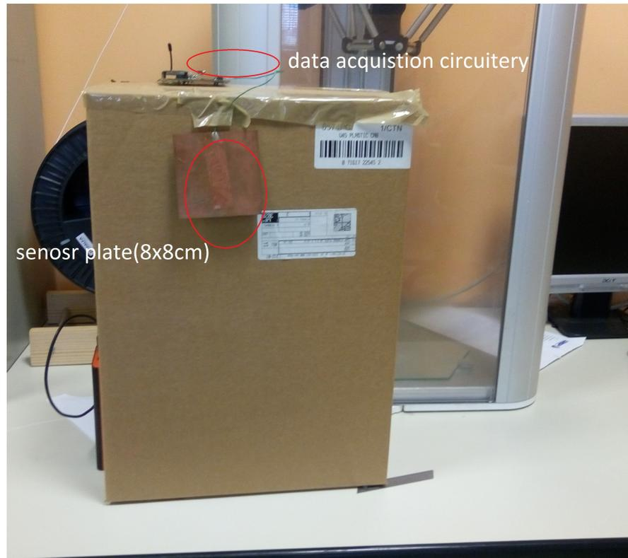
FIGURE 3.12: Experimental setup for checking the response of the transducer (capacitive sensor)
