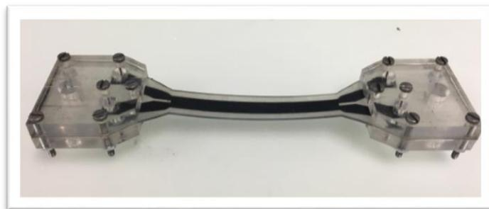
Figure 4-4: Capacitive stretchable sensor tested at EPFL [23].
