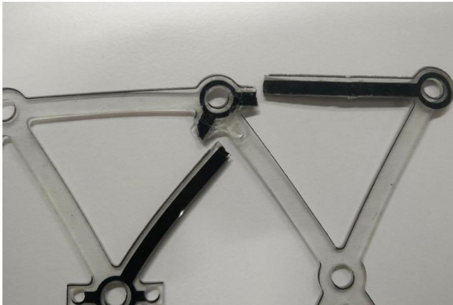
Figure 5-7: Sylgard-184 broken net.
