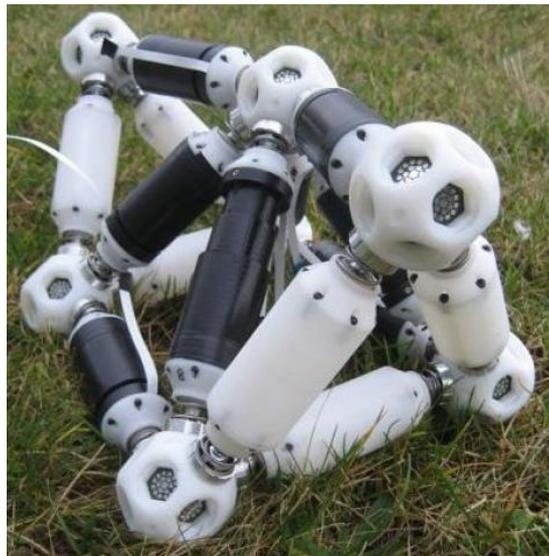
Figure 2-7: Odin robot with 21 modules: 8 telescoping link modules (black links), 6 rigid passive link modules (white links), and 7 joint modules.
