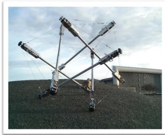
Figure 1-9: Super Ball Bot all-in-one landing and mobility platform based on tensegrity structures. All credits to NASA research center.
