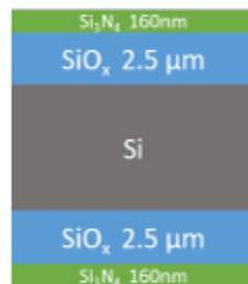
FIGURE 3.9: Starting wafer, provided by *Lionix*<sup>®</sup>
