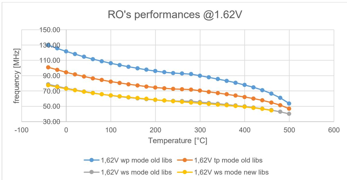
Figure 22: RO's frequency driven at 1.62V
