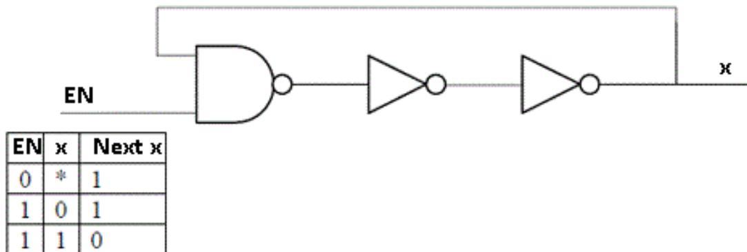
Figure 19: 3-stages Ring Oscillator with Enable signal
