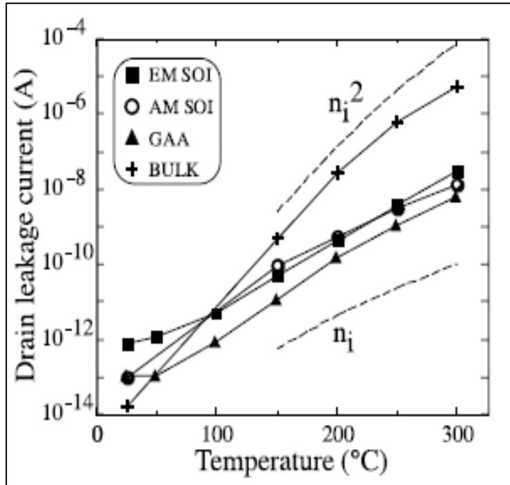
Figure 12: Drain leakage current vs temperature
