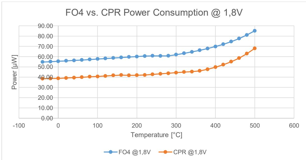
Figure 55: FO4 vs. CPR power consumption as a function of temperature driven at 1.8V
