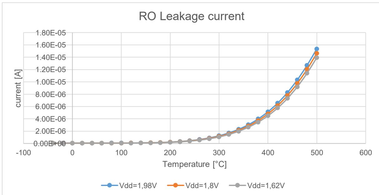
Figure 32: RO's leakage current vs temperature
