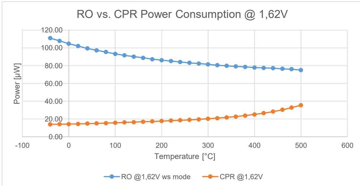
Figure 51: RO vs. CPR power consumption as a function of temperature driven at 1.62V
