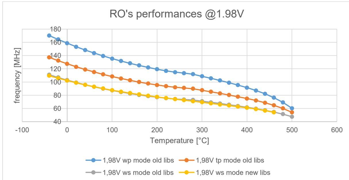
Figure 20: RO's frequency driven at 1.98V
