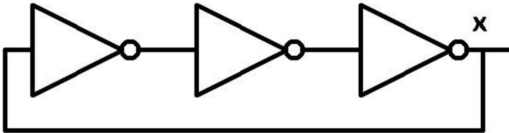
Figure 18: 3-stages Ring Oscillator
