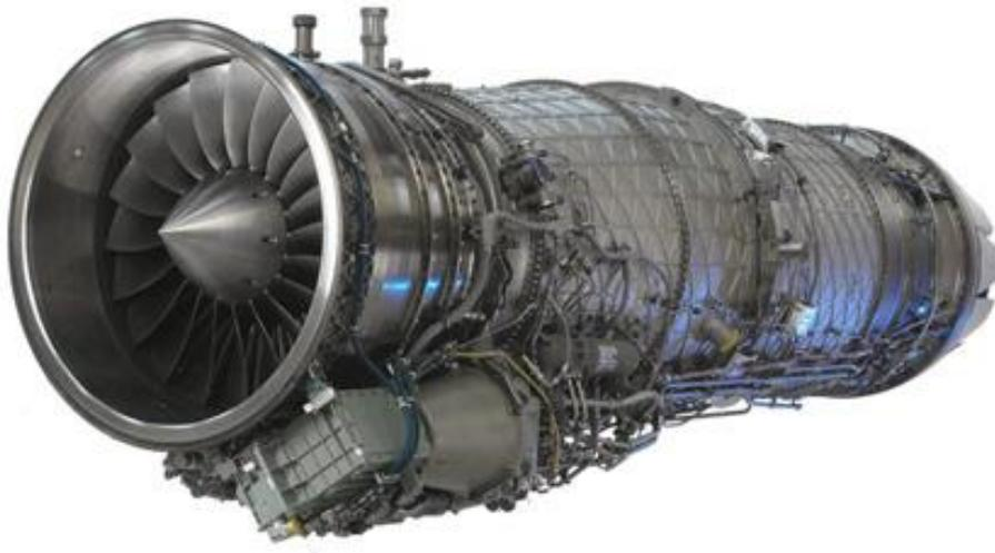
Figure 3: Aircraft engine with electronic controls
