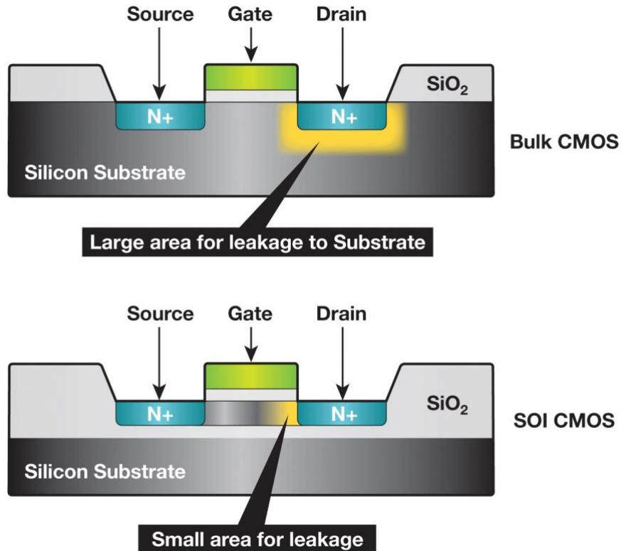
Figure 1: Leakage-current paths bulk CMOS and SOI CMOS
