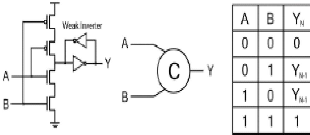
Figure 38: C-element, symbol and logic function
