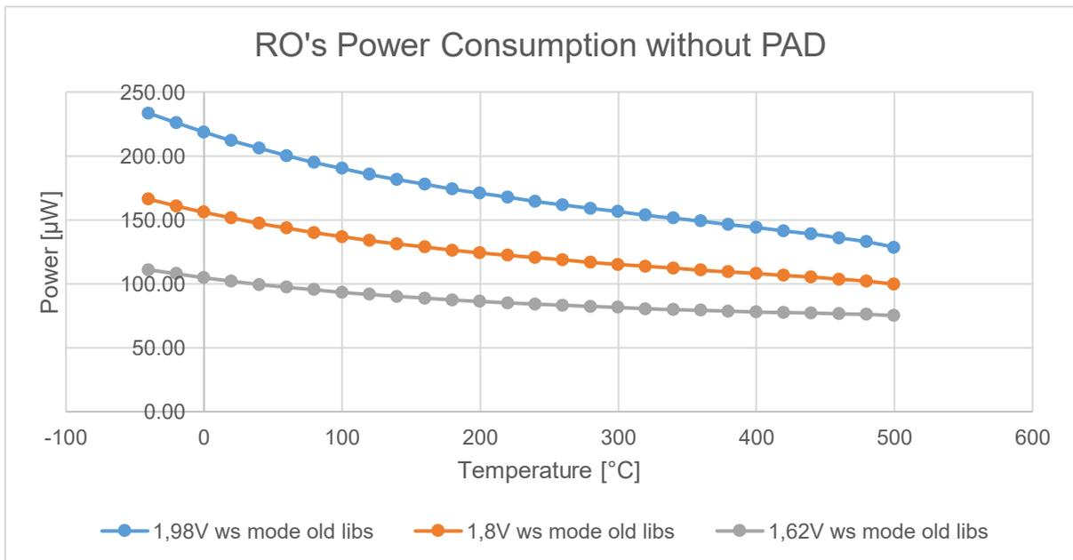
Figure 26: RO's consumed power vs temperature
