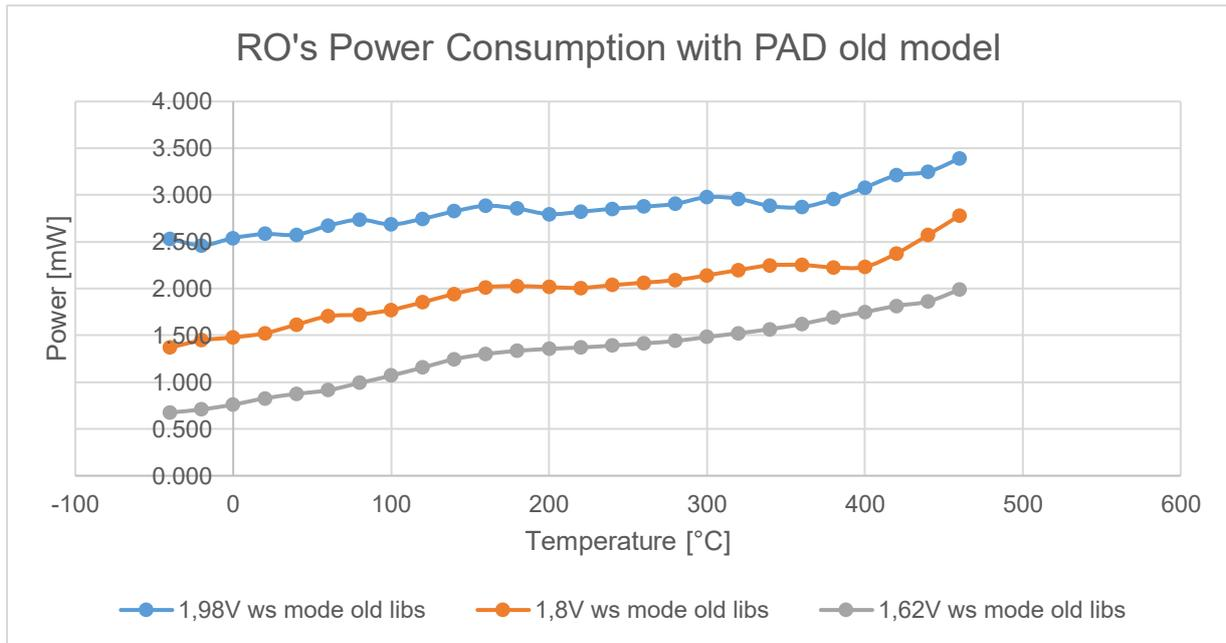
Figure 27: RO's consumed power vs temperature
