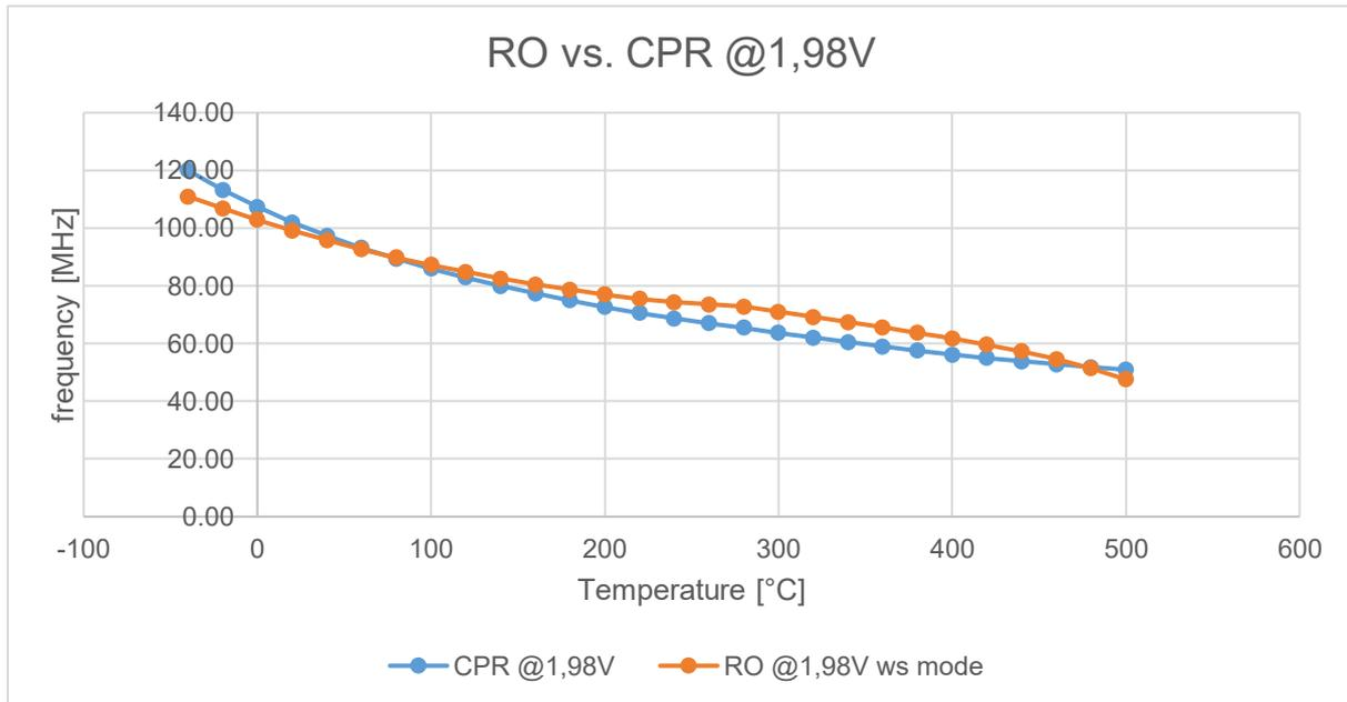
Figure 46: RO vs. CPR frequency as a function of temperature driven at 1.98V
