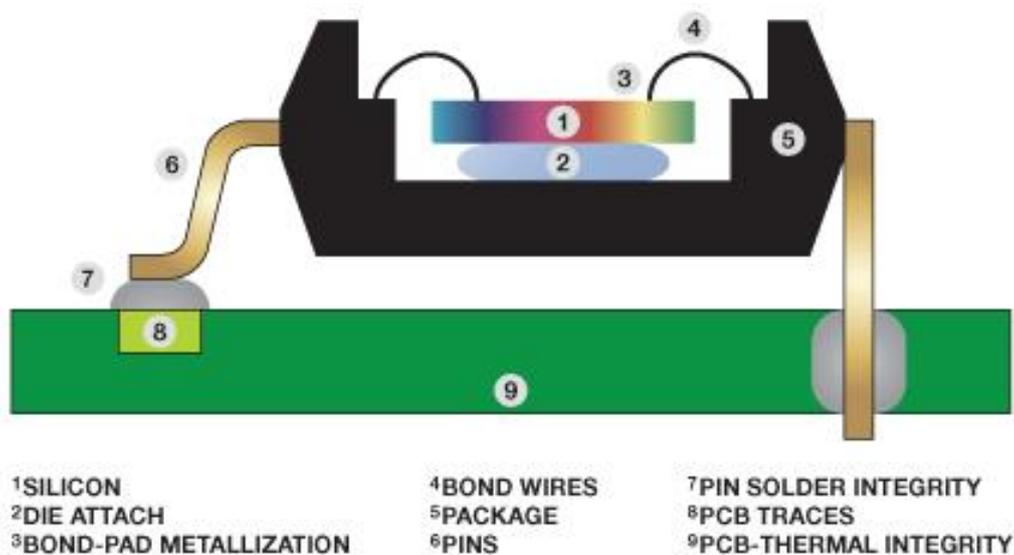
Figure 5: Elements of IC packaging and mounting
