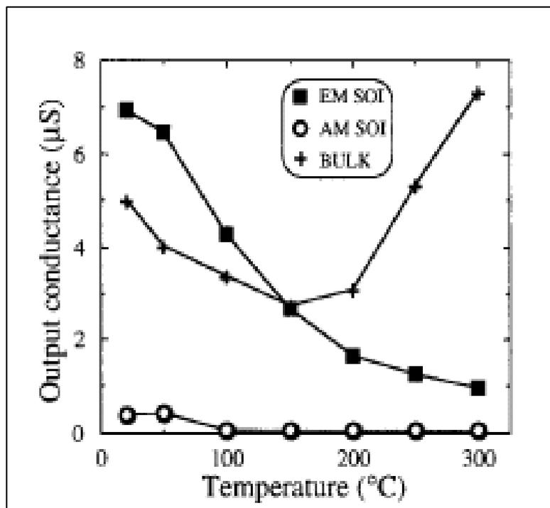
Figure 14: Output conductance vs temperature
