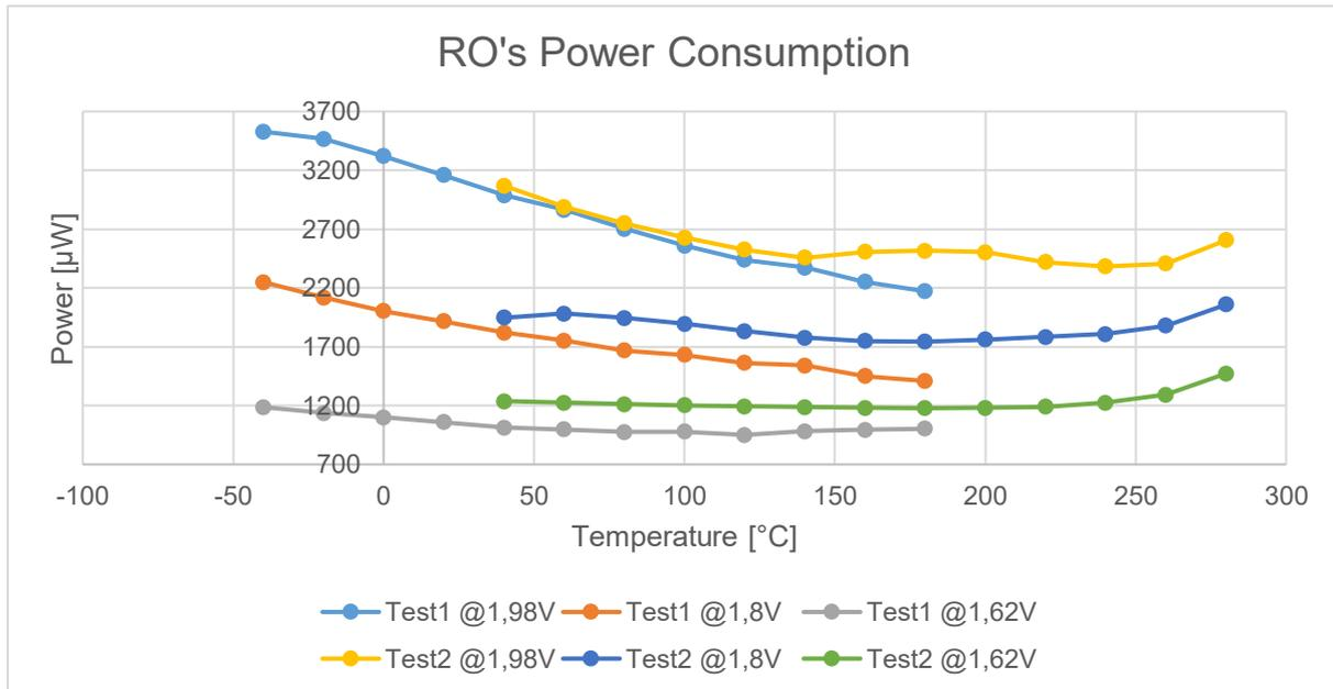
Figure 62: RO's power consumption vs temperature
