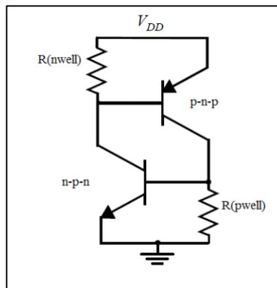
Figure 70: Equivalent circuit of the thyristor
