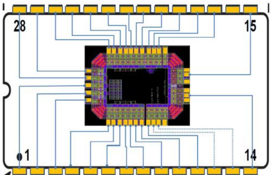
Figure 60: Wires' connection inside the package
