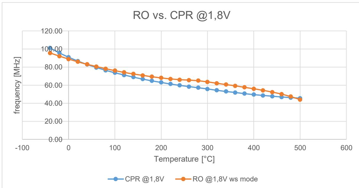
Figure 48: RO vs. CPR frequency as a function of temperature driven at 1.8V
