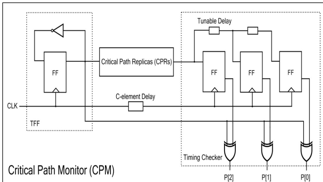
Figure 37: Critical Path Monitor
