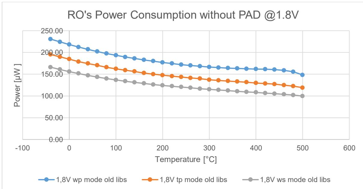
Figure 24: RO without PAD power consumption driven at 1.8V
