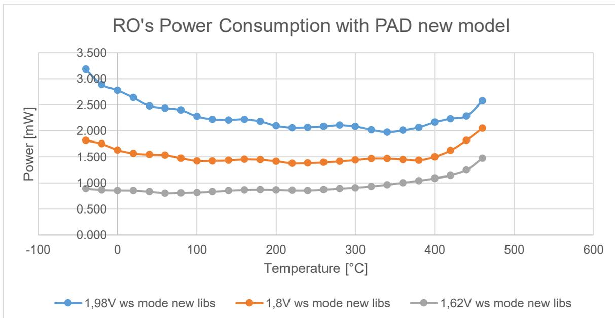
Figure 28: RO's consumed power vs temperature
