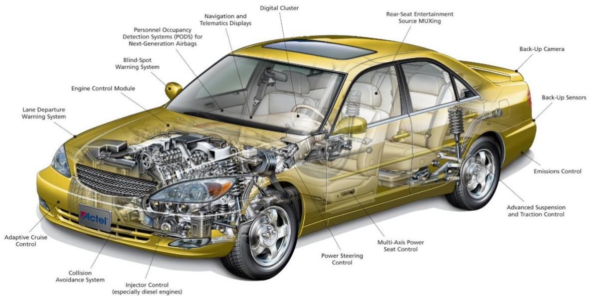
Figure 4: Electronics in automotive
