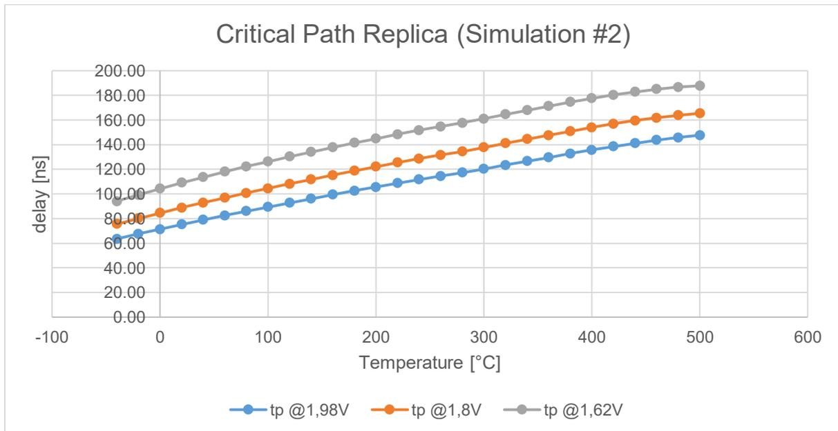
Figure 42: CPR's delay vs temperature (Simulation #2)
