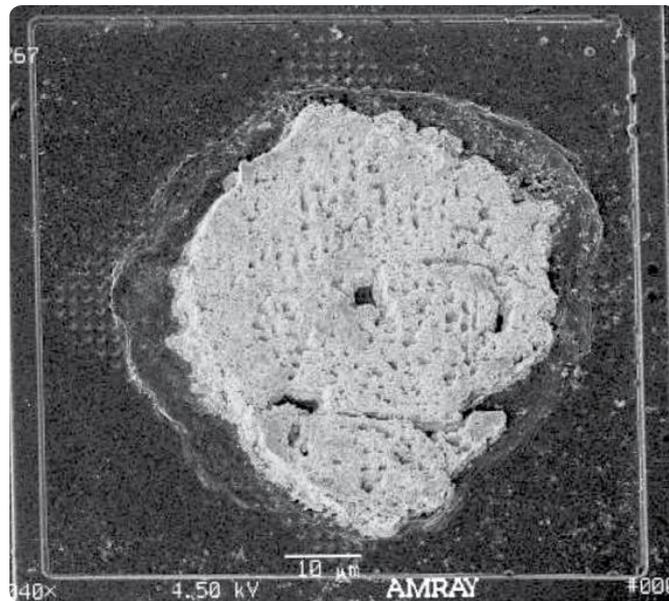
Figure 6: Kirkendall voids after bond failure
