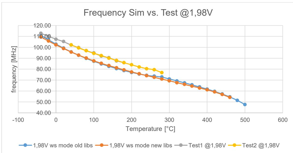
Figure 63: Simulation and Test frequencies driven at 1.98V
