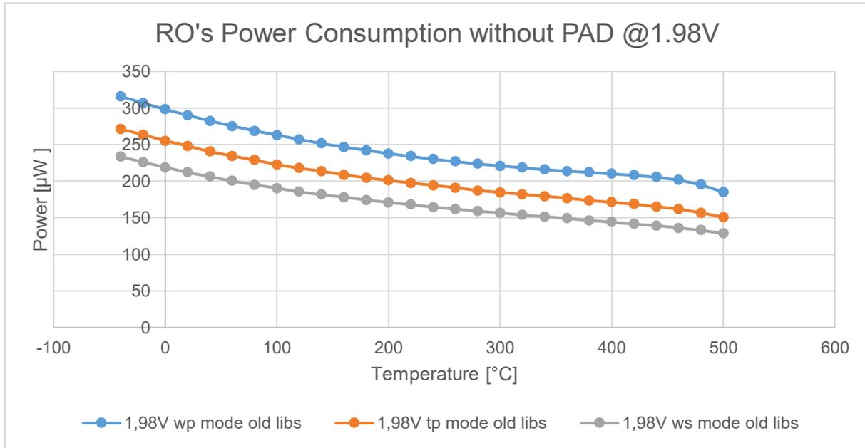
Figure 23: RO without PAD power consumption driven at 1.98V
