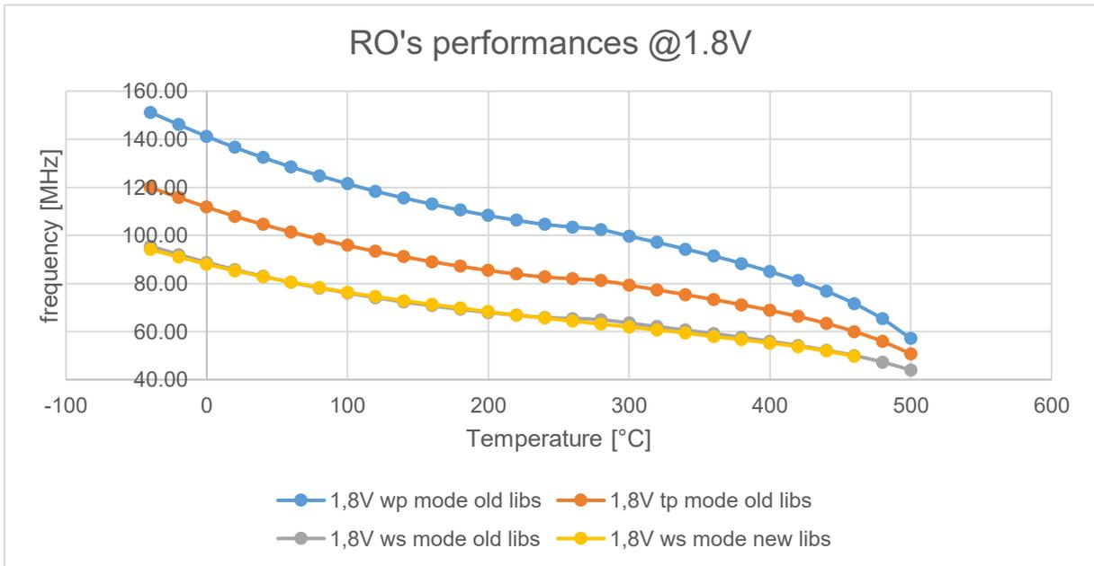
Figure 21: RO's frequency driven at 1.8V
