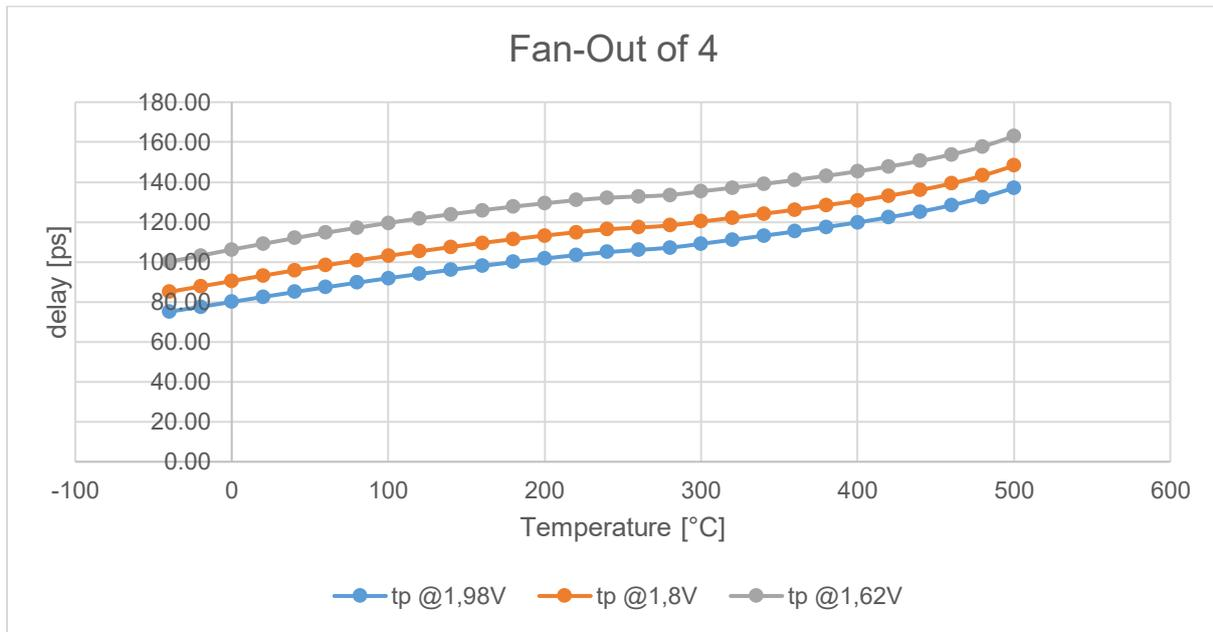
Figure 34: F04 vs temperature
