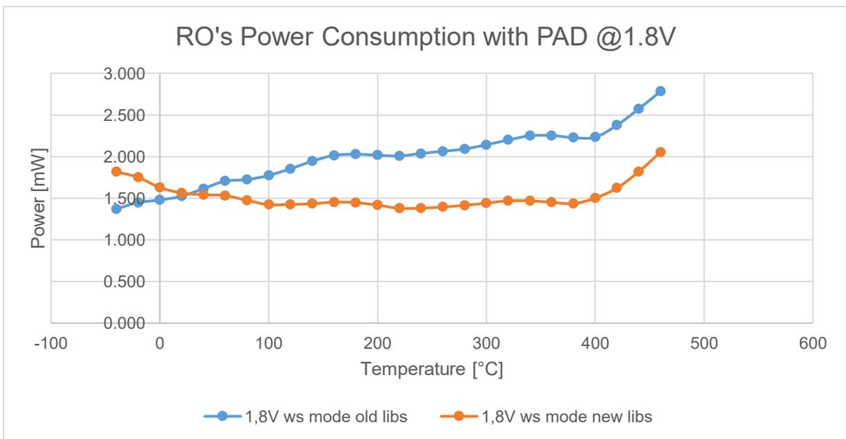
Figure 30: RO's consumed power vs temperature driven at 1.8V
