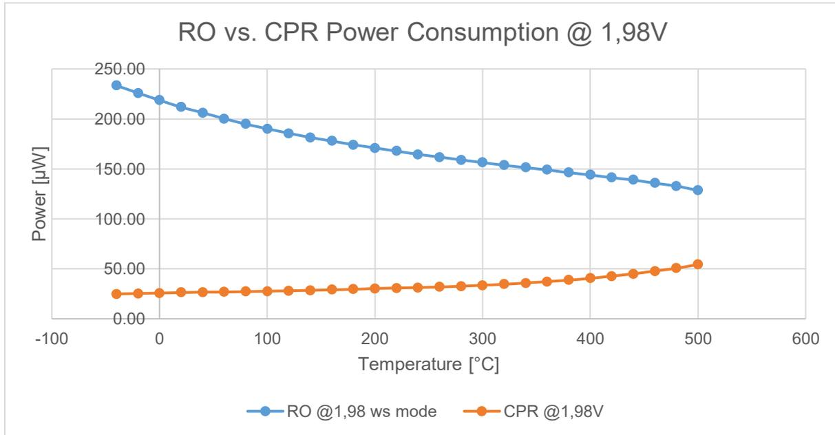
Figure 47: RO vs. CPR power consumption as a function of temperature driven at 1.98V
