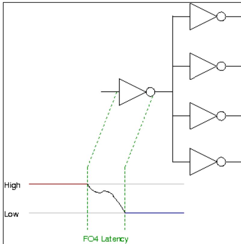
Figure 33: Fan-out of 4 latency
