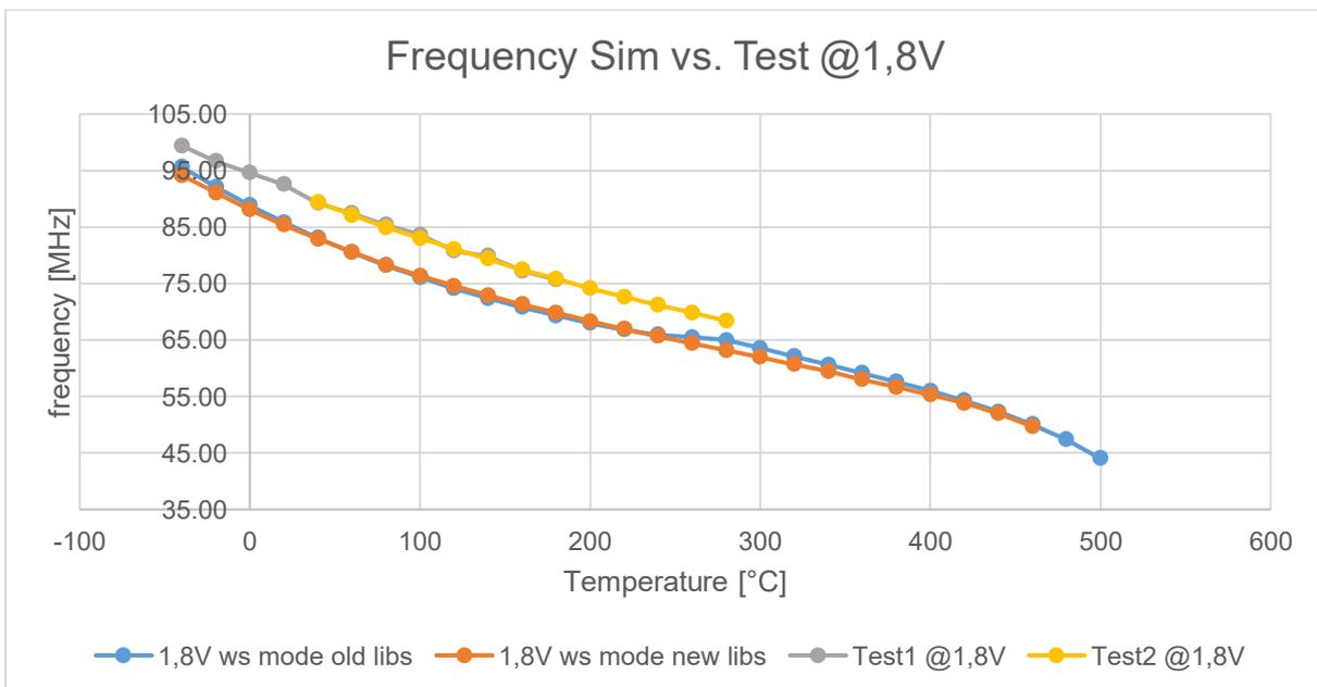
Figure 65: Simulation and Test frequencies driven at 1.8V
