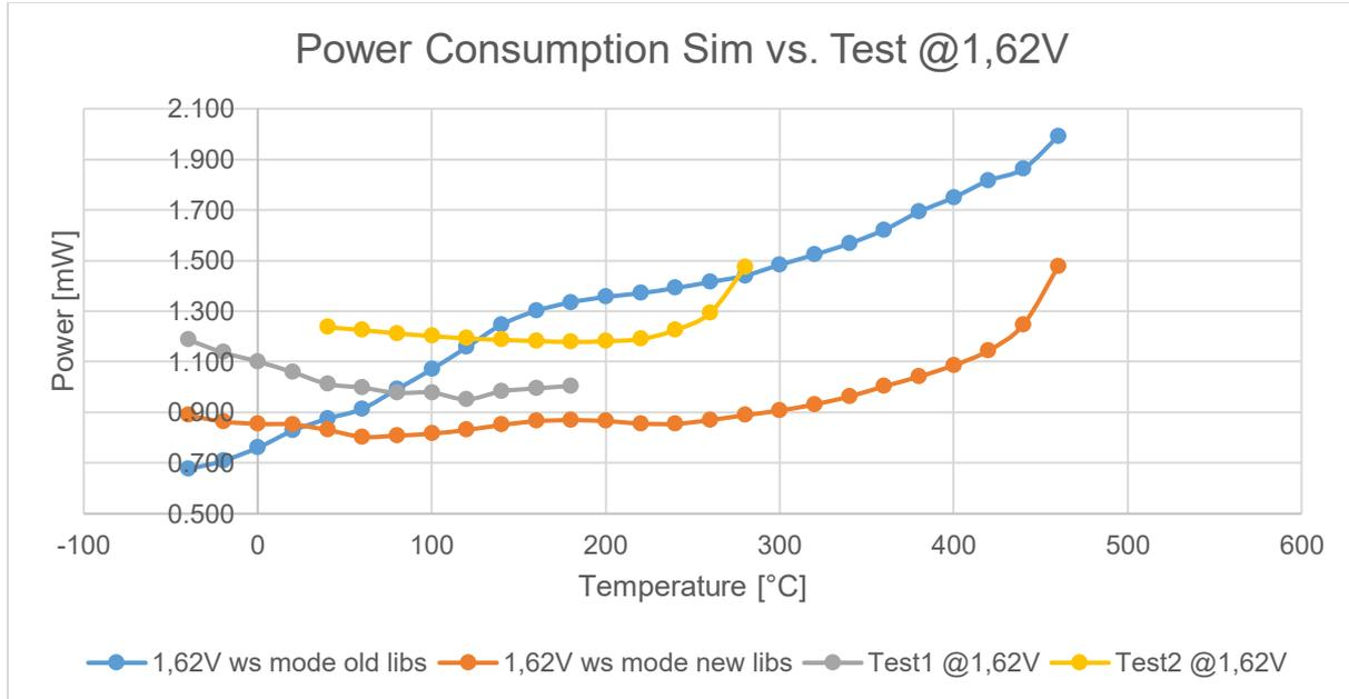
Figure 68: Simulation and Test power consumptions driven at 1.62V
