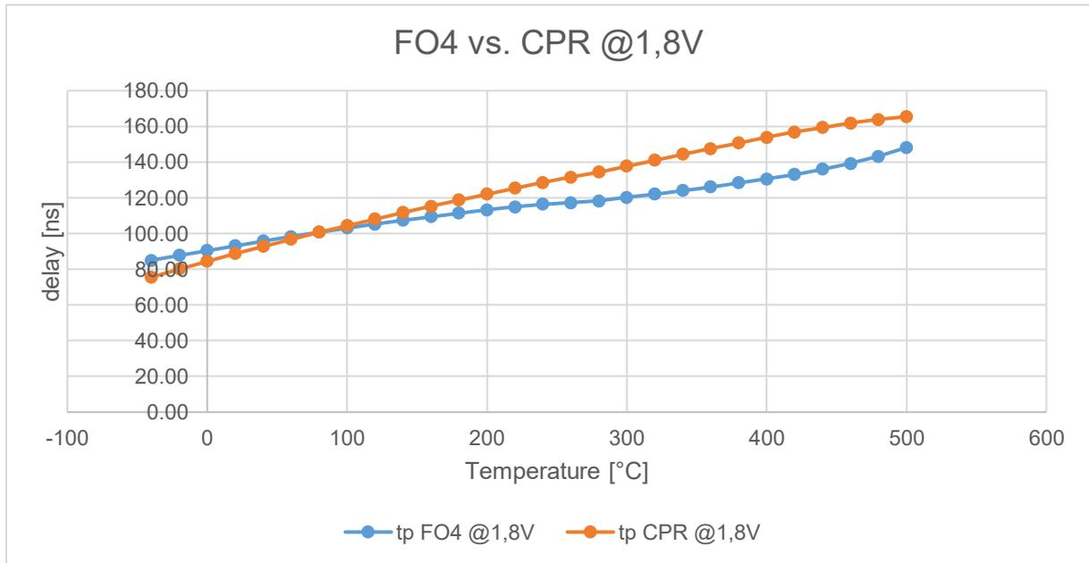
Figure 54: FO4 vs. CPR propagation time as a function of temperature driven at 1.8V
