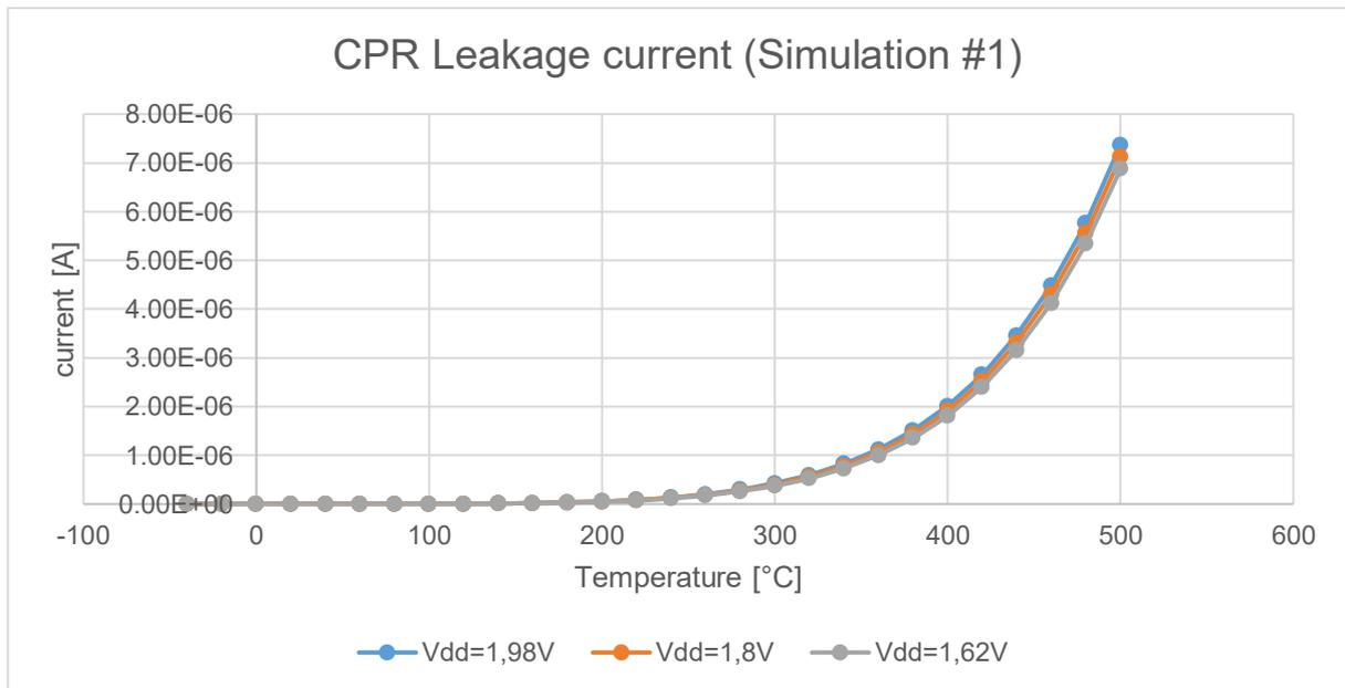
Figure 45: CPR's leakage current vs temperature
