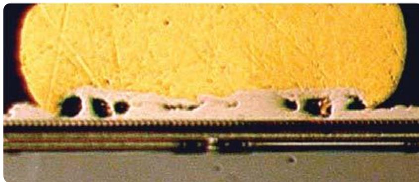
Figure 7: Au/Al InterMetallic Compound growth after 500 hours at high temperature
