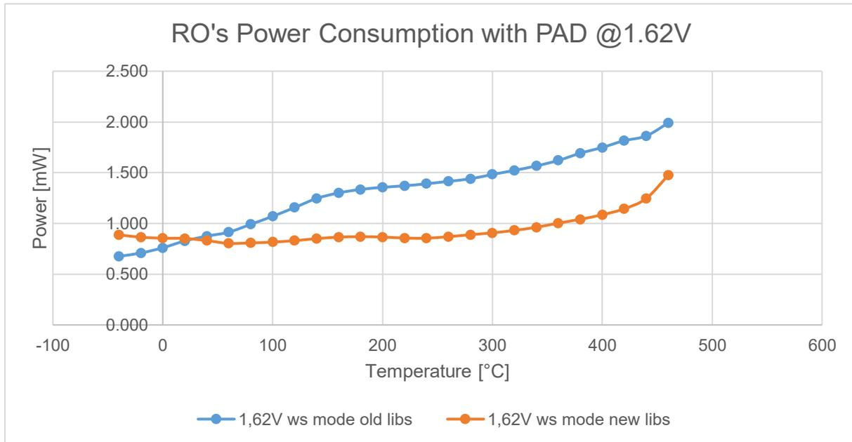
Figure 31: RO's consumed power vs temperature driven at 1.62V
