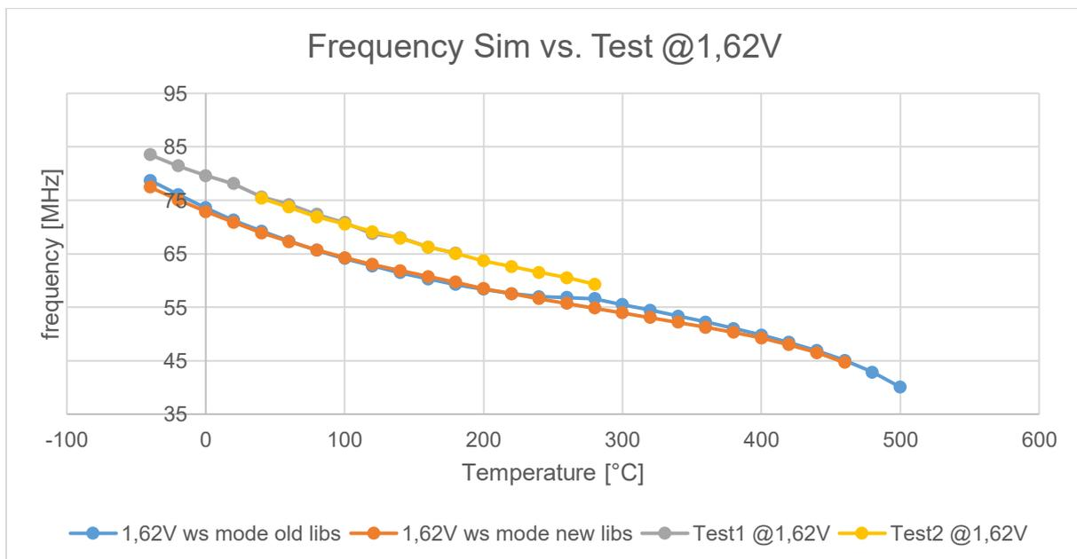
Figure 67: Simulation and Test frequencies driven at 1.62V
