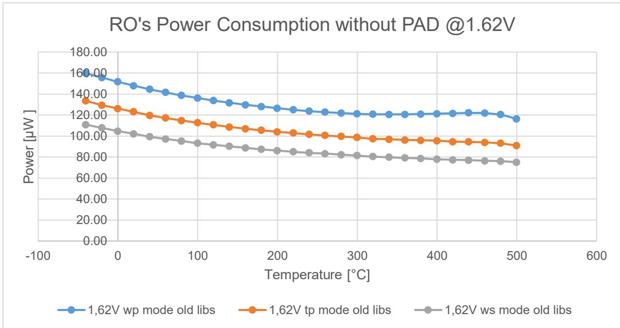
Figure 25: RO without PAD power consumption driven at 1.62V
