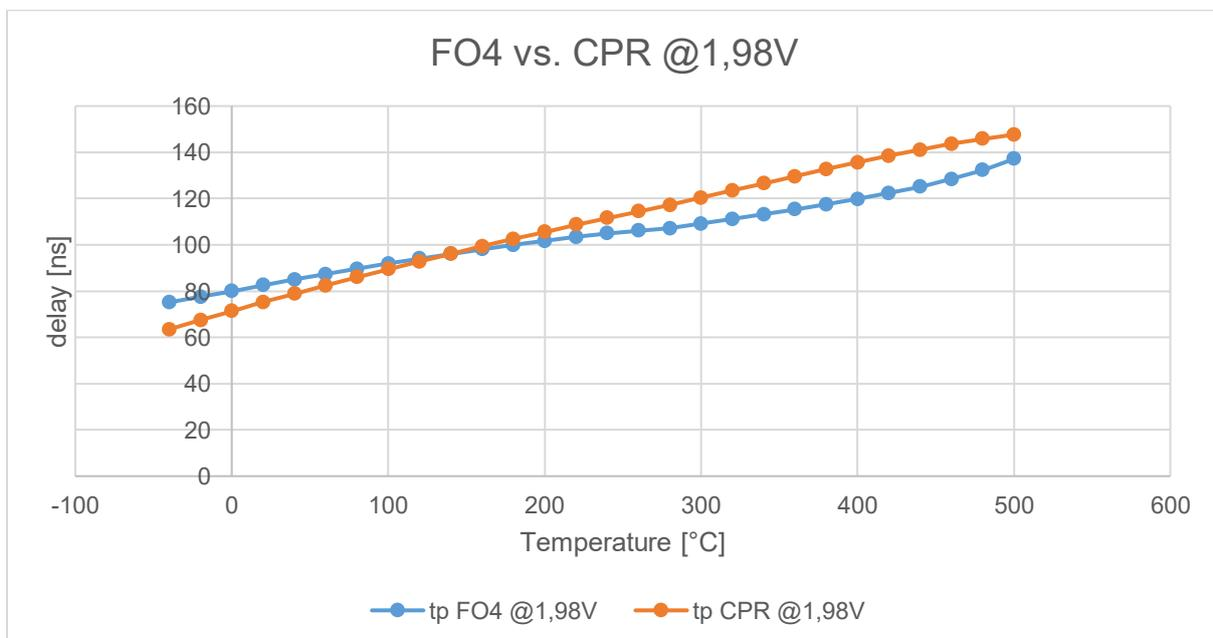
Figure 52: FO4 vs. CPR propagation time as a function of temperature driven at 1.98V
