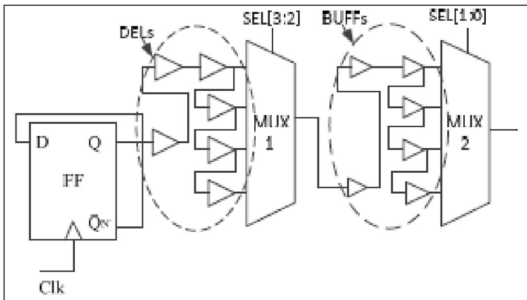
Figure 40: Configurable Critical Path Replica
