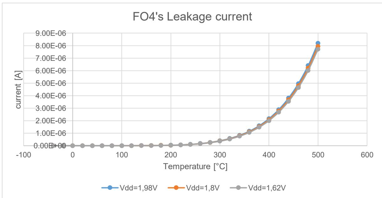
Figure 36: FO4's leakage current vs temperature
