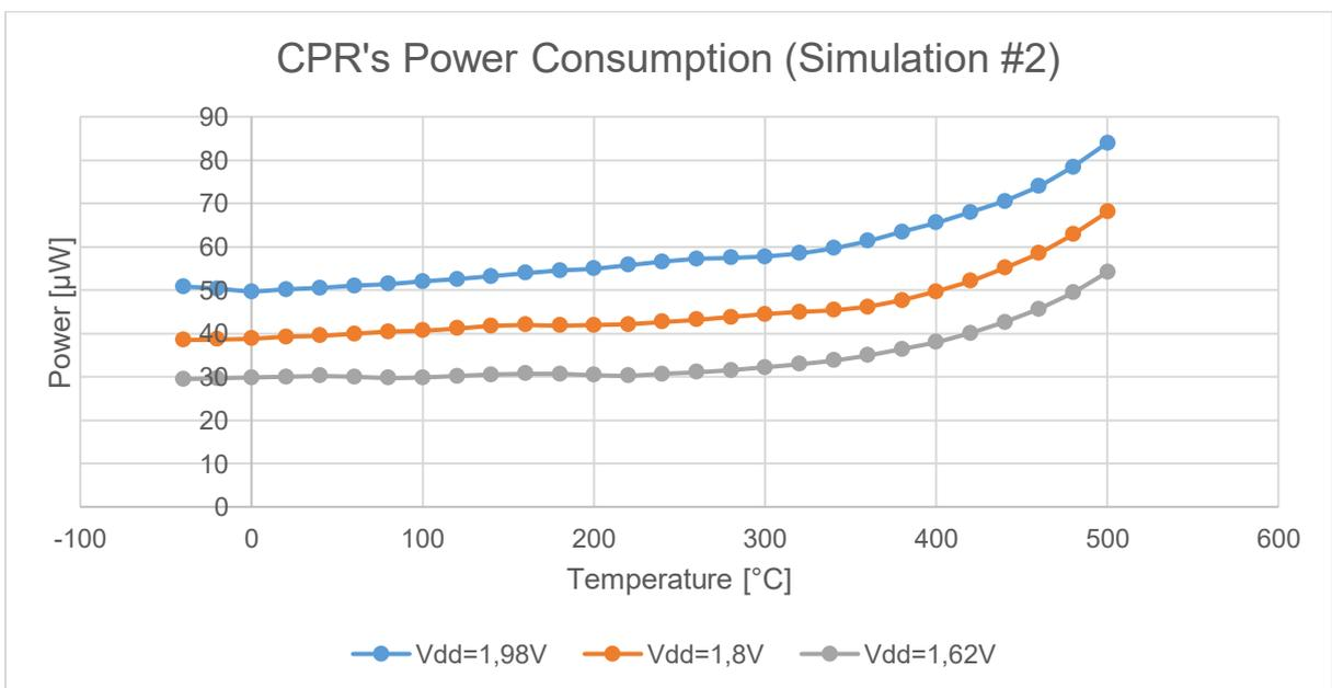
Figure 44: CPR's consumed power vs temperature (Simulation #2)
