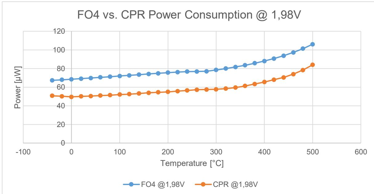
Figure 53: FO4 vs. CPR power consumption as a function of temperature driven at 1.98V
