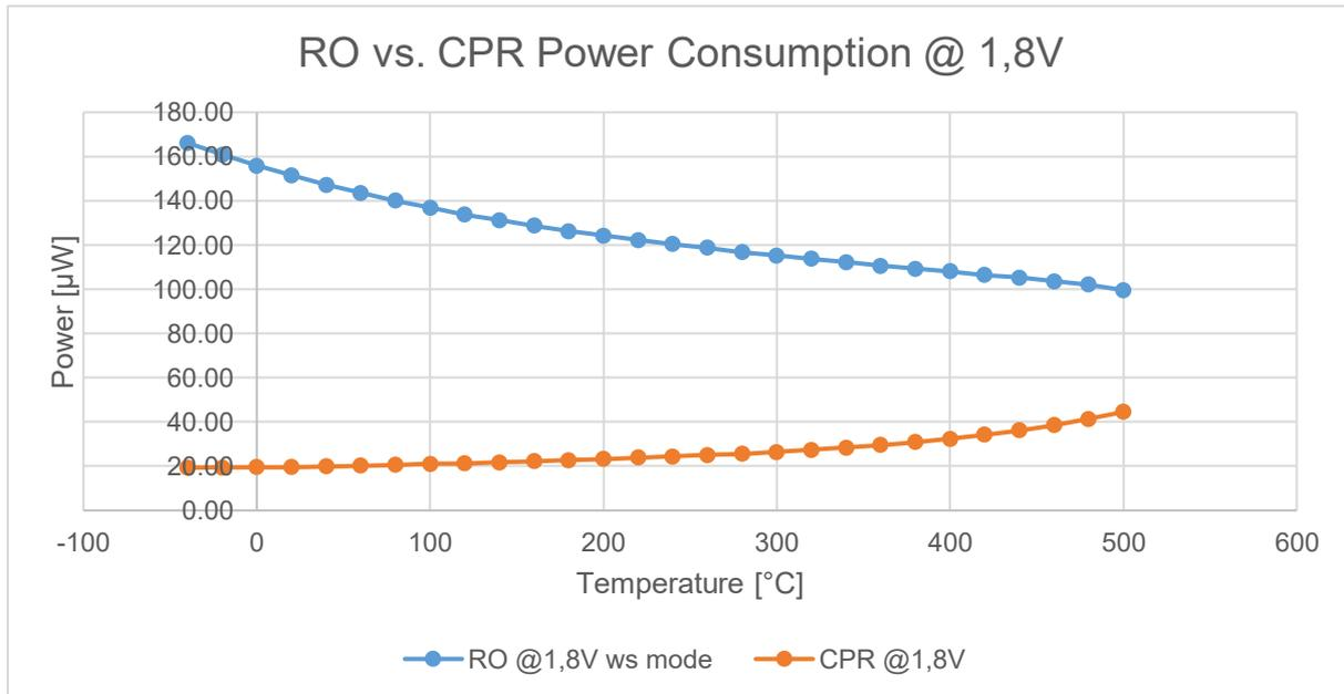
Figure 49: RO vs. CPR power consumption as a function of temperature driven at 1.8V
