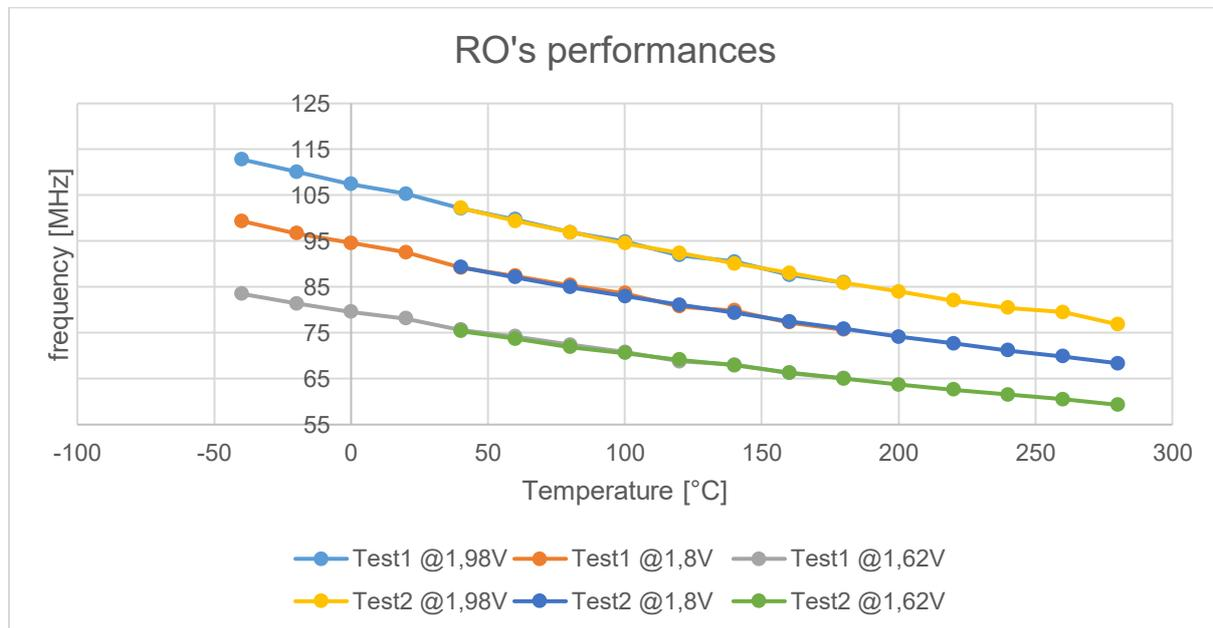
Figure 61: RO's frequency vs temperature
