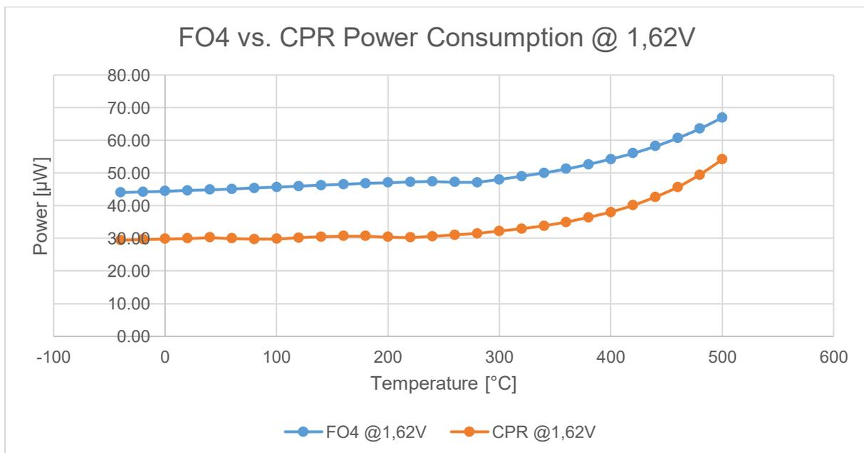
Figure 57: FO4 vs. CPR power consumption as a function of temperature driven at 1.62V
