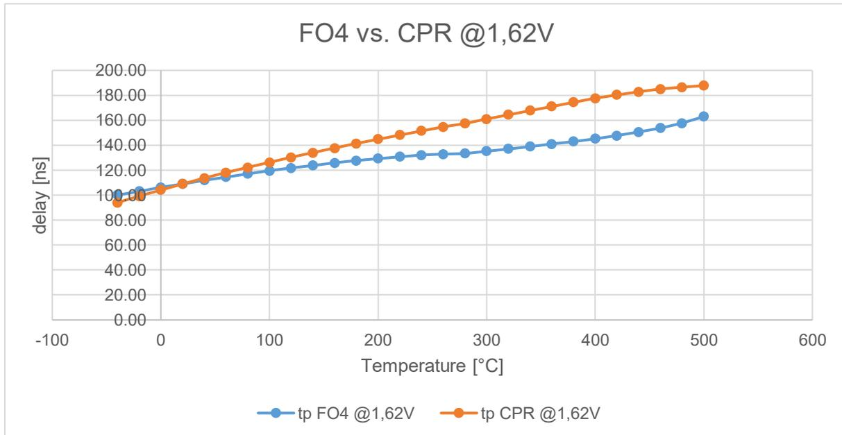
Figure 56: FO4 vs. CPR propagation time as a function of temperature driven at 1.62V
