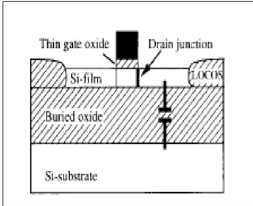
Figure 13: Junction component of the output conductance
