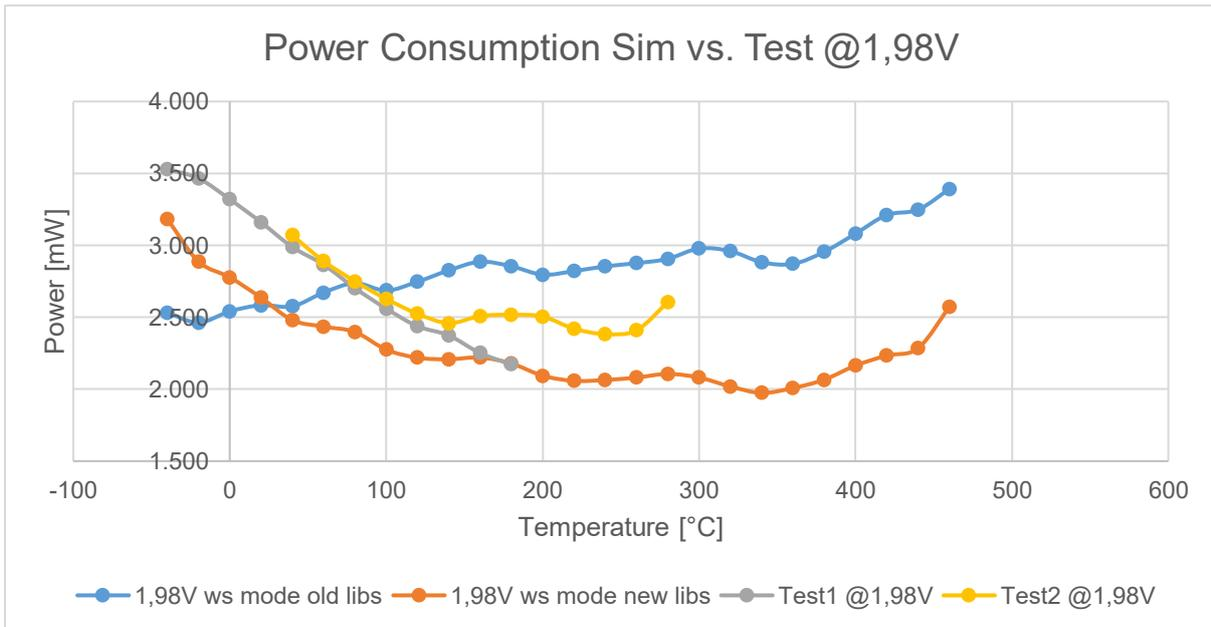
Figure 64: Simulation and Test power consumptions driven at 1.98V
