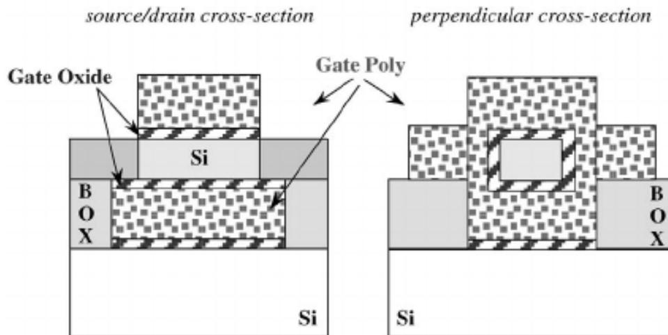
Figure 10: Gate-All-Around SOI transistor
