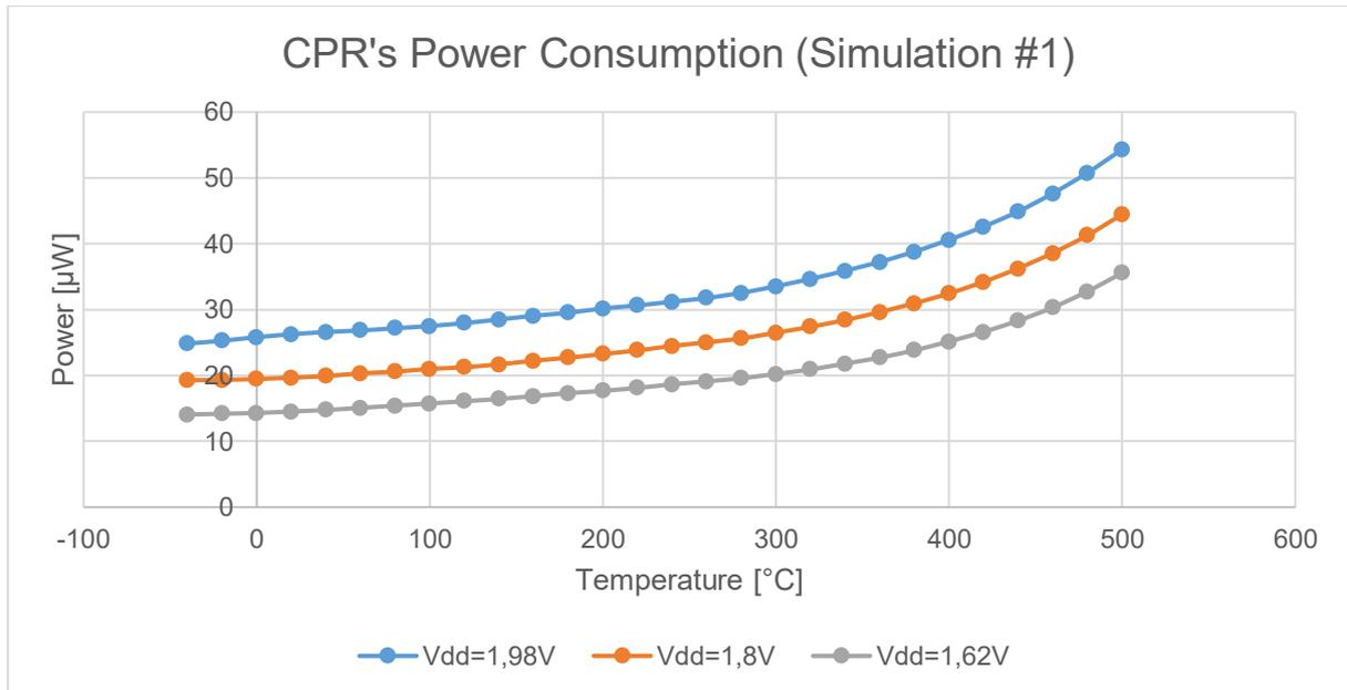
Figure 43: CPR's consumed power vs temperature (Simulation #1)
