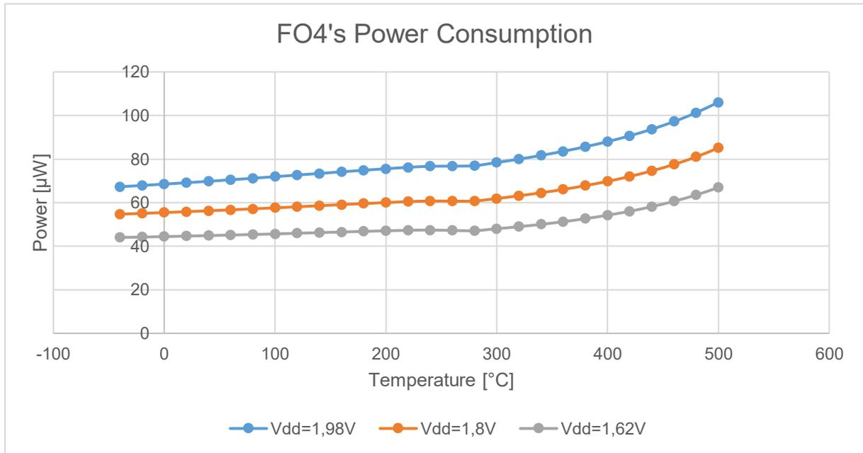
Figure 35: FO4's consumed power vs temperature
