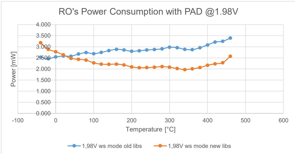
Figure 29: RO's consumed power vs temperature driven at 1.98V
