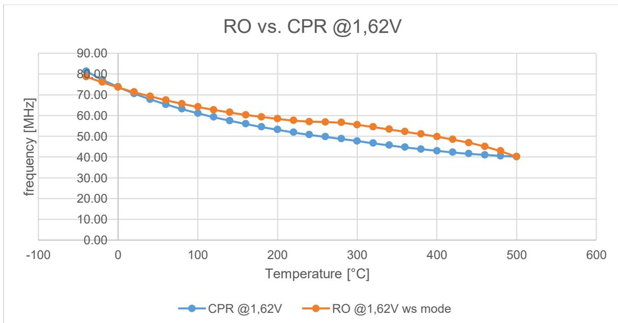
Figure 50: RO vs. CPR frequency as a function of temperature driven at 1.62V
