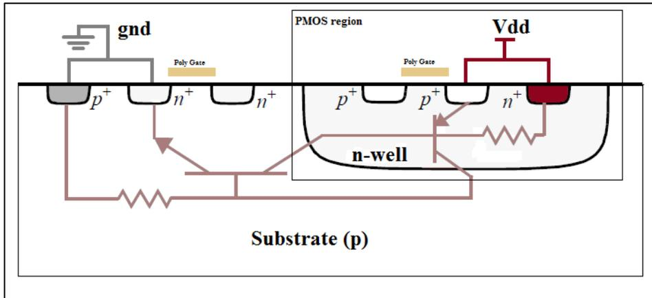
Figure 69: Thyristor created by the n-p-n-p structures
