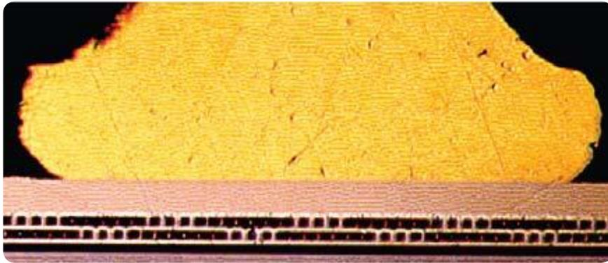
Figure 8: Monometallic bond after 3000 hours at high temperature
