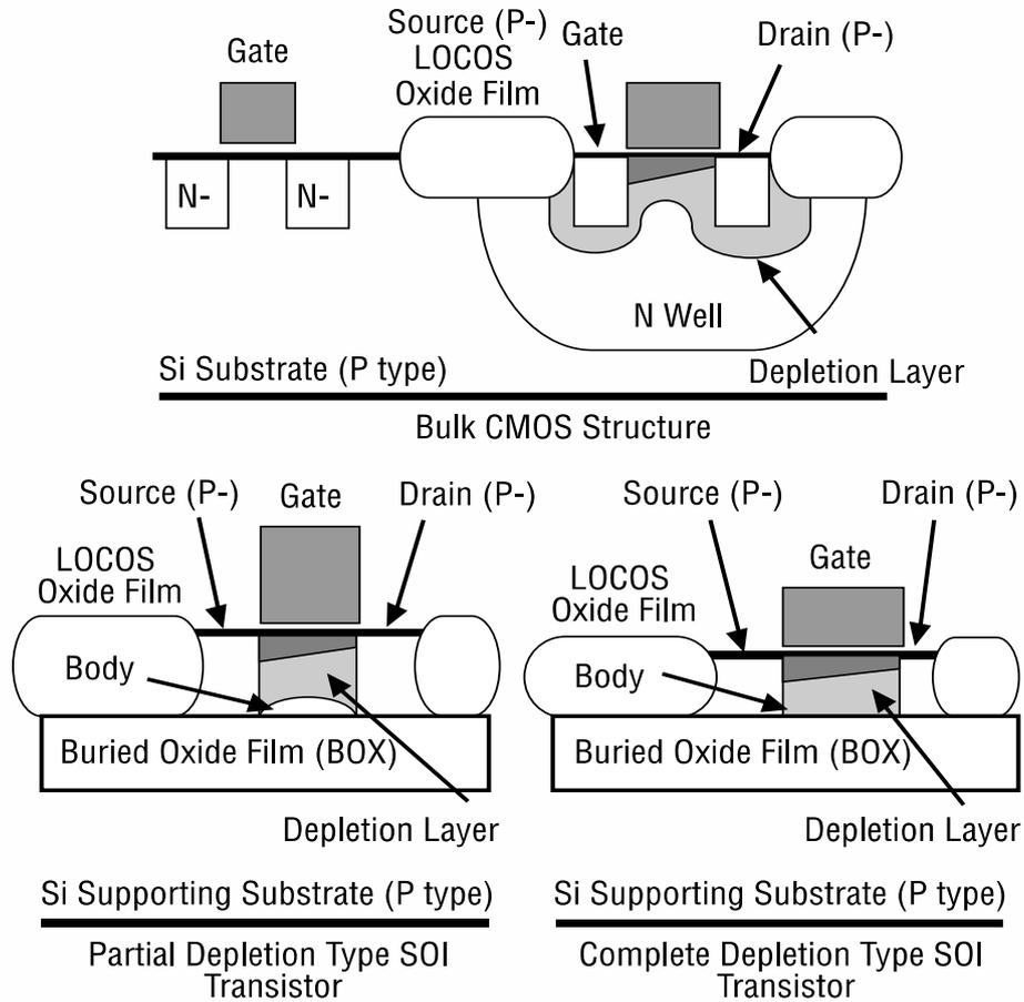
Figure 9: Bulk CMOS (top), PD SOI (bottom left) and FD SOI (bottom right)
