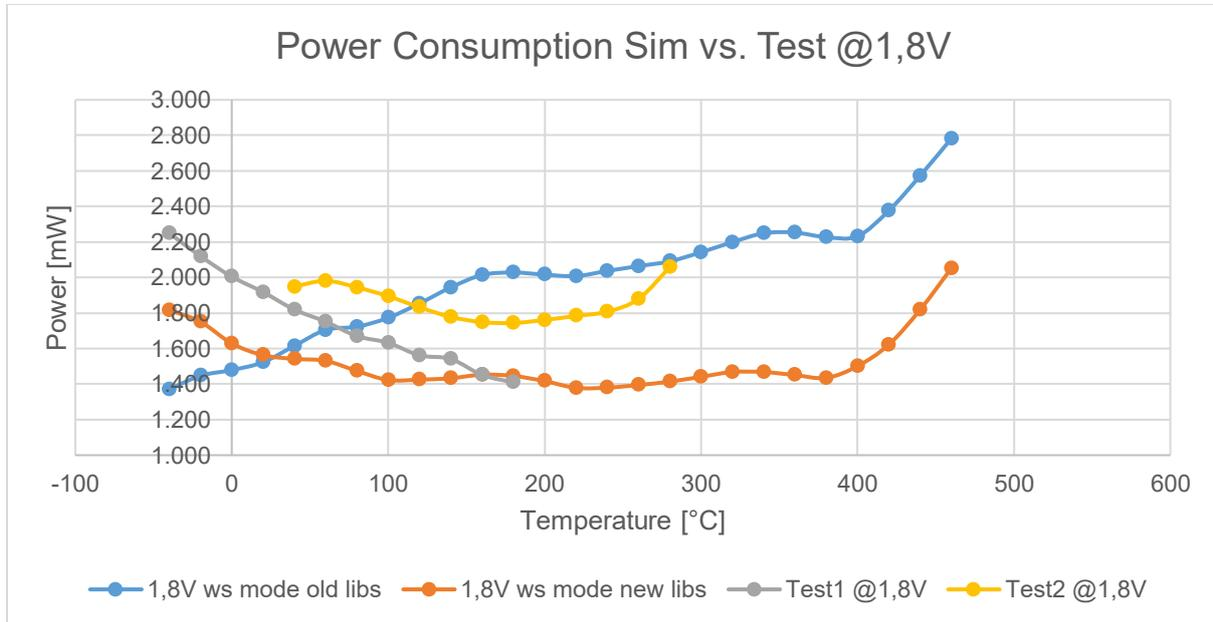
Figure 66: Simulation and Test power consumptions driven at 1.8V
