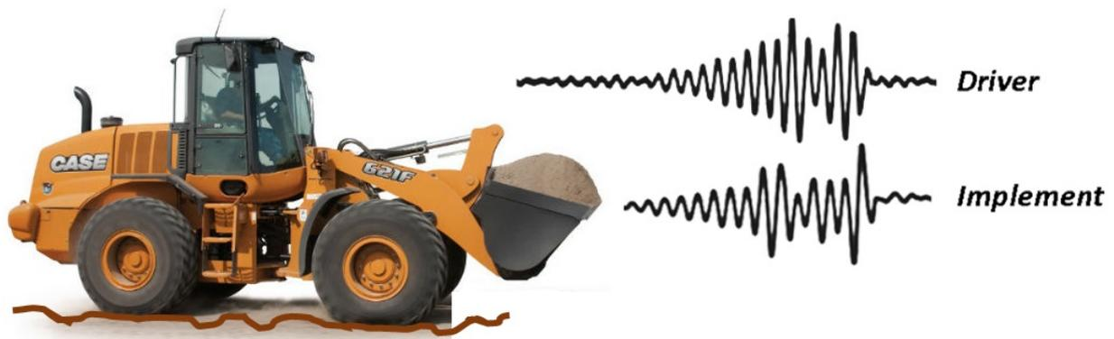
Figure 1.1: Uneven road oscillation transmission
