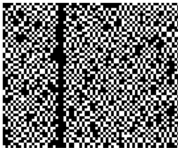
Figure 50: An SEM image processed for raw bits extraction. 1s and 0s written in the memory are turned into white and black spots. Source: Texplained
