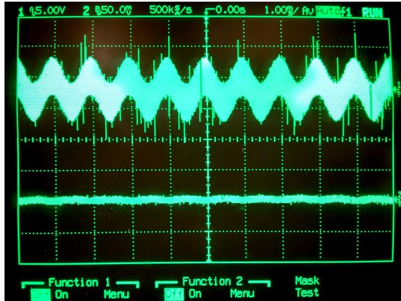
Figure 5.4: Voltage across the antenna terminals when a 1kHz signal is applied
