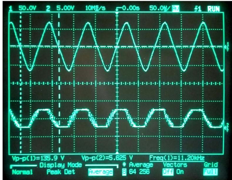
Figure 5.1: Positive and negative terminals of the transmitting antenna
