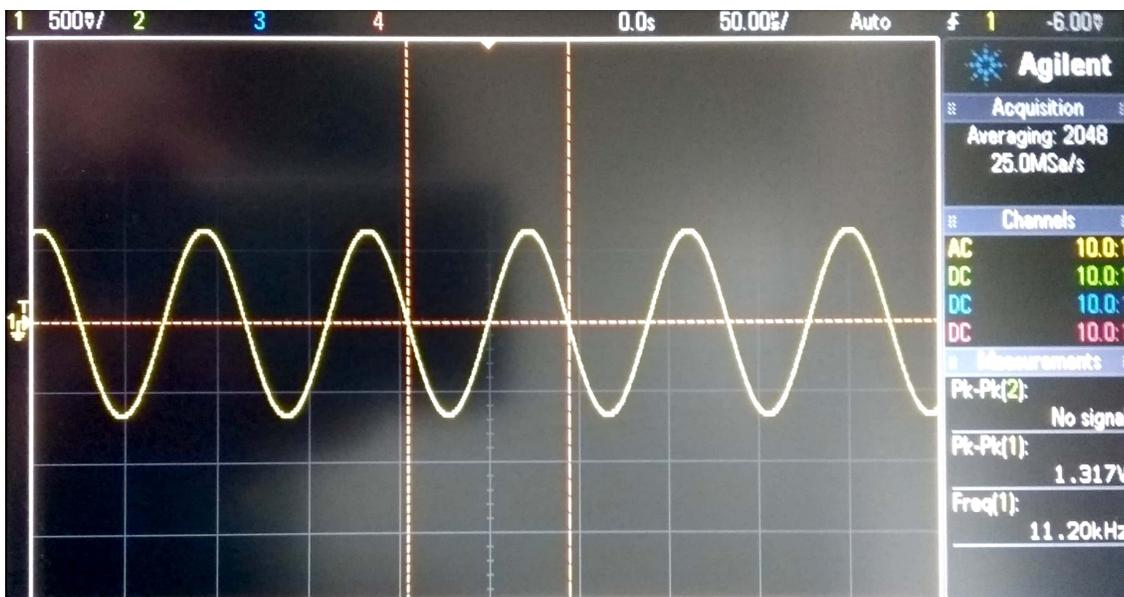
Figure 5.15: Receiver output voltage at  $d = 3.5m$
