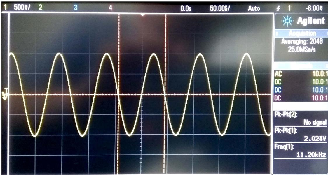
Figure 5.14: Receiver output voltage at  $d = 3m$
