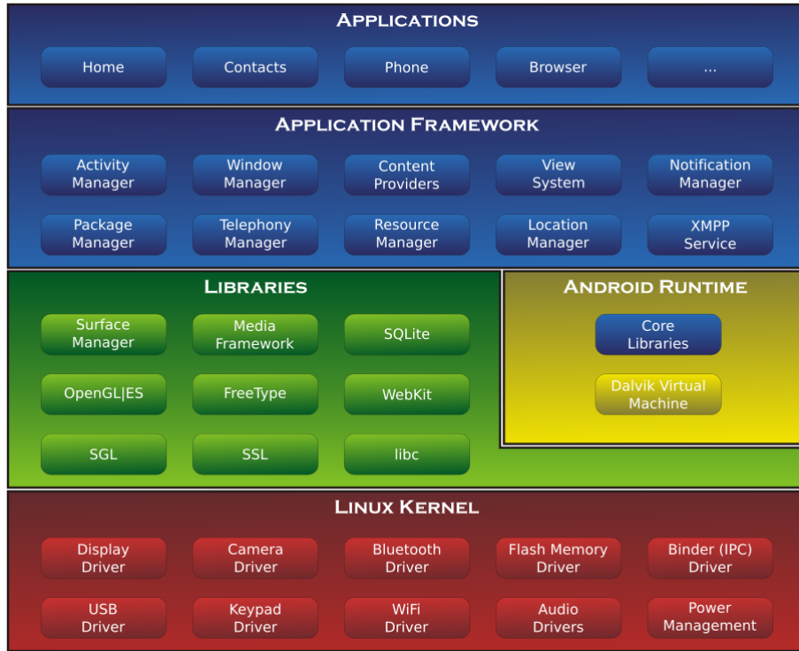
Figure 2.4: Historical Android's architecture diagram with DVM runtime environment.
