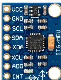
Figure 10.1: MPU-6050 Sensor [21]
