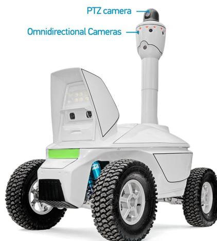
Figure 1.3: Surveillance Robot
