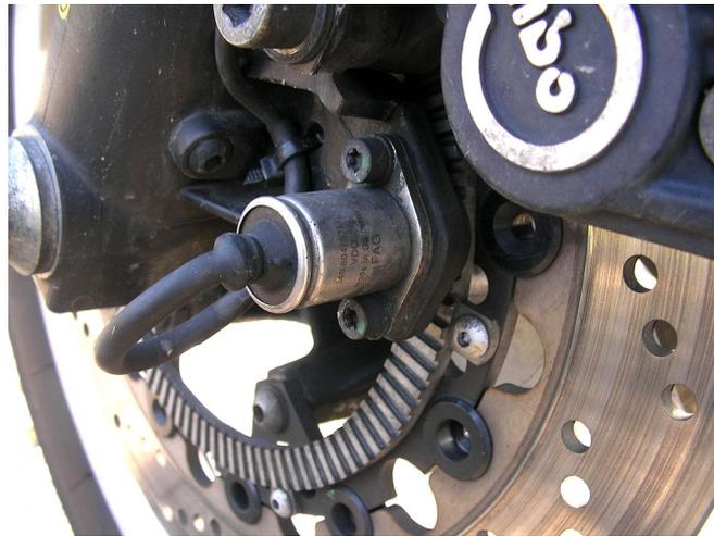
Figure 10.13: A relative encoder implemented by means of a phonic wheel, used as motor-bike ABS sensor
