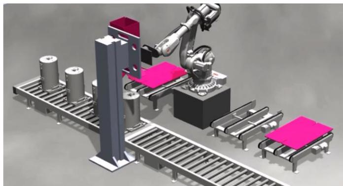
RobotStudio is a tool that can be useful at every stage of a project. It allows to pick the robotic arm that best suit the requirements of the project, and allows to recreate the environment in which it is going to be deployed. The modeling and simulation tools it contains, allow to create a realistic 3D version of the layout even at early stages: during step 2 the layout is still not completely defined, but it is however possible to verify the actual
