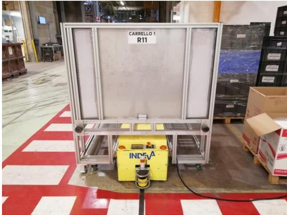
The cons of using a total of four trains is in the amount of space they occupy. The empty trains have to be parked in the picking area, in front of the aforementioned rails, while the loaded trains wait stationary until the radio signal in another parking area: for the first line this area is outside the picking area, just at the beginning of the final line, for the second line the train waits just in front its empty counterpart.
