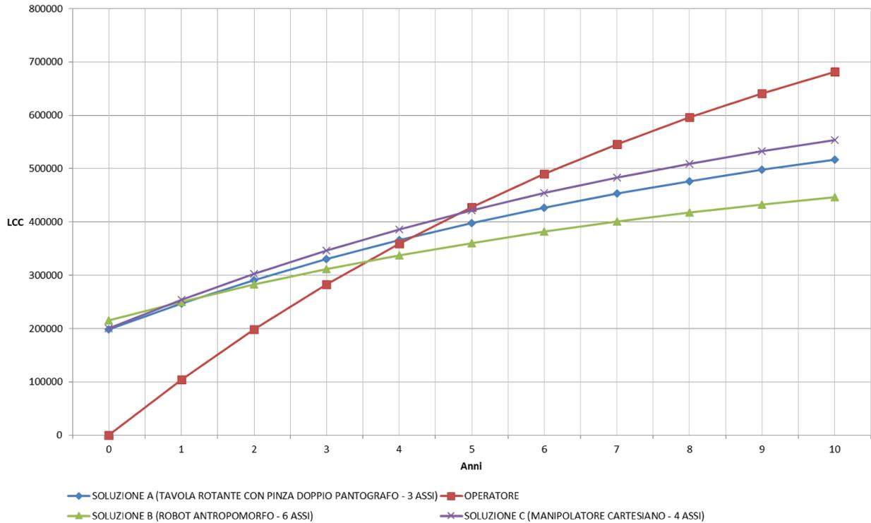
The redline shows the current situation, i.e. the labor cost of the operator over the 10 years period. The adoption of an automation is clearly advantageous for the plant.
