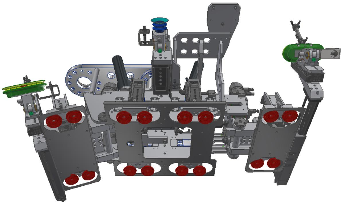
The central section of the tool is the only one that is required to hold the whole weight of the carton at a certain point during the cycle. During pick up, two faces are facing upwards: one is pulled by the central section, while the other is held by one of the lateral sections.
