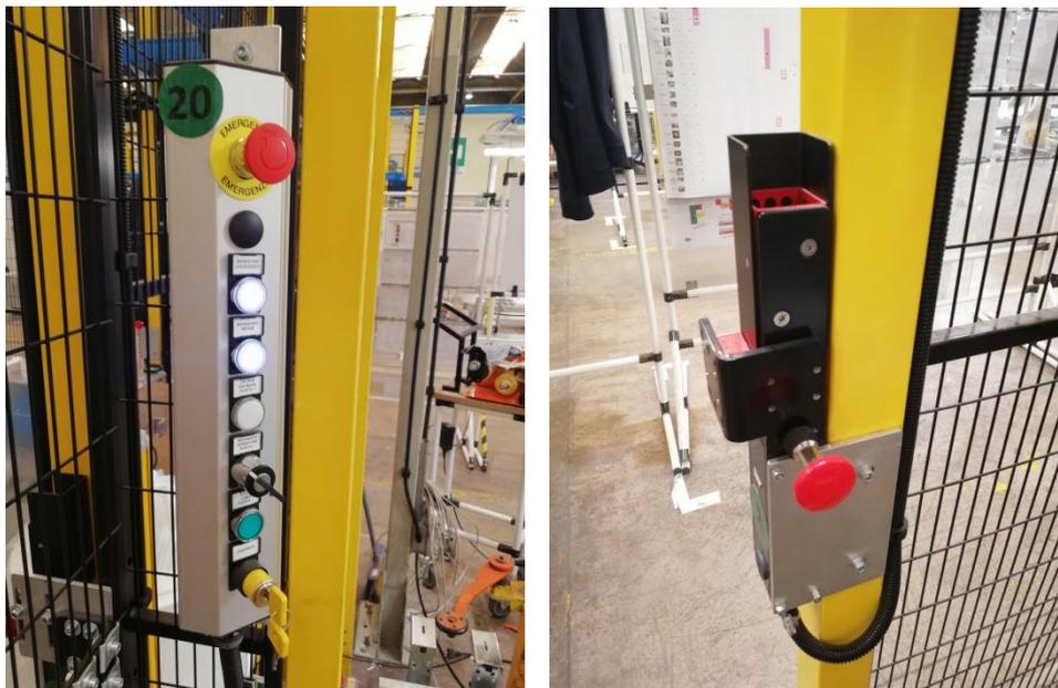
Additional emergency stop “mushroom” buttons are located outside of each door, on the main panel, and inside the barriers so that in any case in which a person is at a risk of being harmed the automation can be instantaneously halted and blocked completely.
