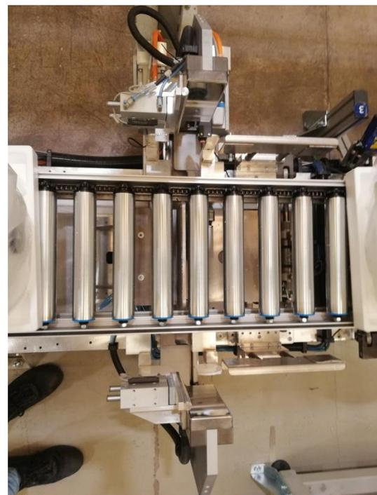
The first tests demonstrated that some inaccuracies in the process were still present as the final orientation was not perfectly oriented. Another solution proved functional and reliable, giving no further issues during the project: the clamping device has been substitute with two independently actuated jaws, controlled by the analog reading of an analog sensor that verifies the exact position at which the jaws have to be at the end of the operation.
