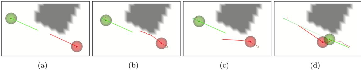
Figure 5.14: Test 5: 2 drones, both moving one toward the other, in presence of a fixed obstacle
