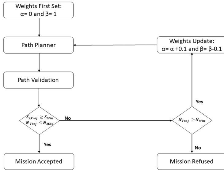
Figure 3.16: Weights assignment procedure
