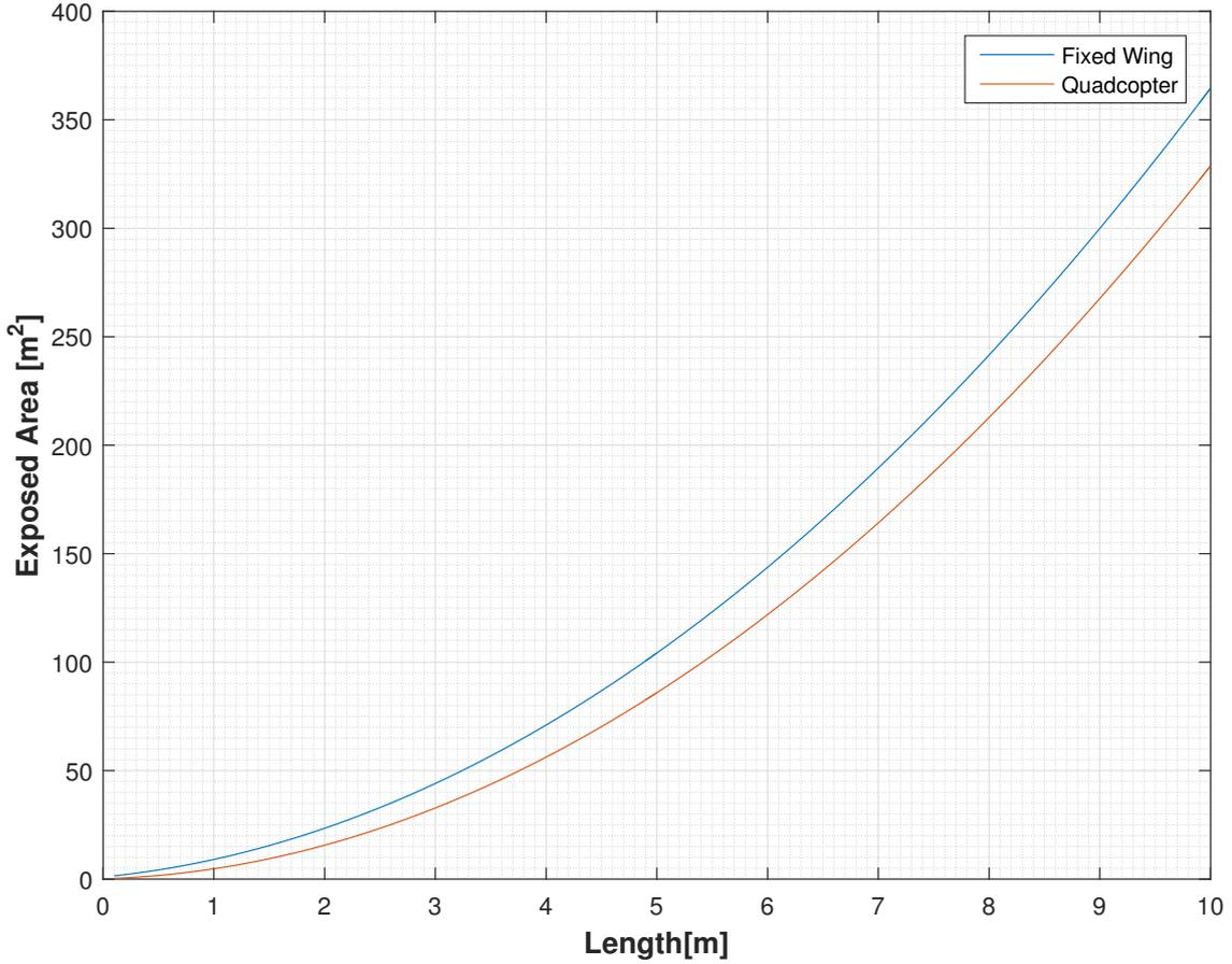
Figure 3.9: Evolution of impact area  $A_{exp}$  in function of drone's length
