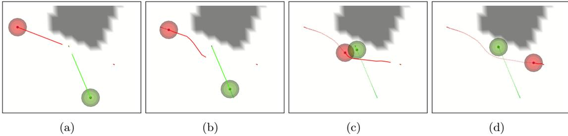
Figure 5.15: Test 6: 2 drones, both moving, crossing their path, in presence of a fixed obstacle
