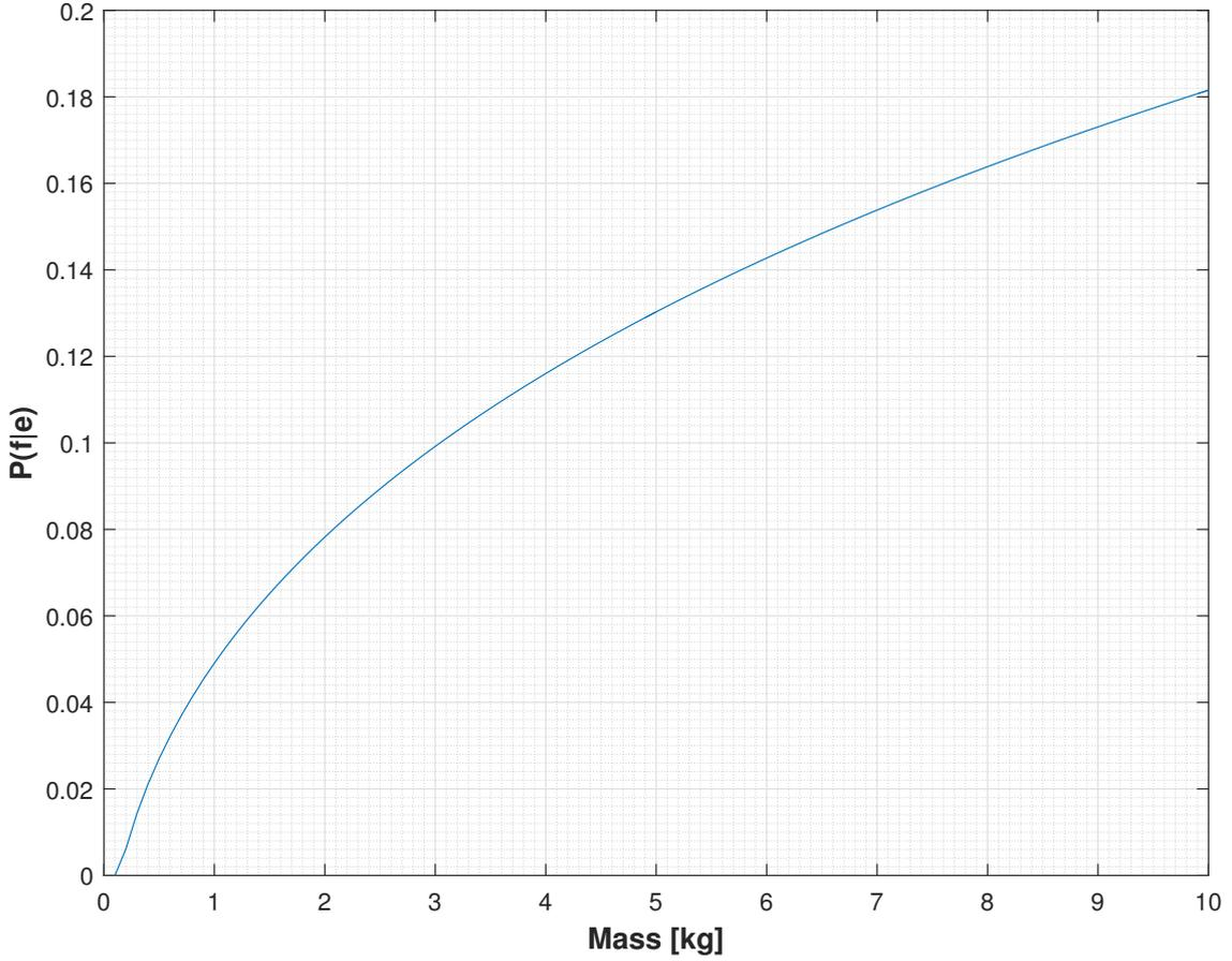
Figure 3.8: Evolution of P(fatality | exposure) in function of Mass
