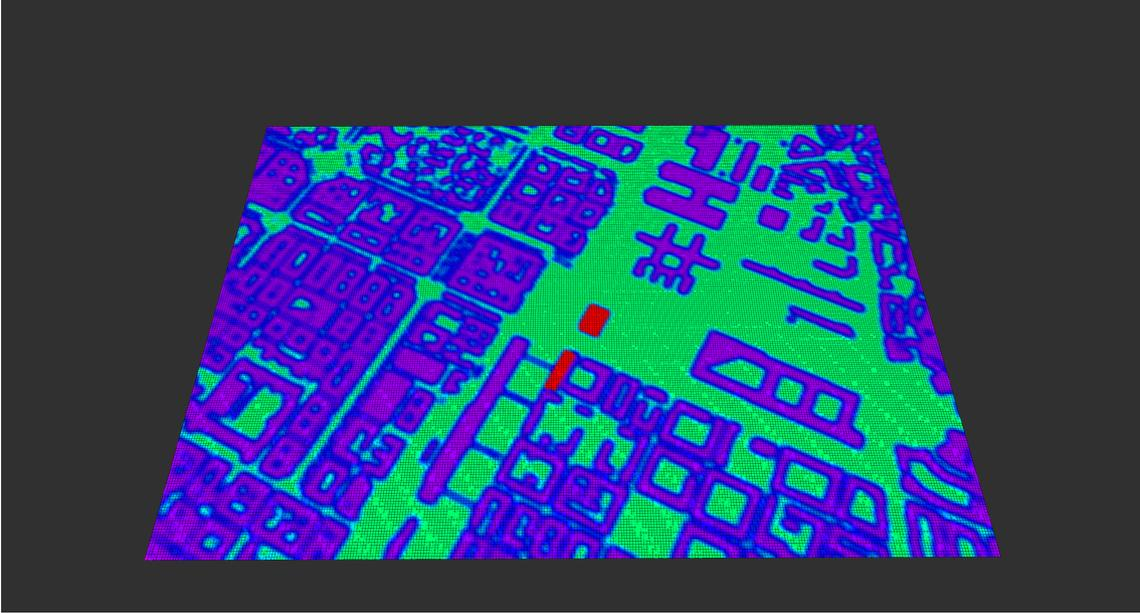
Figure 3.3: Example of Risk Map. Every area of the map has its own colour and height coherent with the risk value calculated. Red squares are no-fly zone
