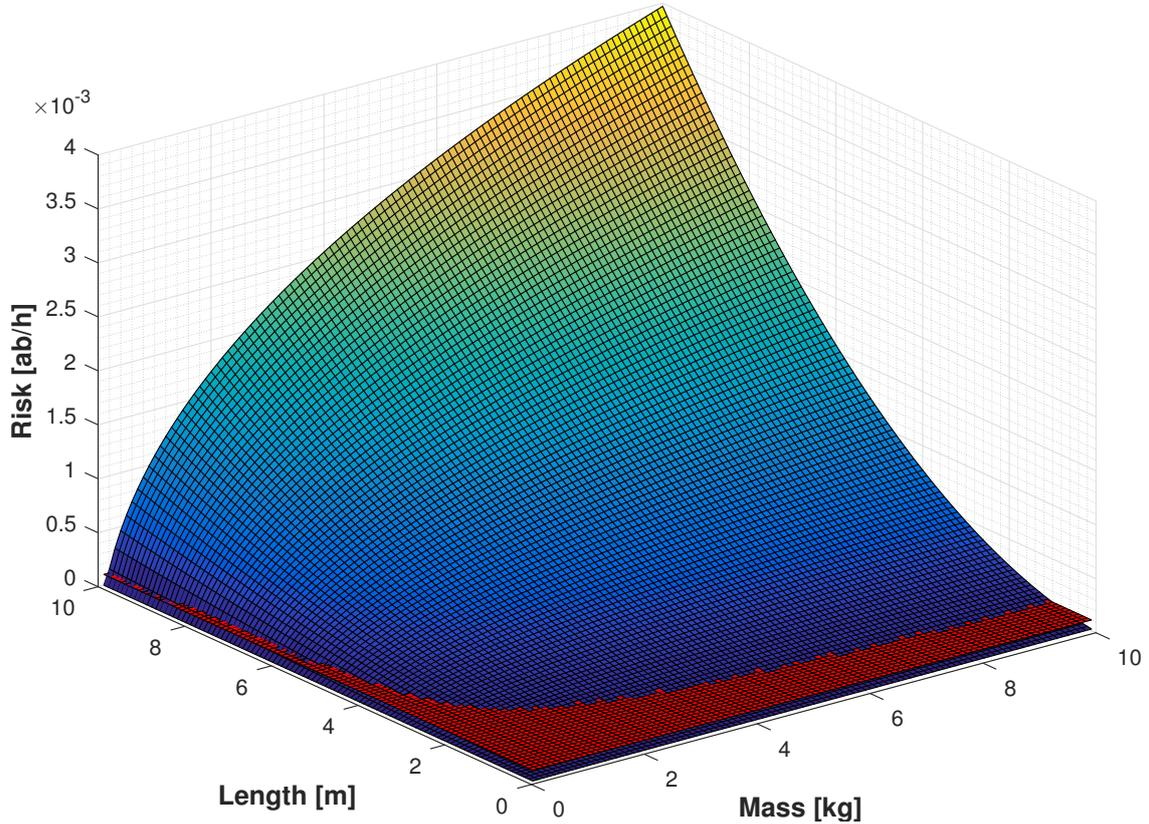
Figure 3.10: Evolution of Risk  $f_{F,i}$  in function of quacopter drone's length and mass
