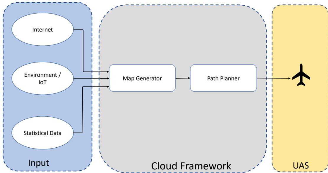
Figure 3.11: Open chain cloud framework
