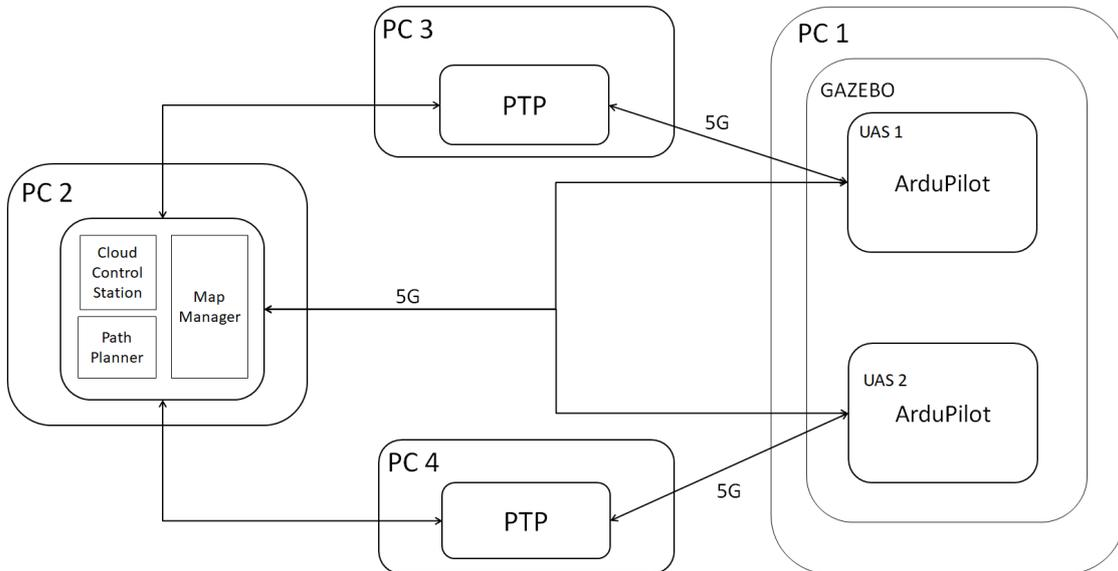
Figure 5.1: Architecture of the distributed simulation environment
