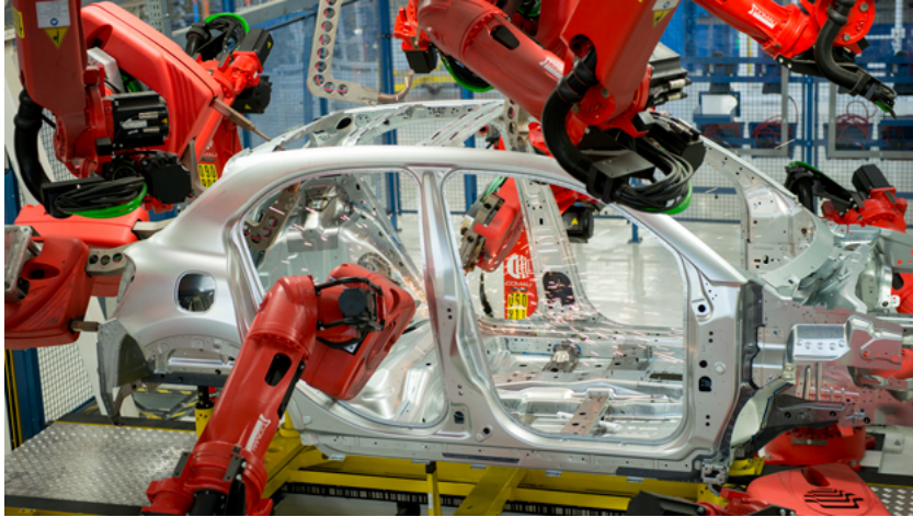
Figure 2.7: Assembling of the body metal components
