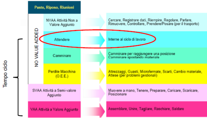
Figure 2.16: The figure shows the composition of a Time Cycle for an operator.
