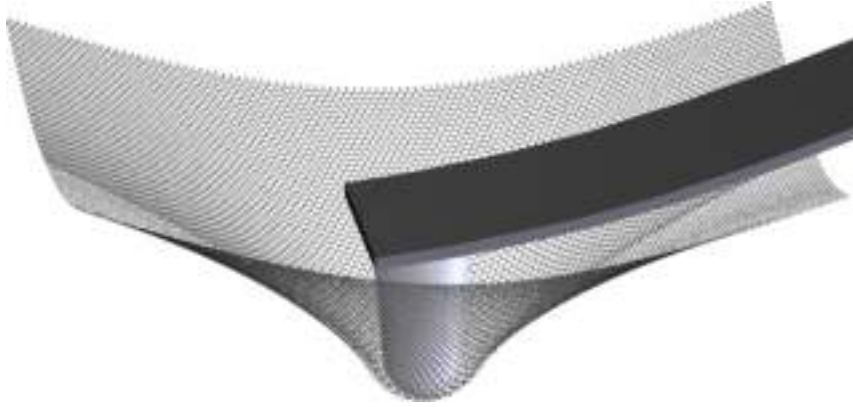
Figure 1.4: AFM tip over graphene membrane [31]
