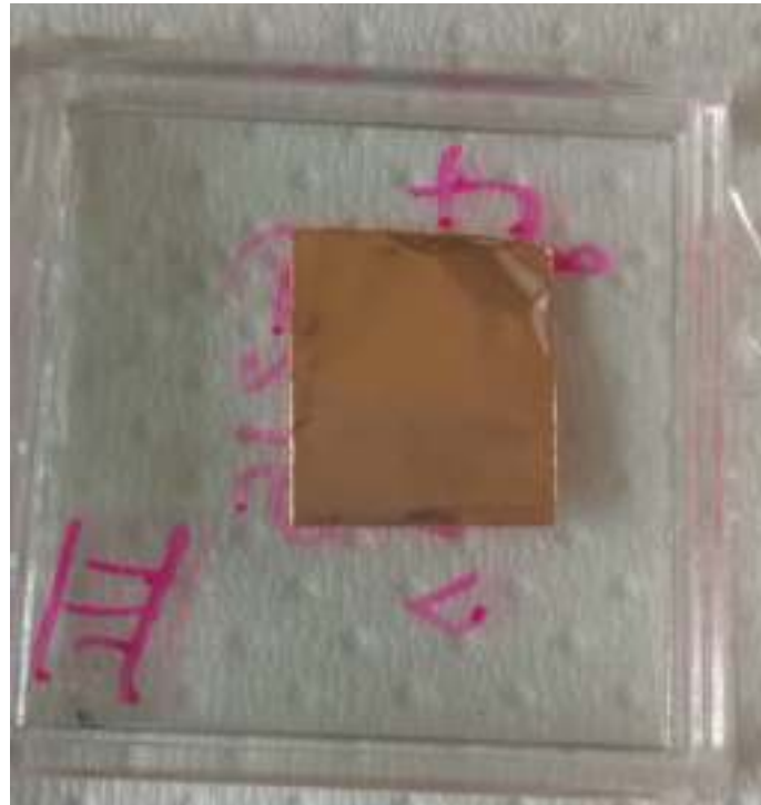
Figure 3.7: Graphene deposited over Copper via Chemical vapor deposition
