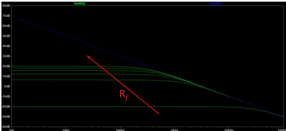
FIGURE 3.28: Transfer function of a finite gain amplifier in green for various values of  $R_f$ . Transfer function of an infinite gain amplifier in blue.
