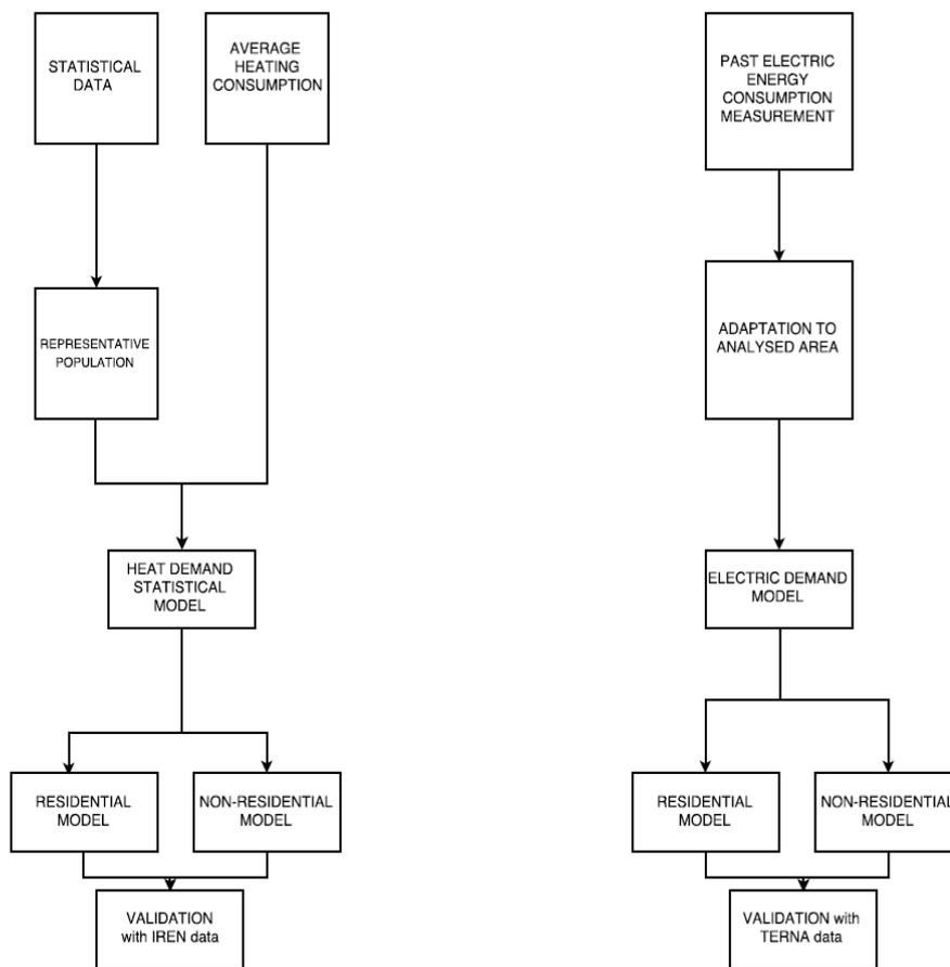
Figure 2 - Model approach for thermal energy demand (left side) and electric energy demand (right side)
