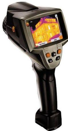
Figura 3-27. Termocamera a infrarossi (8-14  $\mu\text{m}$ ).
