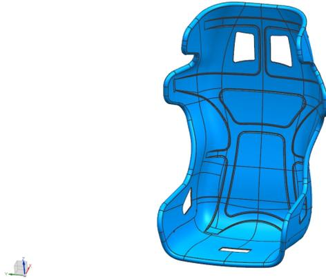
**Figure 5.2:** Shell CAD design
