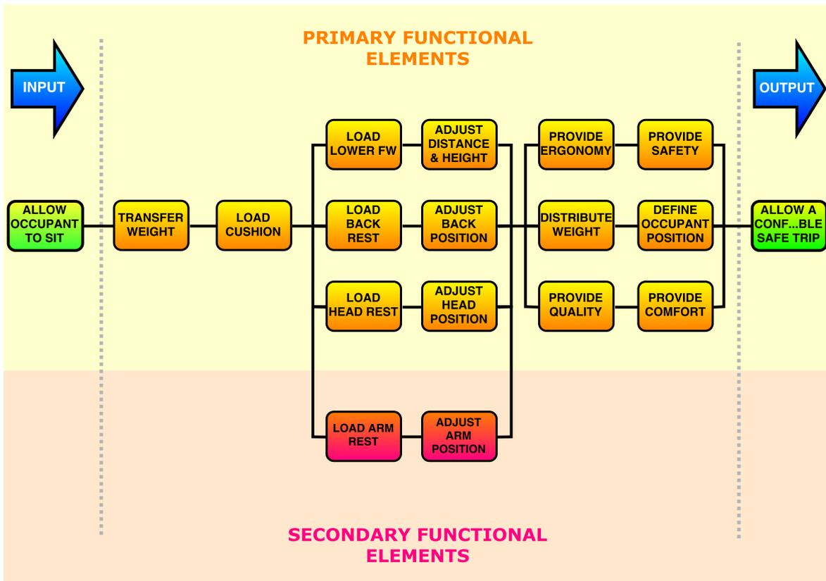
**Figure 4.8:** FAST diagram
