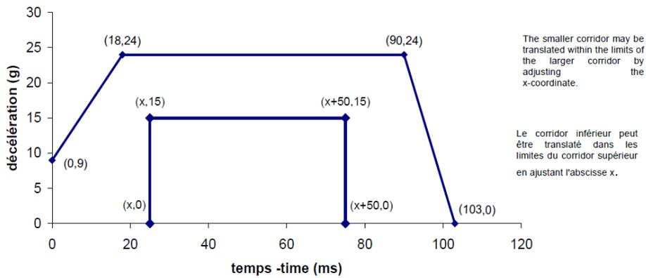
Figure 5.8: Side impact deceleration corridor - 15g
