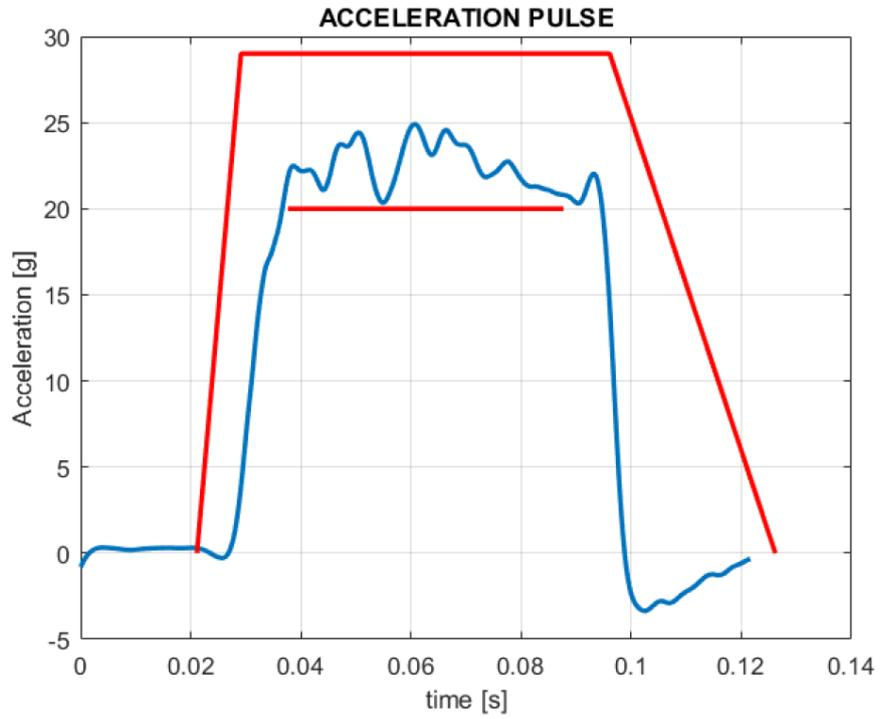
Figure 5.13: First rearward impact test result
