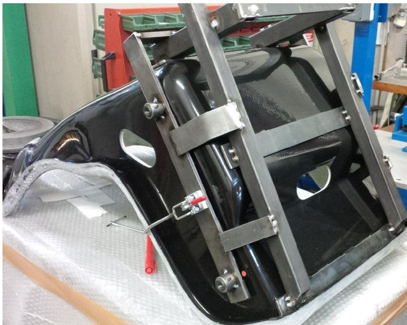
Figure 5.11: Mounting template
