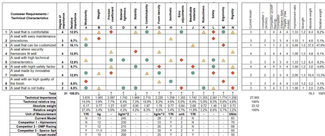
Figure 4.11: QFD matrix with modularity as technical solution
