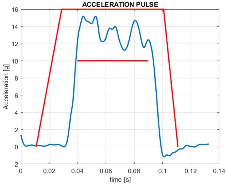
**Figure 5.15:** Second rearward impact test result
