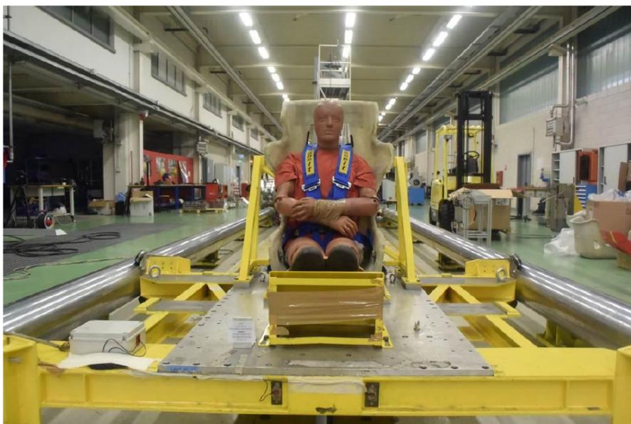
**Figure 5.12:** Dummy positioning during test
