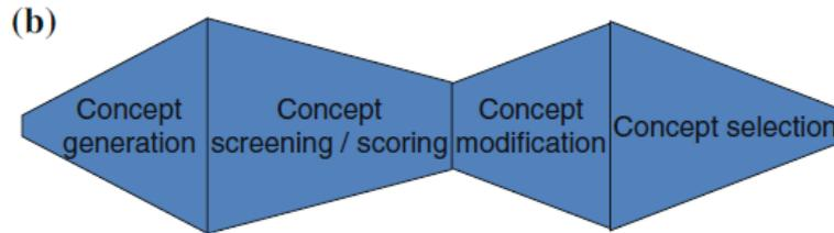
**Figure 4.5:** Conceptual design process
