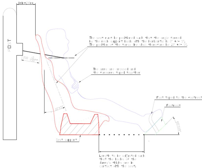
**Figure 5.6:** Dummy standard position
