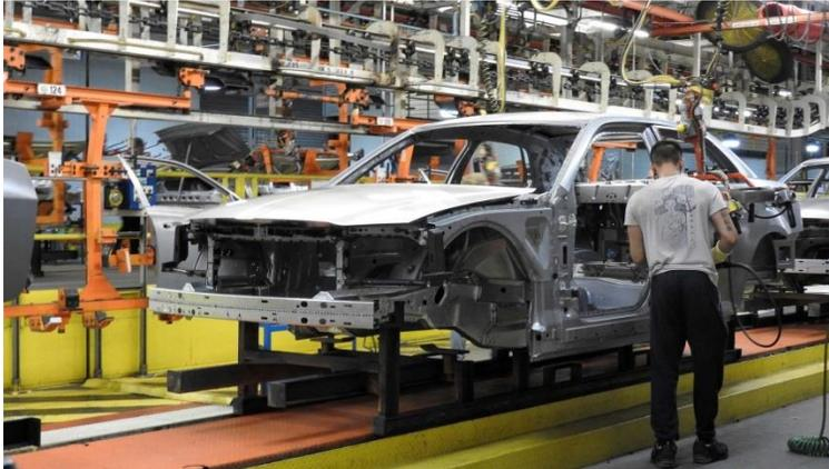
*Figure 9: example of on line repair on a car that could not be checked during the Reaction Process as it was in an elevated position.*
