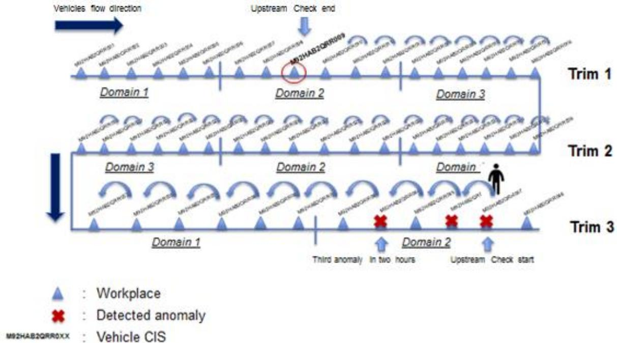
Figure 8: graphic display of Upstream Check; the second workplace of Domain 2 (Trim 3) detects three anomalies in few minutes; note that the Team Leader who must perform the control does not start from the workstation that detected the defect, but from the first of the three cars presenting the anomaly; during the check, the Team Leader must not only verify that all cars are in conformity but also repair them in the event of anomaly found.
