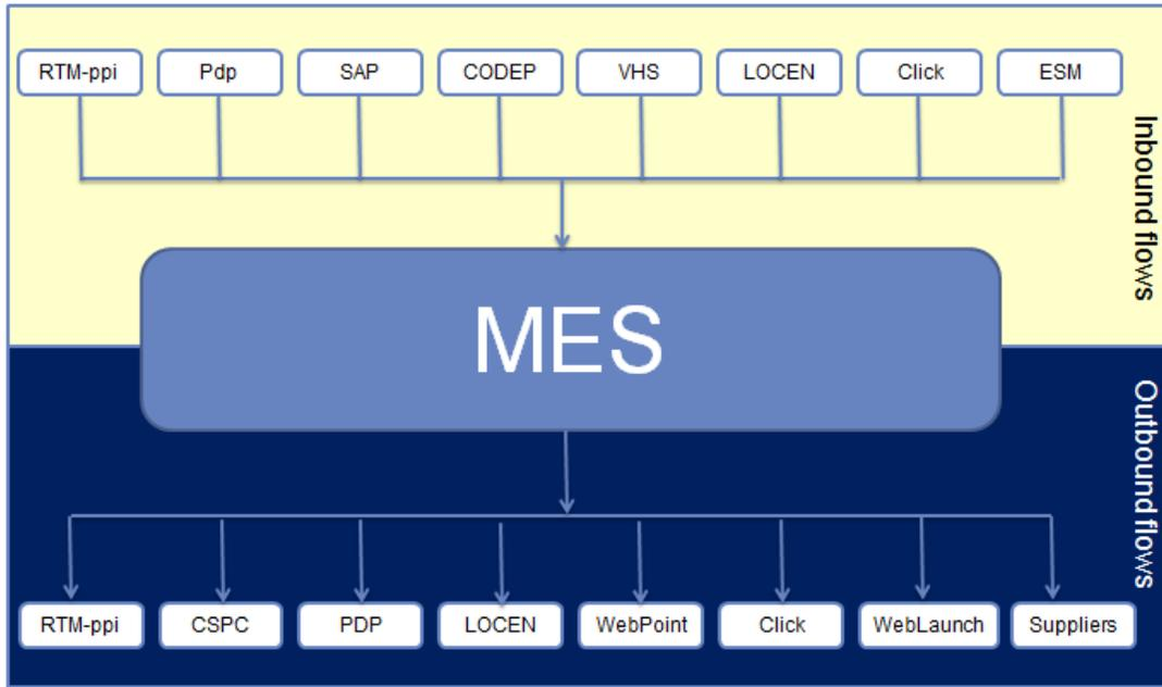
Figure 6: the scheme of the Mirafiori's digital system with underlined connections with the plant subsystems in input and output.
