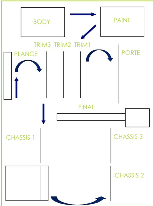
Figure 4: the traditional Assembly Shop layout of an automotive “Premium” plant; after the Body Shop and the Paint Shop, the product flows in three lines of Trim and in three lines of Chassis before arriving at the Final where all the controls are performed. The workings of the doors and the planks occur in parallel with the Trim.
