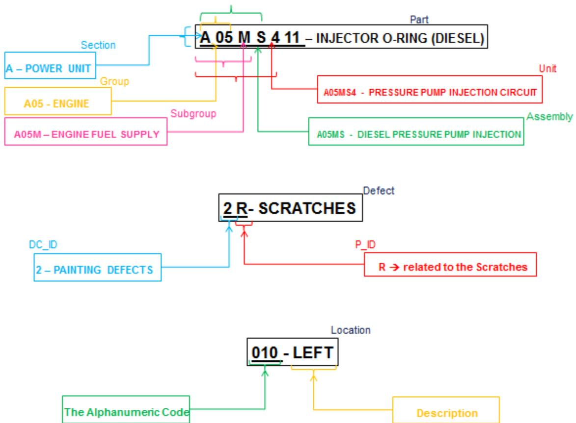
Figure 22: component, defect mode, location digits code details (from the top to the bottom).
