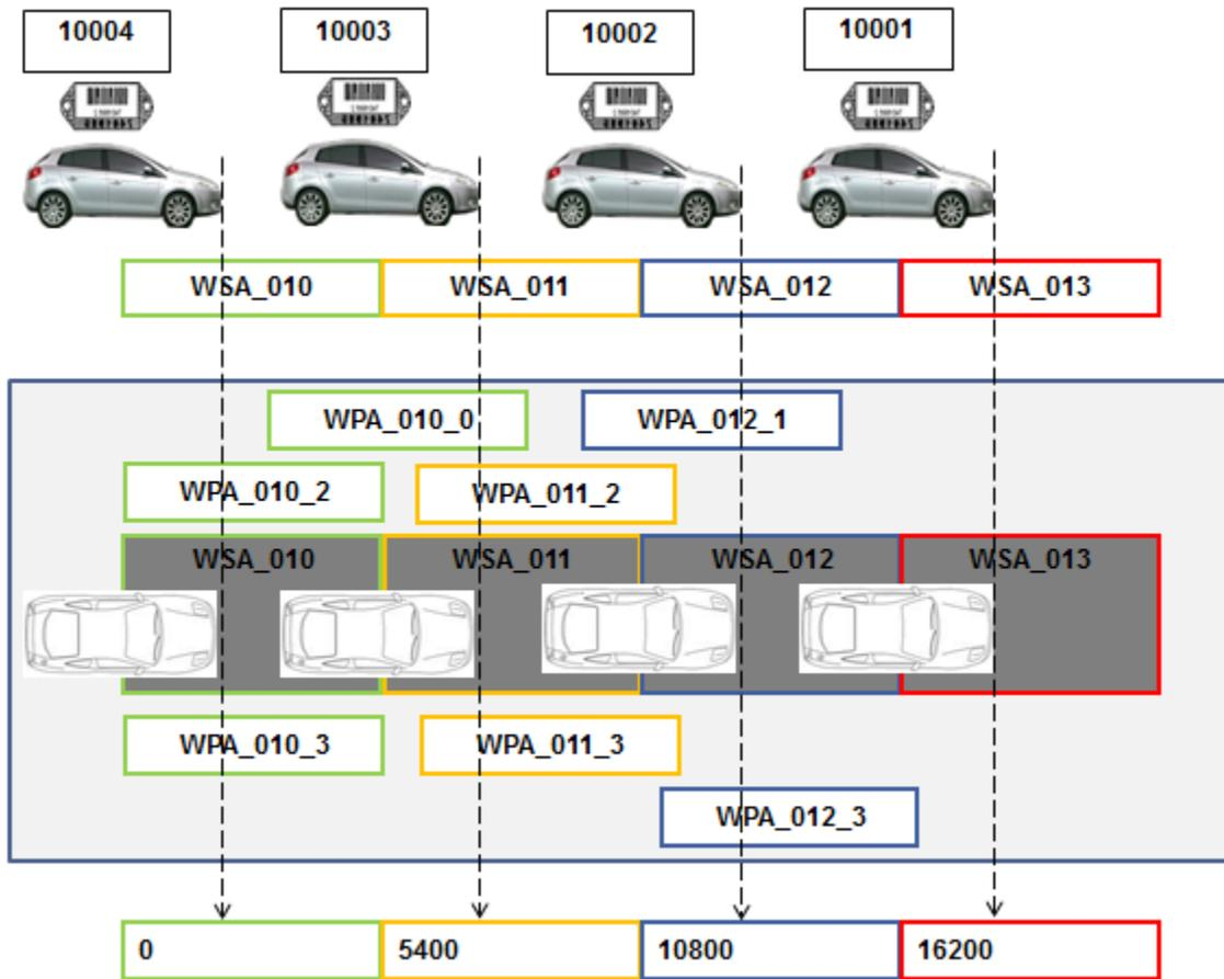
Figure 7: framework of the “Premium” plant line flow with an example of the different workstations (WSA) and workplaces (WPA) locations.
