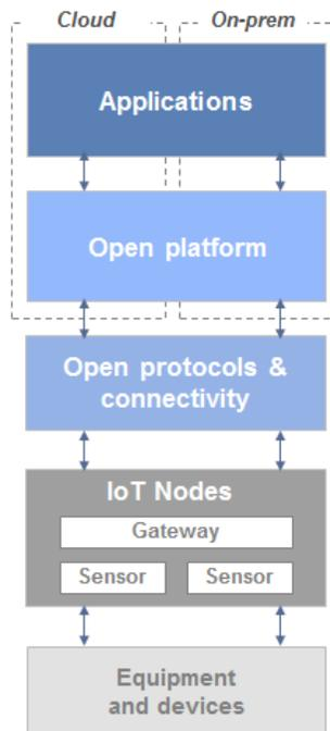
Figure 44: apps support use cases to reduce losses and generate profit; the open platform collects data from the devices; the connectivity standardizes the communication; the network infrastructure supports a large amount of data management; gateway sends data from sensors to open platform.
