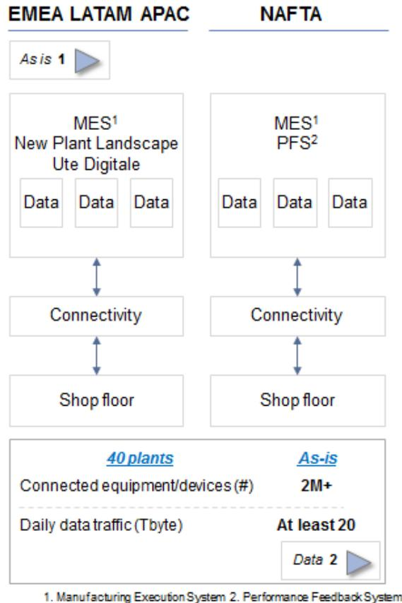
Figure 43: graphical framework of the As Is situation where it is clarified that the systems which collect data need a powerful connectivity tool to be linked to the Shops of the three Units.
